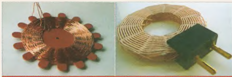
The spiderweb coil at left is wound through the radial fingers of the flat former to reduce the inter-turn capacitances. At right, the basketweave coil , another method of reducing the capacitances between turns and layers, is arranged to be self-supporting (Wikimedia). These two examples also represent pancake-style coils. In the early days of radio, such coils also served as antennas in broadcast receivers, from crystal sets to superhets.
