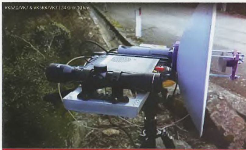
Photo 5. VK5KK/VK7 system at Mt Wellington (134 GHz configured).
