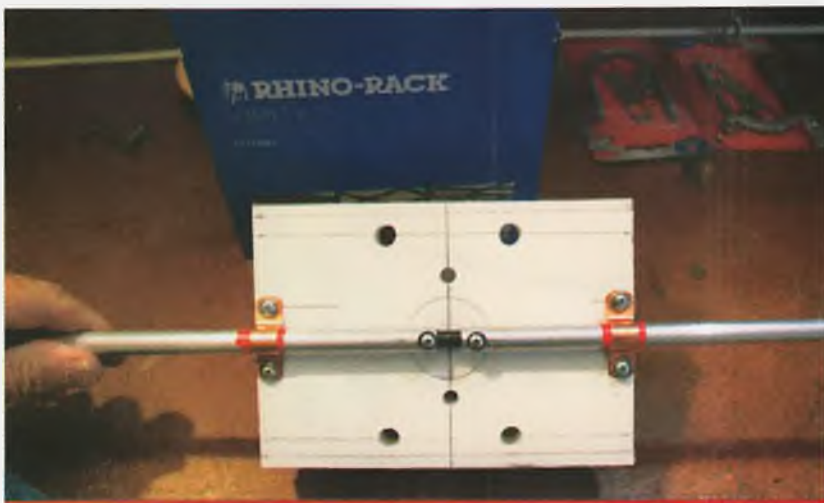
Figure 13. Driven element mounting details.
