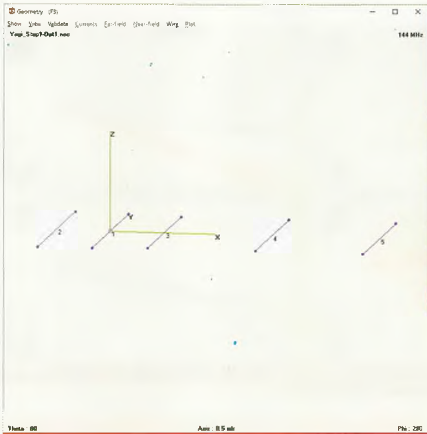
Figure 4-2. 5-element 2m Yagi model – Starting Parameters – Geometry Screen.
