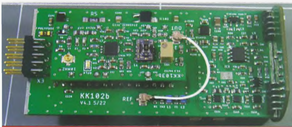
Photo 2. The 40–100 MHz PLL VCTCXO PCB installed on VK5KK's 122 GHz PCB.
