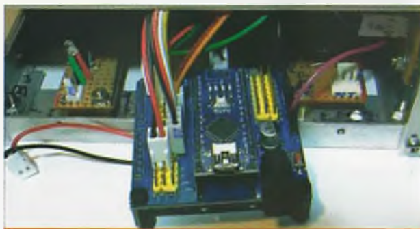
Photo 5. The Arduino Nano and Shield pulled out of the case showing the general arrangements.
