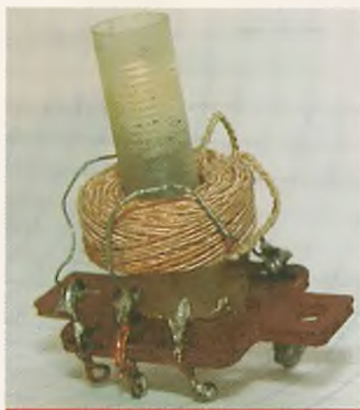
Basket-wound, or honeycomb, coil made with fine Litz wire for a receiver IF transformer (Wikipedia). The winding itself is known in the trade as a "pi, or pie" (hence, "pi-wound"). The wires are laid down in a criss-cross way, reducing the capacitances between turns and layers.
