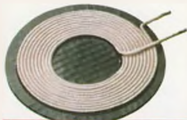
The pancake coil generally refers to a single layer helical coil (flat spiral) reminiscent of a watch spring (tdk.com). They are also wound with Litz wire. Famously, a pancake coil forms the primary of a Tesla coil transformer high voltage spark generator. Pancake coils find application where strong inter-coil coupling is required. Where a coil is wound such that its diameter greatly exceeds its length, it generally attracts the pancake coil label (Ref. 4).
