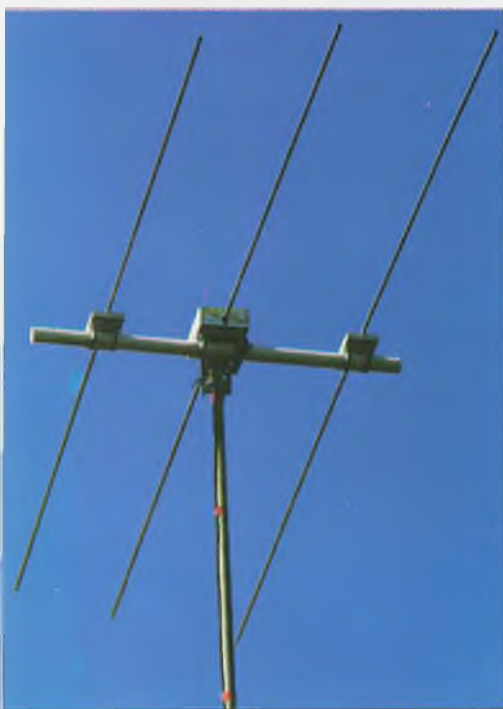
Figure 15. My 3-element Yagi antenna mounted on a mast.
