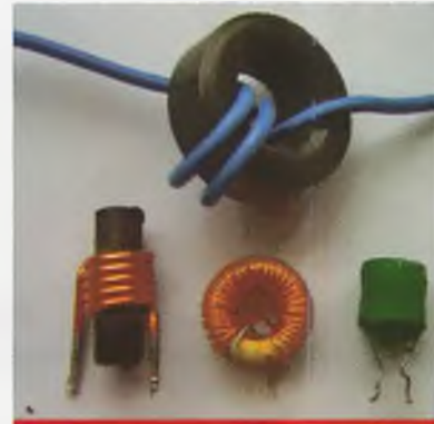
Figure 2: Various inductors that may be seen used in resonant circuits. The toroid at the top, with a few turns of heavy wire wound on it, may be used as a 'choke' to block RF current above a certain frequency.
