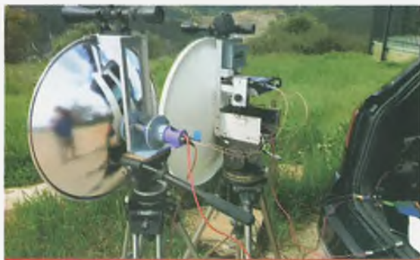
Photo 1. VK5KK's 450 & 600 mm 134 GHz systems – 31 km to VK5ZD, for a new DX record.
