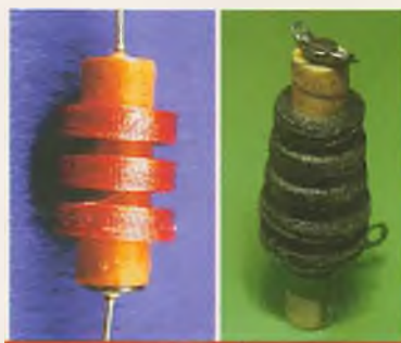
Multi-pi windings: at left is a three-pi honeycomb wound RF choke, often found in the low-power stages of transmitters, and in receivers (surplussales.com). At right is a five-pi progressive-wound RF choke, designed for the DC feed to the plate circuit in an RF power amplifier (eBay). Multi-pi arrangements enable high inductance while maintaining a lower voltage differential per winding. In the progressive-wound RFC, each pi has a different self-resonance arising from the inherent multiple parasitic capacitances. In a multi-band transmitter, the array of self-resonances can be designed to occur outside the operating frequency bands.
