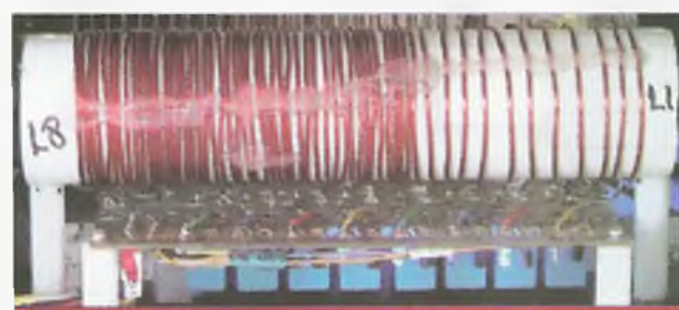
Photo 3. View of the complete inductor mounted in the case. Note the relay board mounted immediately under the inductor. This enables short, direct connections to the inductor sections.
