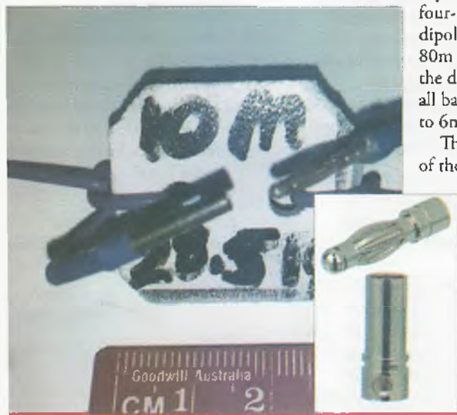
Figure 4. Linked dipole linking - revised design. Inset - the male and female connector parts come from RC suppliers.
