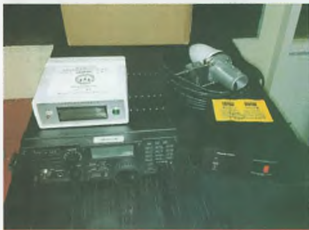
The VK6RBP beacon equipment. Note the NCDXF-built controller atop the rig and the GPS antenna at top right.
