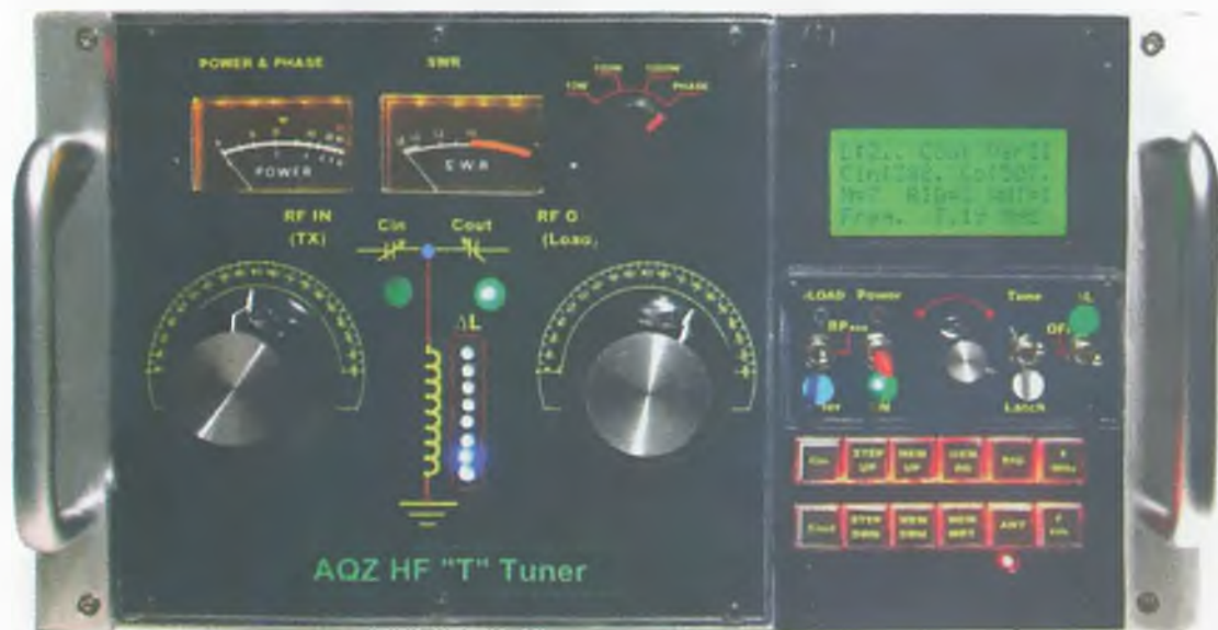
Photo 1. Antenna tuner front panel. Note the two knobs for hands-on tuning of the capacitors, the two analogue meters and the digital display.
