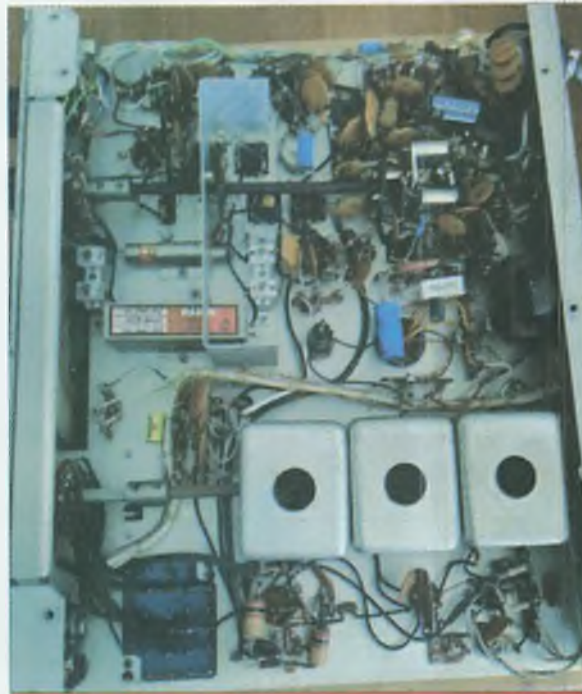
Figure 5. Below chassis view of my 75S-3. Clearly, this unit was designed and built in the days when hand wiring ruled! The three prominent aluminium cans along the bottom edge of the chassis shield sections of the band switch.
