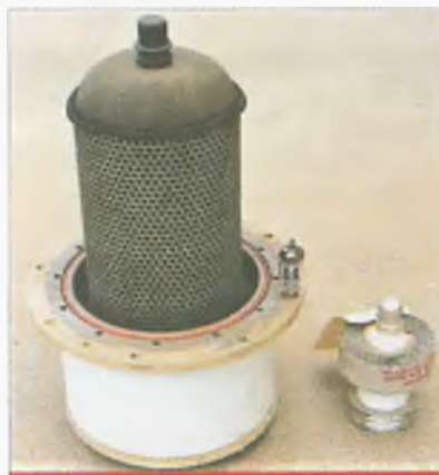
At 100 kW, size matters. At left is the STC100's 4CV100,000E output valve, with the 4CX1500A driver valve at right. A 12AX7 provides size comparison.
