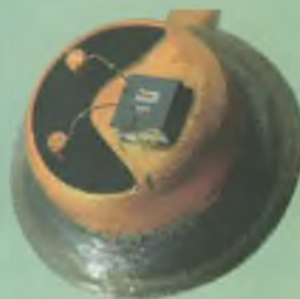
On the inside: Left – a small signal device. Right – a power device; the metal package helps carry away heat. (images: Wikimedia)
