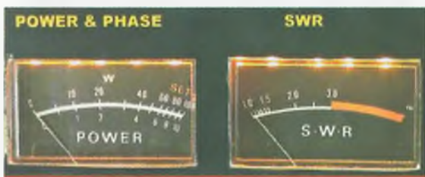
Photo 9. The front panel meters. These have been repurposed from a small commercial SWR meter unit.
