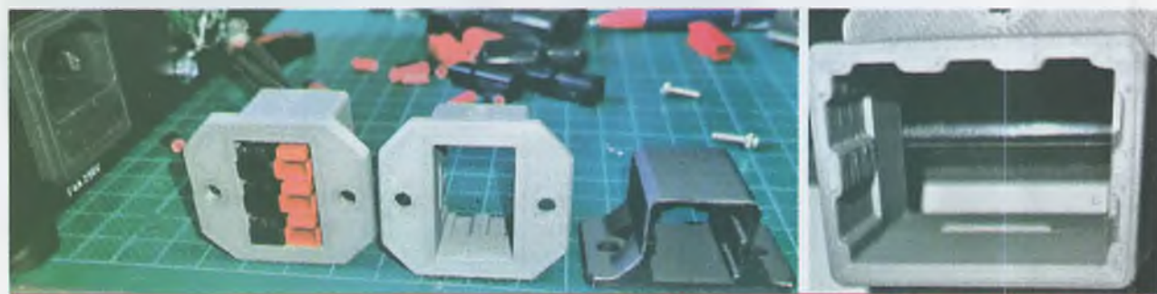
Photo 1. These 3D-printed shells will hold a stack of three Powerpoles and are small enough to fit on the front panel of a Manson SPA-8230. Right - rear view of a shell.
