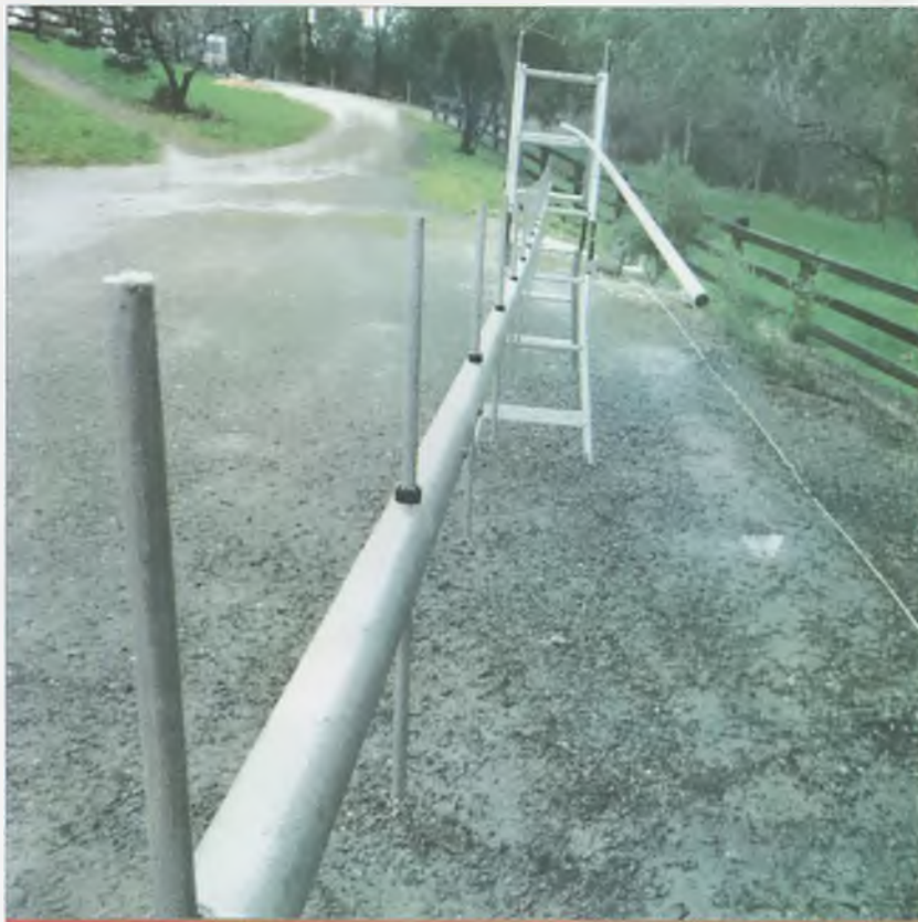
Figure 14. A 70cm Yagi I made earlier!
