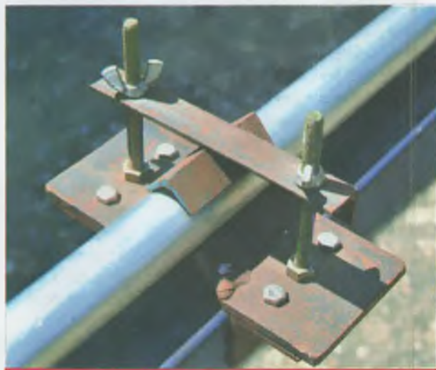
Photo 1. The sliding jig-and-clamp tool essential for keeping the boom aligned during drilling.
