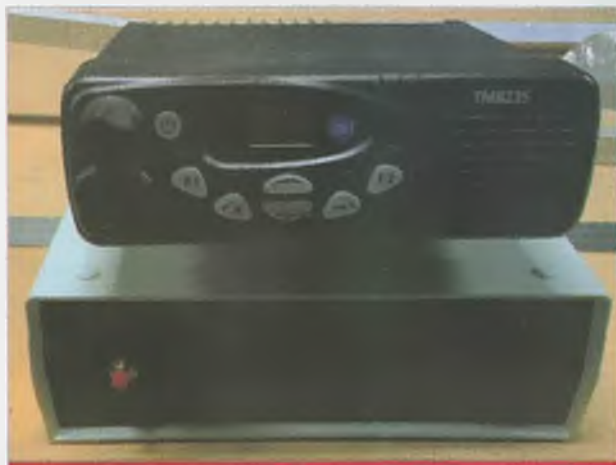
Completed AllStar node - mobile FM rig sitting atop an AllStar node box, ready to go to site.
