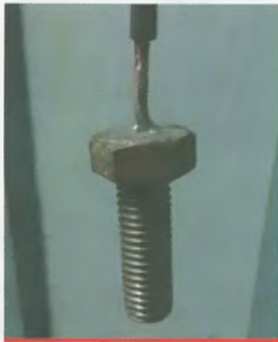
Photo 1. Using a common fluid as flux, soldering to stainless steel is straightforward.
