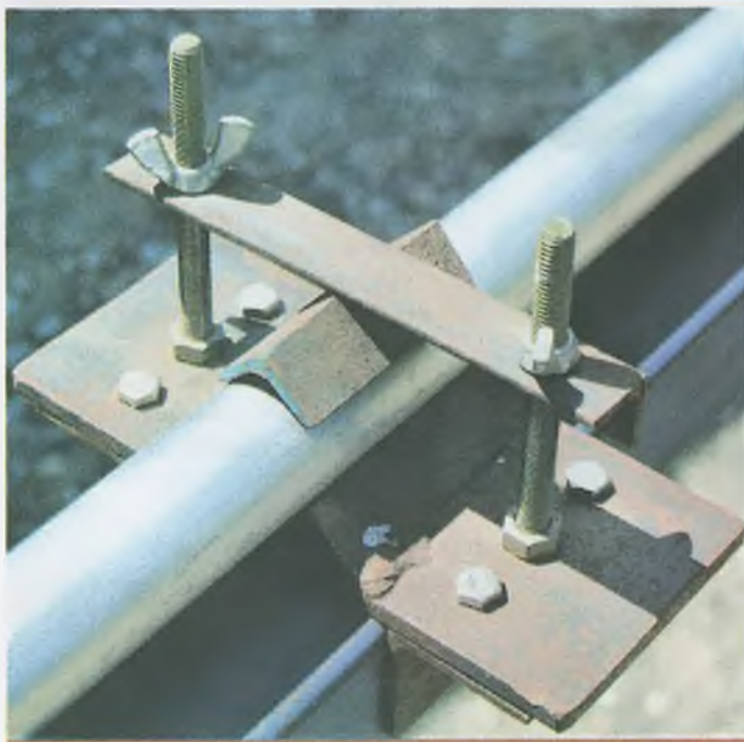
Figure 11. The sliding-jig-and-clamp in situ .
