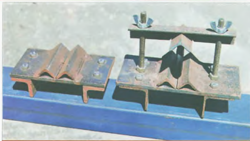
Figure 7. The 'V' jigs: fixed on the left, sliding one at right.
