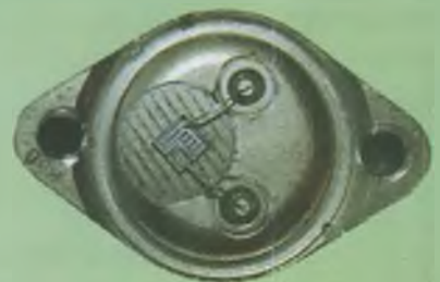
On the inside: Left – a small signal device. Right – a power device; the metal package helps carry away heat. (images: Wikimedia)
