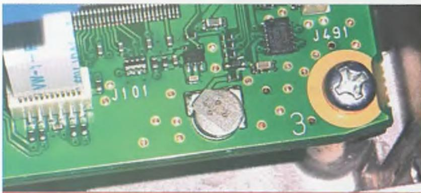
**Photo 3.** The battery is located on the circuit board, next to a mounting post located behind the front of the chassis.
