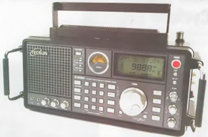
This Tecsun model S-2000 receiver harks back to the rugged case designs of top-shelf units of the past. It is a well-featured rig, covering AM, FM, shortwave, longwave and VHF air band frequencies. Less than \$500 from Tecsun Radios Australia.
