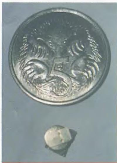
**Photo 1.** The 7300's RTC battery compared to a 5 cent piece, which is 19.2 mm in diameter.
