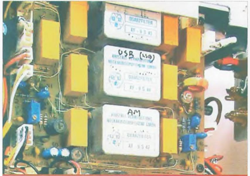
Photo 3A. Showing the three crystal filter units mounted in the transceiver case. The eight yellow blocks are relays.
