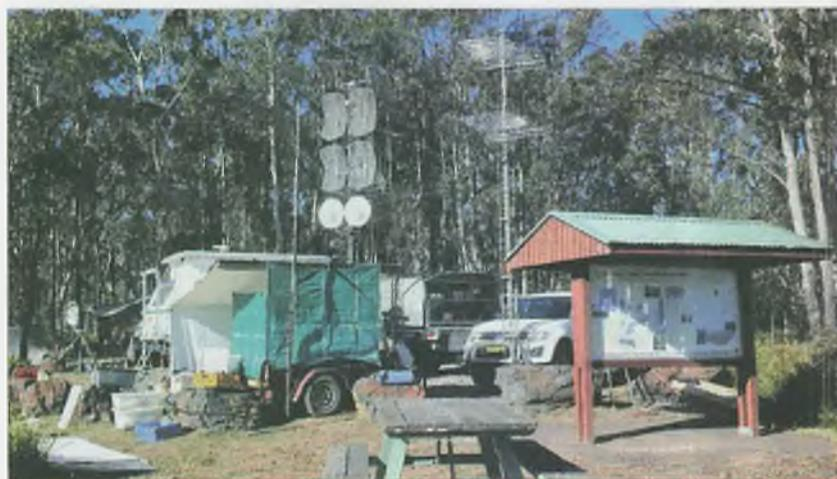
The VK2SRC portable station setup, at Vista Point Lookout for the 2023 Winter Field Day. From far left is 3cm, to its right is the microwave tower with the 23/13/9/6cm antennas, obscured behind it is the rotating pole with 6m and 70cm beams, then 2m at the far right.
