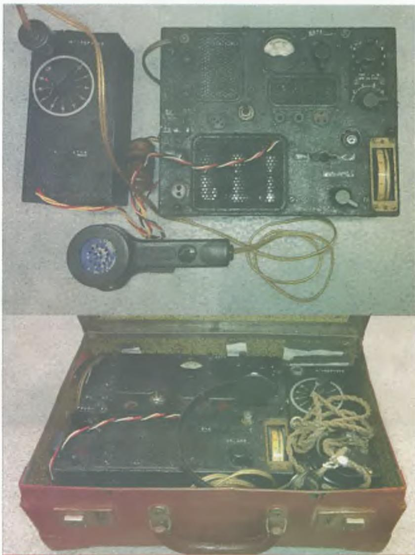
**Photo 4.** The Club's Type A Mark III transceiver; the accessory box (with dial) is a modern addition. These rigs were for WW2 resistance fighters and spies, carried in a red leather suitcase, the 'Go Box' of that era (Photos by Bert VK3TU).
