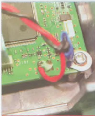
**Photo 6.** Showing the negative lead attached to the mounting screw and acting as a strain relief.
