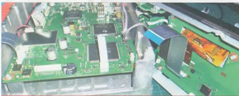
**Photo 2.** Showing the front panel moved aside after dismantling the rig's covers and relevant cables.
