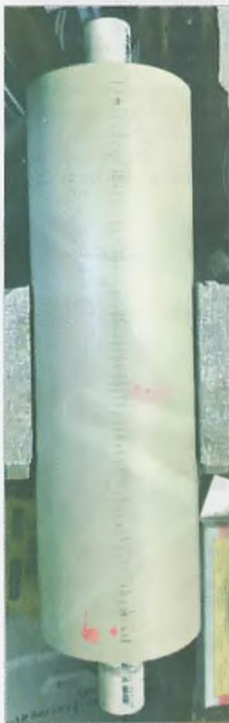
The PVC coil former marked ready for winding.
