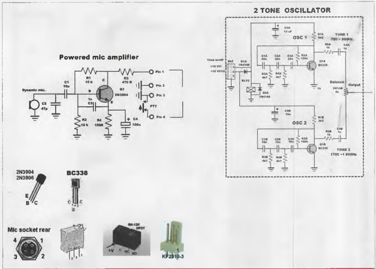
Figure 15. Transmitter two-tone oscillator and power microphone circuit diagrams.
