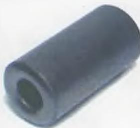
It is suggested that you could slip a few of these ferrite barrels up the feedline coax, right up at the dipole centre adaptor, to make an RF choke – the barrel is an FB43-540002 6.35 mm hole of #43 ferrite, "suitable for sliding over RG-58, and all 195 or 240 cables." – Editor.
