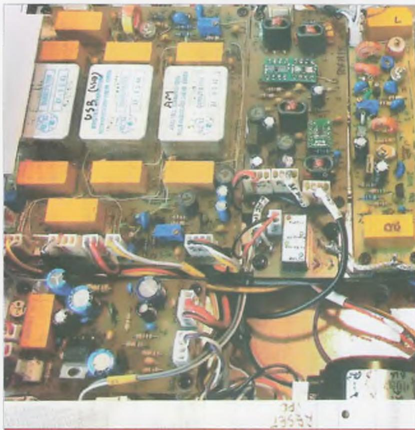
Photo 3B. Inside view of the Mk5, showing some of the receiver boards. The loudspeaker audio amplifier as at lower left, with the crystal filters above it. Immediately to the right is the receiver mixer, then the 20m RF preamp at far right.
