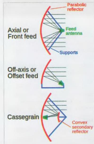
Common, practical feed arrangements for parabolic dishes.
