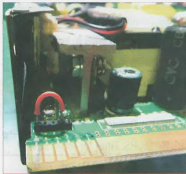
Two pins on a header are bridged to start the supply on its own.
