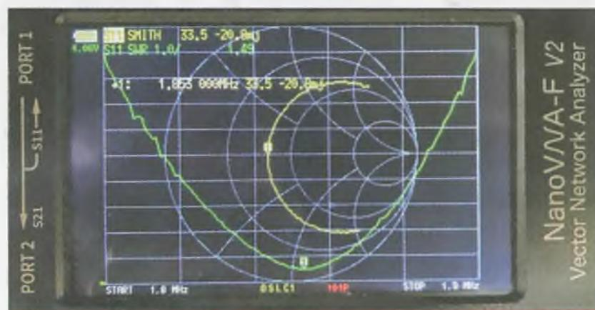
The NanoVNA sweep of my 160m vertical shows it is resonant close to 1850 kHz with a feedpoint impedance yielding an SWR of 1.49.
