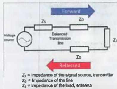
**Figure 2.** The 'workings' of balanced transmission line, such as 'ladder line' or open wire feedline.
