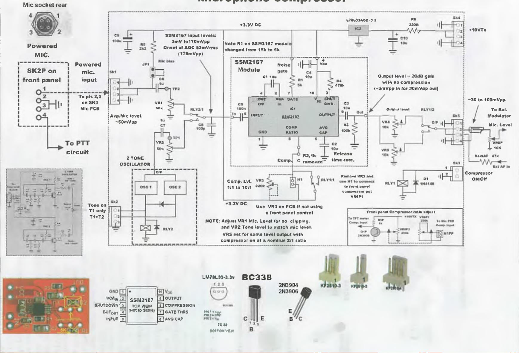
Figure 14. Microphone speech compressor circuit. IC1 is a chip developed specifically for speech processing, providing noise gating and compression in the one device.
