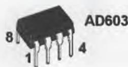
Figure 18. The transmitter power amplifier driver buffer circuit exploits the AD603, a low noise, voltage-controlled broadband amplifier.
