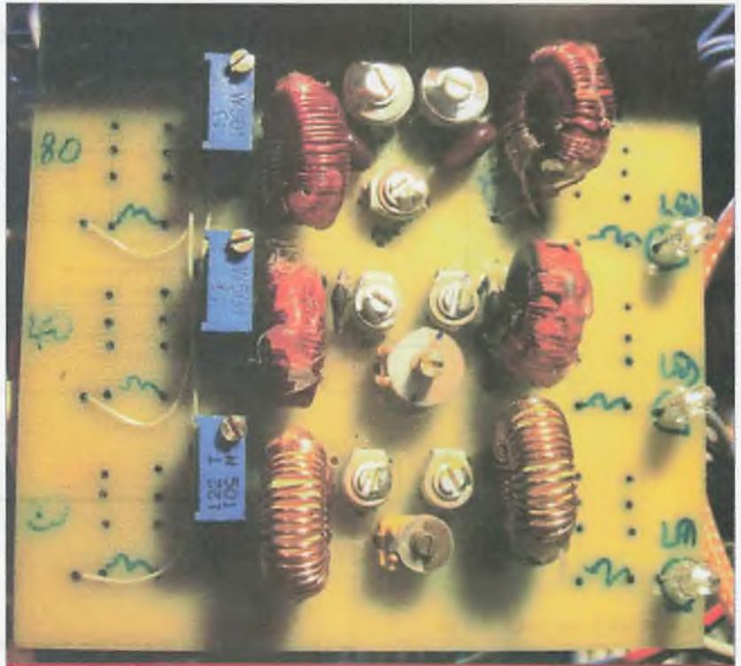
Photo 9. The transmitter band-pass filter board. Note the trimpots at the left. These enable individual adjustment of the transmit power level on each of the three bands so that they're equal.
