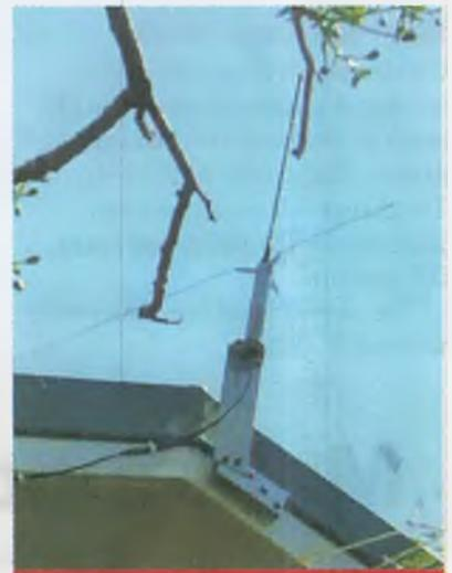
Easy-as: a simple airband ground plane-style antenna is easily mounted to a bargeboard on the gable using TV antenna fixings. This gets the antenna well in the clear, for best listening. (Photo: Doug Friend)
