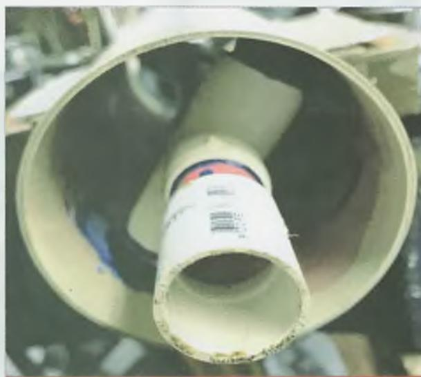
The PVC coil former glued into the 90 mm PVC tube.
