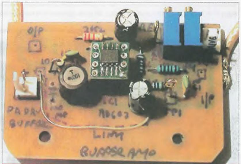
Photo 10. The transmitter power amplifier driver buffer board. The broadband amplifier chip is on the small PCB mounted to the main PCB board on header pins.
