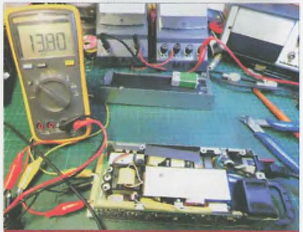
**Bench check.** I successfully set the output of this supply to 13.8 VDC.
