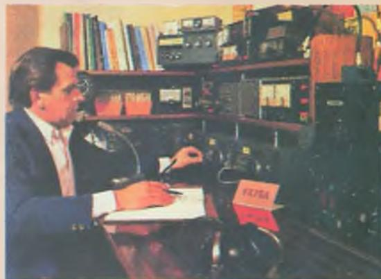
Barry's V175A station featured on the cover of AR, July 1985. The equipment lineup included an IC-751 driving a pair of 3-500Zs in a homebrew linear, and an IC-271H.
