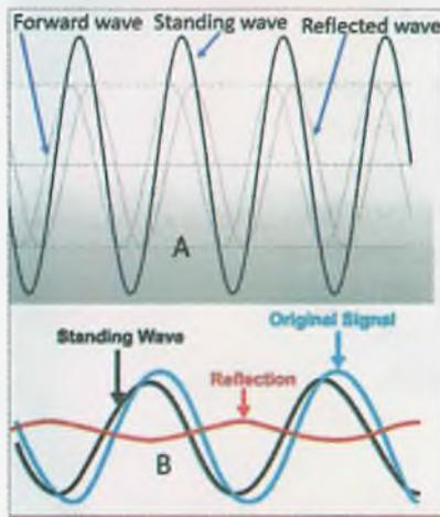
Figure 3. Showing how standing waves are produced.
