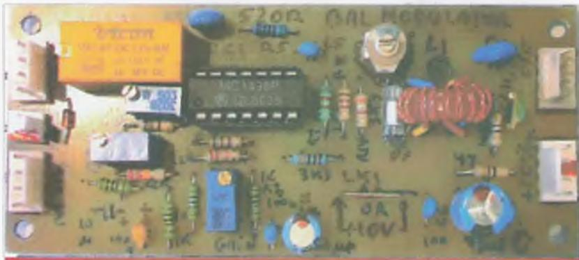
Photo 6. The transmitter balanced modulator circuit board. Note the trifilar-wound RF output toroid and the three trim pots.
