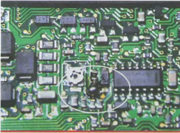
**Volts boost.** A resistor adjacent to the output adjustment pot, is bridged to allow more range.
