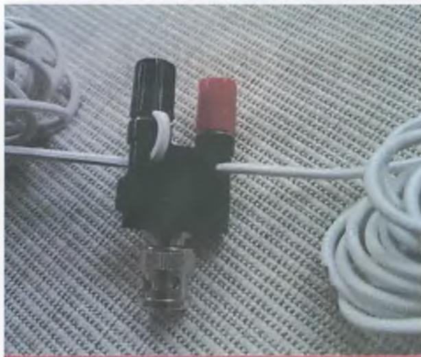
**Threading** the antenna wires through the handy holes in the BNC-to-banana socket adaptor provides strain relief.
