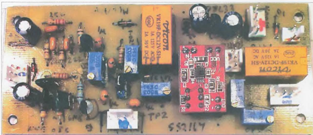
Photo 7. The microphone speech processor board. The small red board at centre-right is the mic preamp/compressor module.
