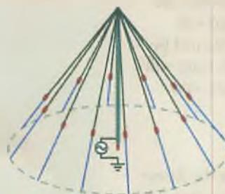
An umbrella antenna is a capacitively top-loaded monopole antenna, consisting in most cases of a mast fed at the ground end, to which a number of radial wires are connected at the top, sloping downwards.
