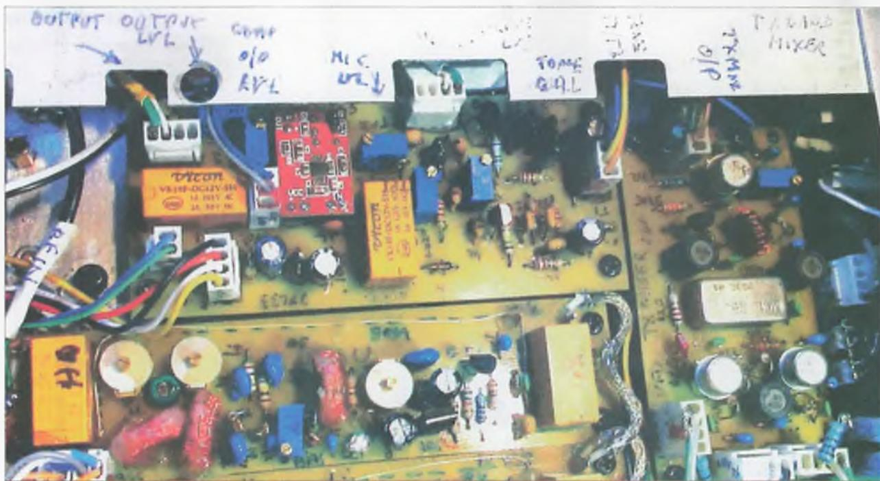
Photo 8. Underside view of the rig's chassis, showing the transmitter's band mixer board at the righthand side. At upper left is the microphone speech processor module's PCB.
