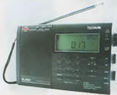
Typical of what casual and beginner airband listeners use is the Tecsun PL660 portable radio. It features VHF airband coverage along with all the major broadcast bands, including AM-MW, FM, shortwave (including single sideband), and longwave. It comes with an inbuilt extendable whip antenna. Around \$200, from Tecsun Radios Australia.
