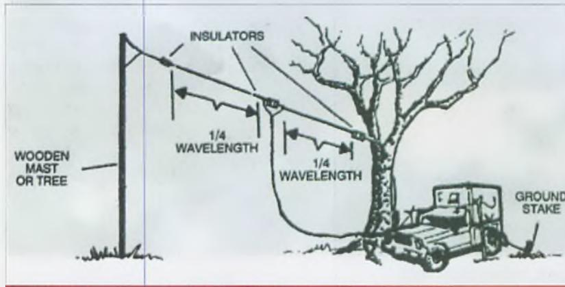
A half-wave dipole, as imagined by an illustrator for a US Army field manual!
