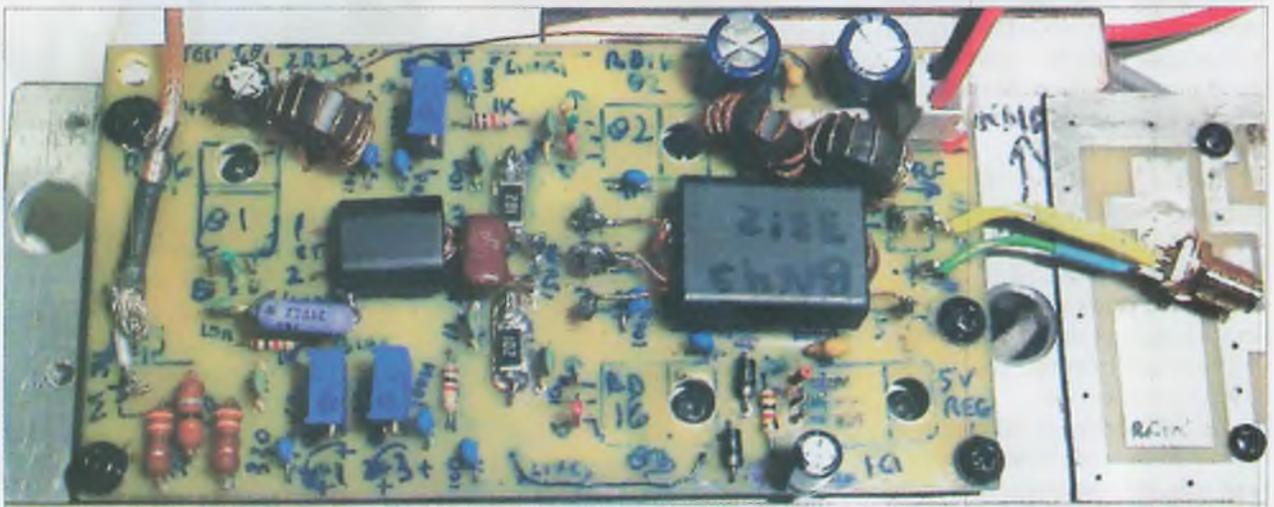
Photo 11. The partially completed 10 W PA driver board for the 3-band transmitter. Note the ferrite core coupling transformers, T1 (left) and T2 (right).
