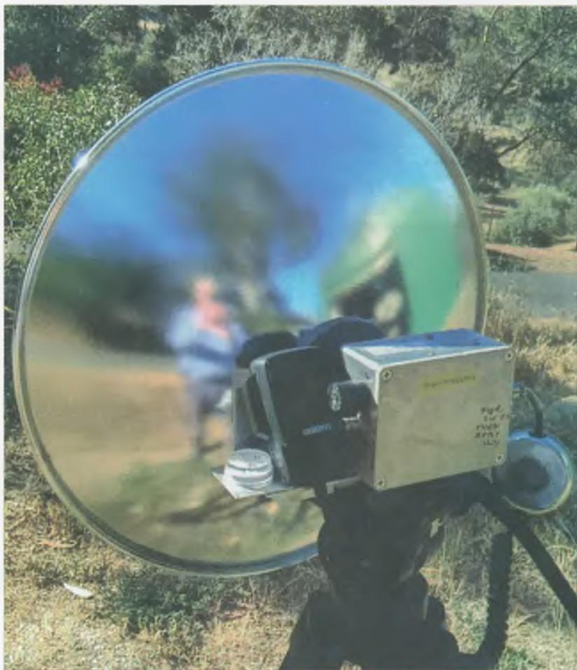
Rear view of my 122 GHz rig. The diecast box houses the 122 GHz PCB, the sequencer and OXCO. Note the bubble level at the left. The round can at right is the mic audio amplifier.
