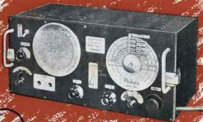
Philips Type R163 Communication Receiver (550 kc/s to 22c/s)
