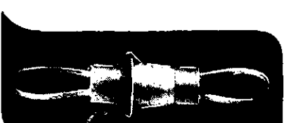
TYPE CAC—Feed-thru flange mounting type can be soldered direct to the chassis or shield plate in tuner units. From 50 pf. min. to 1500 pf. max.
