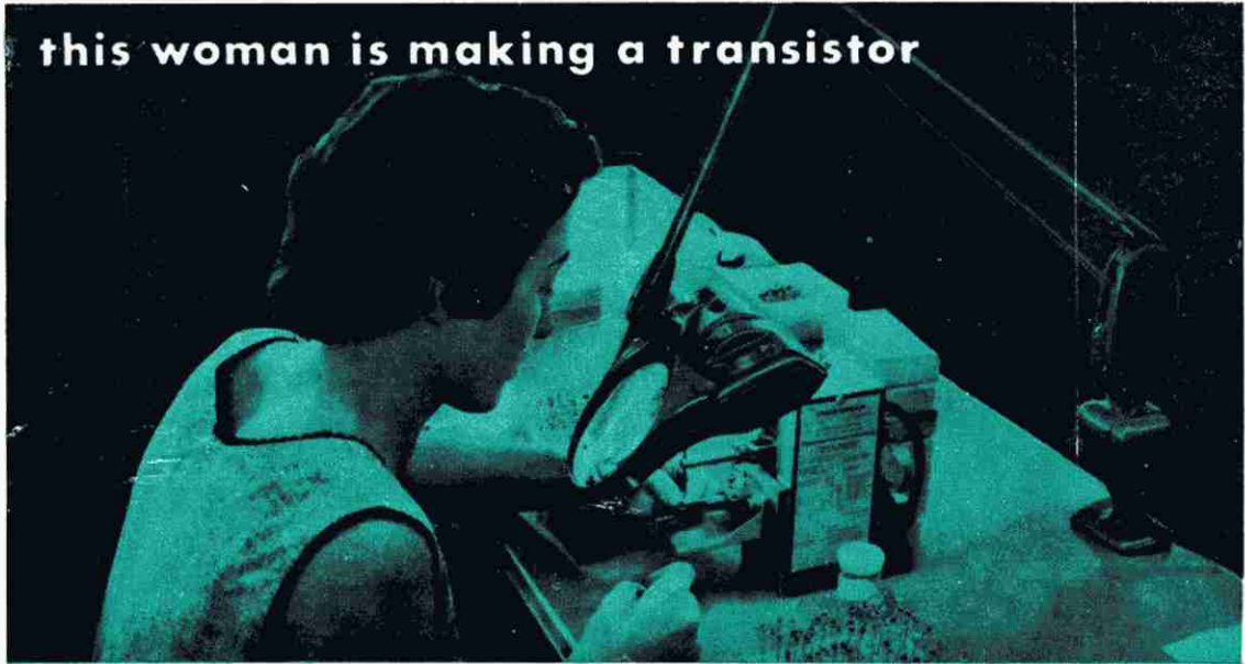
Seen above: "Base tab assembly spot welding", one of the mid stages of AWV transistor manufacture.
