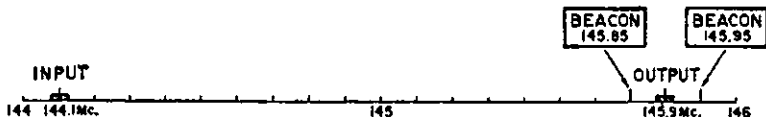
Fig. 2.—The 2 metre spectrum of Oscar III. The 50 kc. input band of the satellite is centered about 144.1 Mc. The corresponding output band is centered about 145.9 Mc. (Inverted). Beacon transmitters are on 145.85 Mc. and 145.95 Mc., bracketing the output band.
