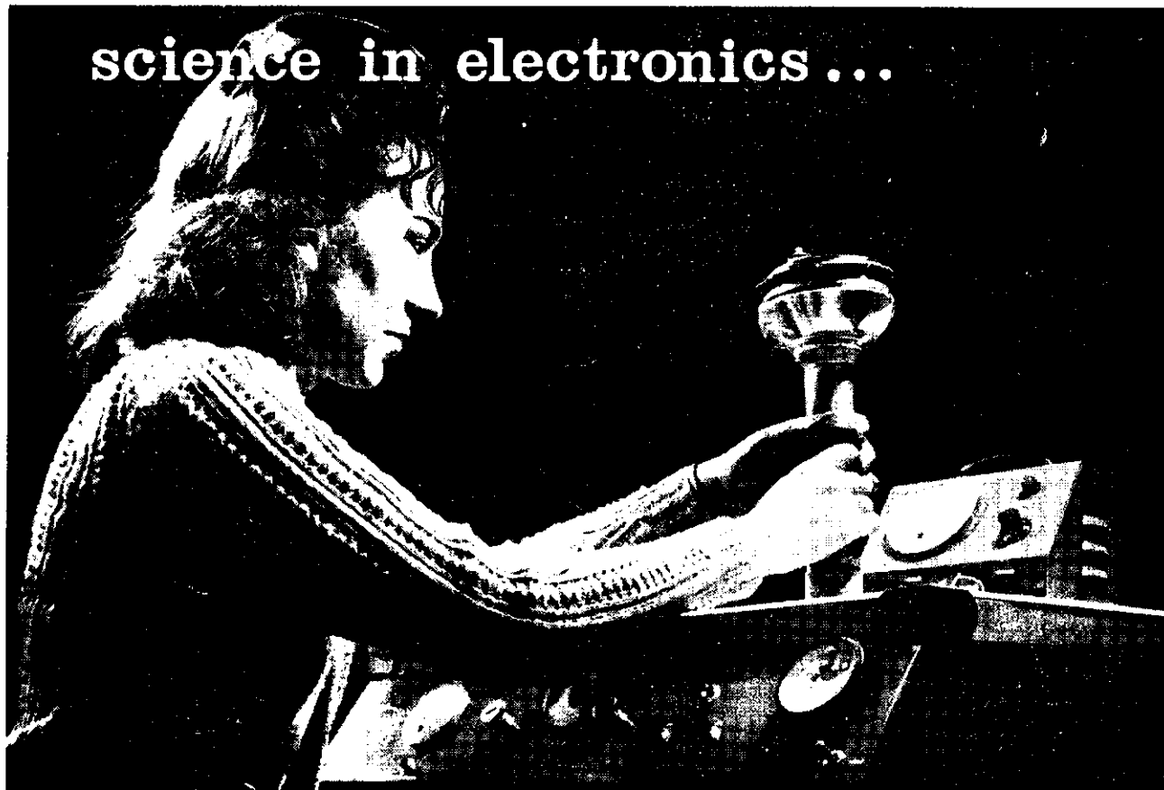
AN AWW 5762 POWER TRIODE IS PLACED IN THE LEAK DETECTOR TEST PORT
