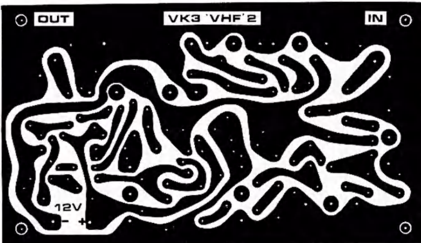
Modified Printed Circuit Board of the VK3 V.H.F. Group 2 Metre Converter
