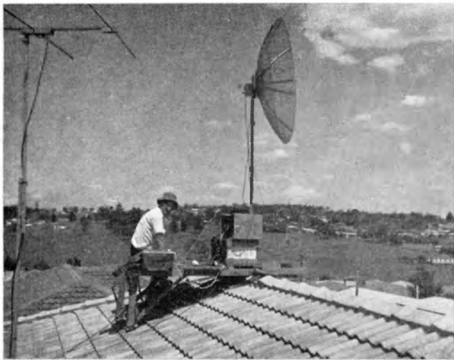
VK4ZT's 1296 Mc. set-up with VK4ZP in attendance. 144 Mc. yagi in corner.
