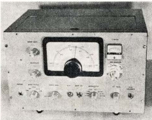
The W5OMX Receiver. Main tuning dial (J. W. Miller, MD-7) has both 6:1 and 36:1 tuning ratios. A 6:1 planetary drive assembly (Arrow Electronics, Type 4511) is used on the pre-selector tuning capacitor. The pointer is home-made.
