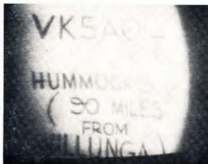
Picture received at Willunga Hill. Camera and monitor was enclosed in a light-proof housing. The actual distance scaled from the Adelaide Land Department map was 93 miles.
