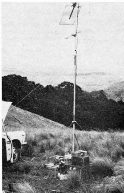
VK4KE/P at Mt. Mowbullan, Bunya Mts. 1296 Mc. equipment and corner reflector antenna; 3 el. 144 Mc. yagi. (53-mile contact with VK4ZT at Toowoomba.)
