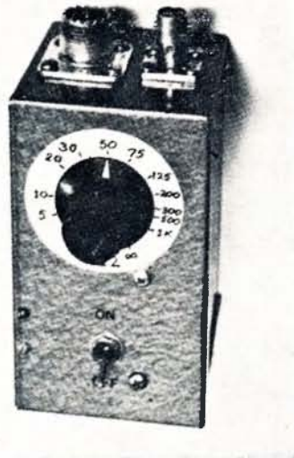
Recommended replacement for the common v.s.w.r. bridge—the radio-frequency bridge and noise generator.
