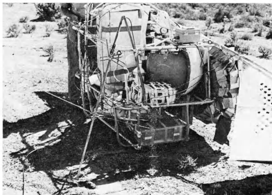
The gondola after landing. The 144/432 MHz. antenna can be seen (somewhat bent) in the foreground.
