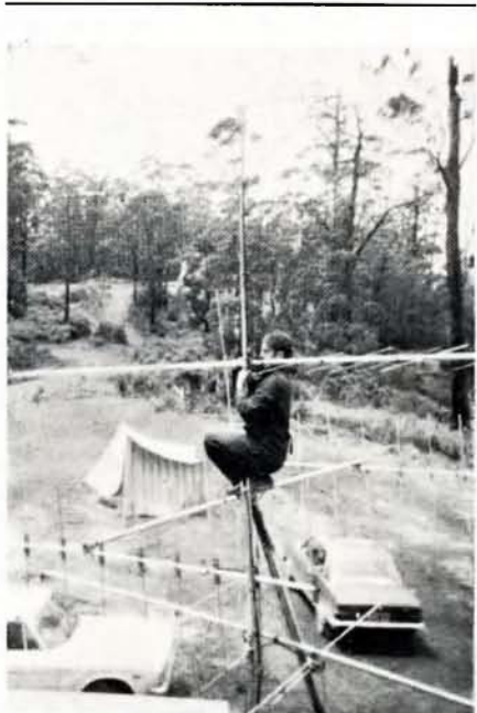
John VK2ZJQ adjusts a 10 el. 2 metre yagi. Top antenna is a 15 el. 432 MHz. yagi. Beneath John are a pair of 146 MHz. vertical 10 el. yagis and a 4 el. 6 metre yagi. The tent in the background housed a 2 kva. motor-generator set. These aerials were in use by VK3AOT/P at Mt. Cowley from 18/12/70 to 2/1/71.
