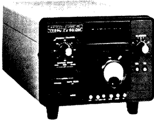
FV-901DM Synthesized, Scanning External VFO Flexibility in frequency control; PLL synthesis in 100 Hz steps; auto scan mode, which will search the band for a signal; manual mode which scan at one of three rates while you activate lever switch. Memory bank for up to 40 frequencies and clarifier for fine tuning between the 100 Hz steps. etc.
