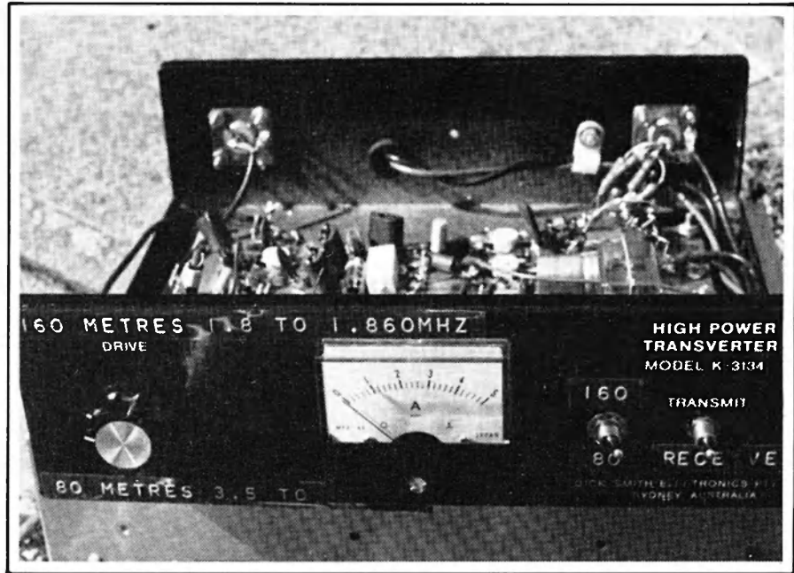
Front view of transceiver. Notice that 160 and 80 Mx can be selected at the flick of a switch.
