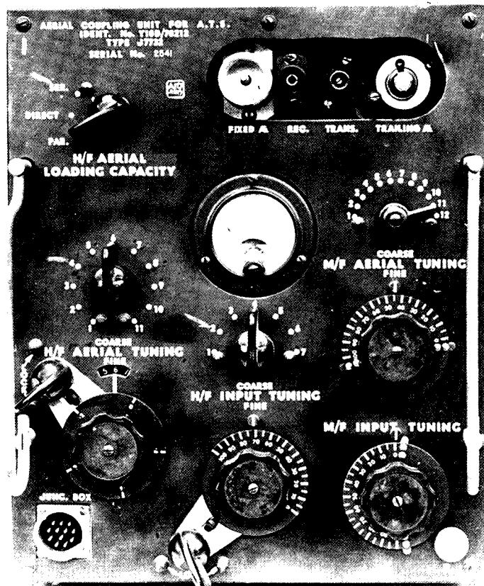
RIGHT: Photo No. 12, AT5 Aerial Coupler
