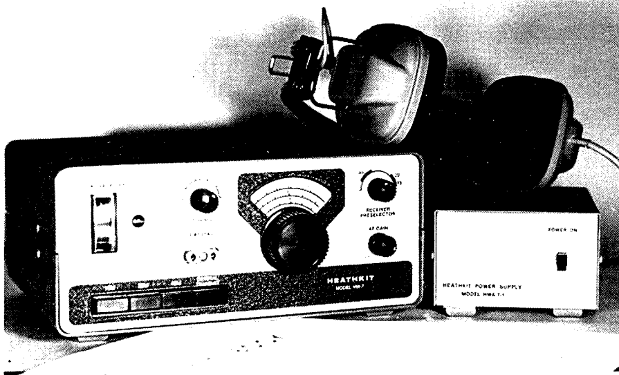
PHOTO 2: One of the popular QRP rigs — the HW7 now superseded by the HW8.
