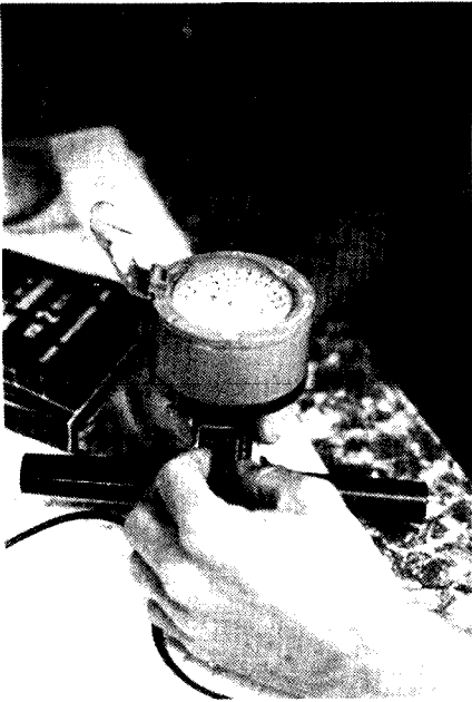
PHOTO 3: Using the Brookes and Gatehouse RDF hand held antenna to find the bearing of radio-navigational beacons. The operator uses headphones and rotates the antenna until a null is found.
