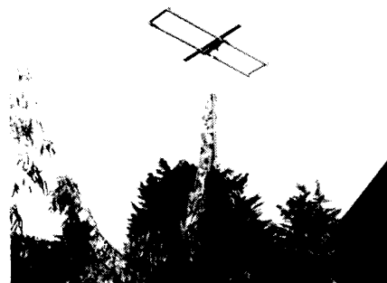
PHOTO 3: Three element beam. Note shorter support for reflector and director.
