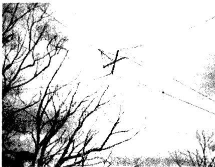
The main body of the multi-band vertical sloped down 45 degrees from the tree to the feed-point. The inverted L sections for 3.5 and 14 MHz extended out to the sides.
