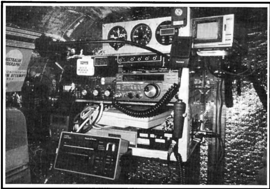
The control console in the gondola. Note the amateur radio installation. (Photos courtesy Australian Geographic)
