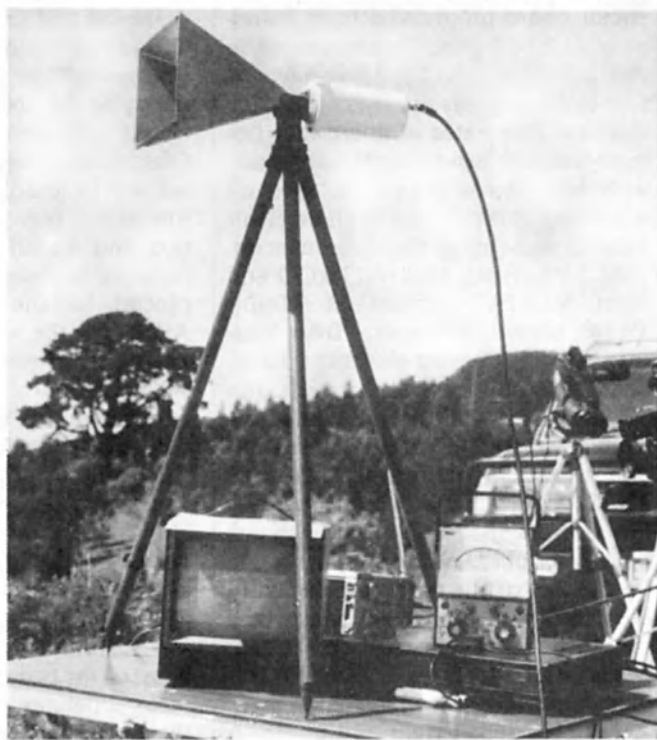
10 GHz Horn Antenna, and equipment used by the group as successful back up equipment.
