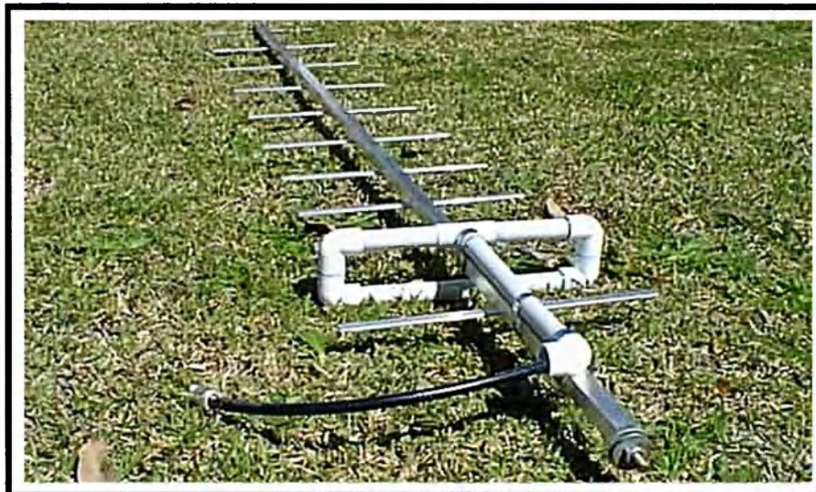
The completed 11 element 435 MHz Yagi before mounting in the air.
