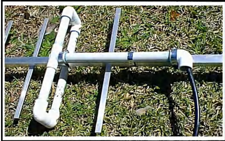
A close-up of the folded dipole and feed. (Photo by VK6UU) (Colour original inserted)
