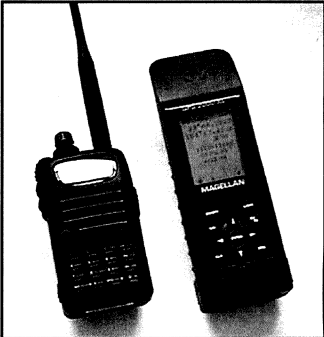
The Magellan GPS-2000XL Mk3 receiver is slightly larger than the Yaesu FT-50, but is lighter by 67 gm.
