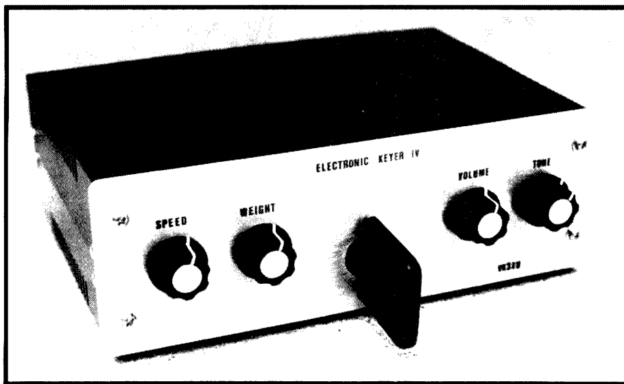
The three-chip electronic keyer in its case.
