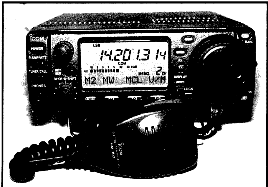
The Icom IC-706MkII HF + 6 m + 2 m all mode transceiver and the matching HM-103 handheld microphone.
