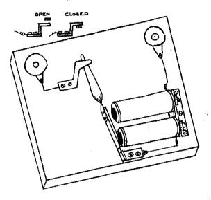
tension, when the relay is in the open position. Screw the other end firmly to the baseboard.
