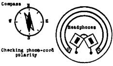
tion of the needle in a reversed direction. Check both phones and the polarity of the magnets and then remove the magnets.
