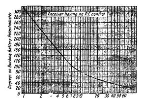
generator. These points may be plotted on semi-log paper, degrees of potentiometer dial against ratio of antenna current increase. Fig. 3 shows a typical set of curves, overlapped.
