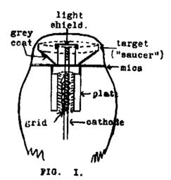
In appearance, the 6E5 is like any other valve; in internal construction, it is totally different. The chief feature of its design is a concave metal "faucer" situated in the top dome of the glass envelope, and coated with a grey fluorescent layer. (See Fig. 1.) In the centre of the saucer is a hot Cathode, shielded from outside light sources by a small black metal cap. Underneath, in the body of the valve, are a continuation of the Cathode, a Triode plate and a Triode grid. (The control grid.)
