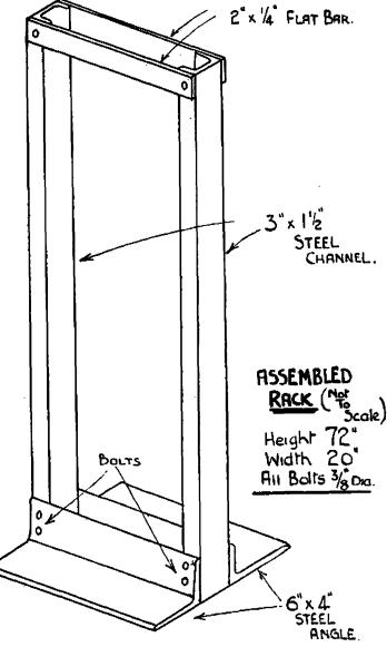
The materials can be bought from any steel merchants at a cost of 25/to 30/. The steel will be cut to the required length, and should need no further machining. To make sure, add a rider to the order stating you want the steel cut to the exact lengths.
