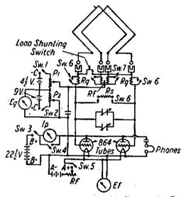
Fig. 3.—Circuit of Field Strength Set.
