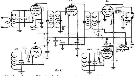
It should then be possible to find a peak on the three plate trimmer across the first detector grid coil. If not it may be necessary to slacken off the grub screws holding the 5 plate condenser tuning this coil and to rotate it independently of the oscillator tuning condensers to find a peak. If this is the case it indicates that the coils need pruning.
