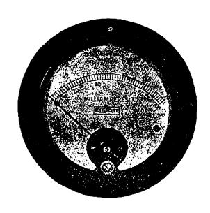
Stocks of minature instruments available for D.C., A.C. and R.F. measurements in moving coil, moving iron, thermo couple, rectifier pattern
