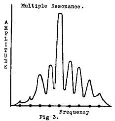
3. Each separate resonant peak can be seen on a sensitive wavemeter and also heard on tuning to a weak carrier and listening on either side of the main peak.
