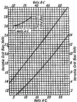
Fig. 4.—Conversion Chart for the Lower Values of Grid Blaa.
