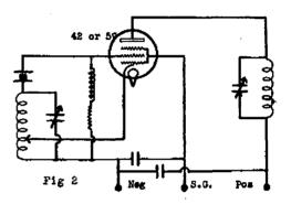
tap on the oscillator grid coil just as in the case of an electron coupled oscillator circuit. This allows one to shift the frequency of the oscillator but still maintain the note and stability of CC. The circuit has been fully tried out and is worth using.—VK5KL.
