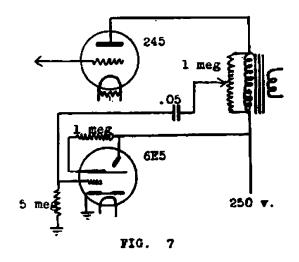
The mechanical installation of the 6E5 should be effected in such a manner as to keep the target reasonably shielded from outside light sources, in order that the angle may be readily observed.
