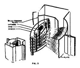
SKETCH SHOWING FORMATION BY GRID WIRES OF BEAM SHEETS
