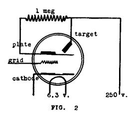
When the grid is -8 volts with respect to the Cathode, the shadow-angle is approximately 0 degrees. (Fig. 3.) When the grid is at 0 the angle is approximately 90 degrees. (Fig. 4.) When the grid is negative to a further degree than -8, the shadow-angle is not only at zero, but the two edges of the green arch overlap, forming a small angle of a slightly brighter green. (Fig. 5.)
