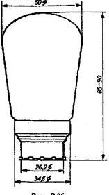
Base P 35 Normally the valve is delivered with the base P 35
