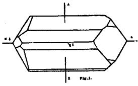
and, due to its more complex chemical structure, is usually found to contain more impurities than quartz. These impurities give it the characteristic colors ranging from yellow through blue to black. The black variety is opaque, and this form (known as schorl) is generally unsuitable as an oscillator.
