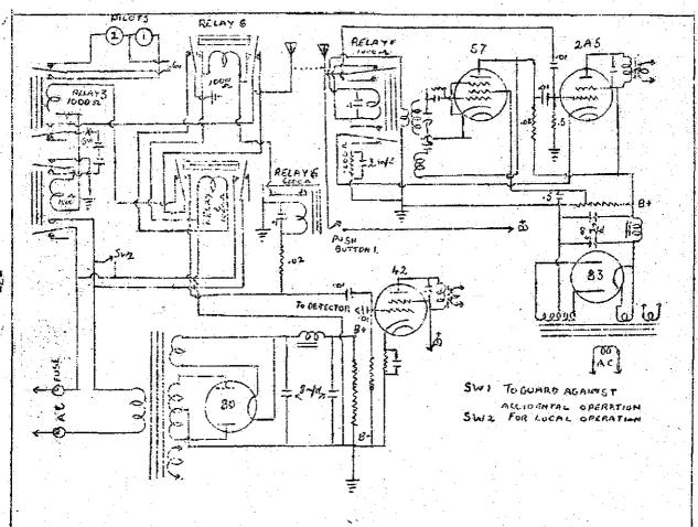
This is the first half of the operations and BCL is still in normal operation with the exception that the grid of the 2A5 is switched to line.
