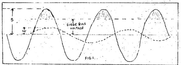
If now the amplitude of the signal is varied by modulation there will be a change in the height of the voltage peaks, therefore an increase or decrease of diode conduction, and this in turn will change the bias voltage so that conduction occupies
