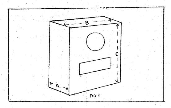
In the following table dimonsions are given for various sizes of speakers. A.B. and C represent the measurements at the points indicated on the sketch.
