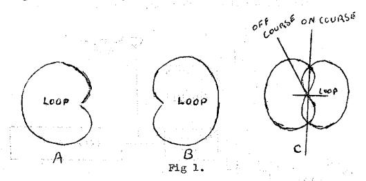
If the connections to the loop are reversed, the pattern will be as in fig. 1B. i.e. the maximum signal will now come in along the line that previously gave minimum response.
