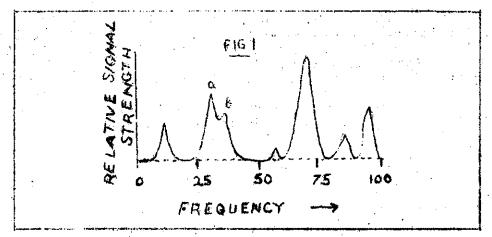
The station to which the receiver is tuned appears in the centre of the screen, while stations above this frequency appear on the right half of the screen and stations of lower frequency on the left half. The band-width represented by the graduated horizontal scale can be varied from 0. to 100 kc or more. The stronger the signal, the higher its "peak", so that relative strongths can be seen at a glance.
