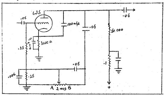
With the arm of the potentiomoter at A, the 250,000 grid resistance is shorted out and the .05 mfd plate condenser is connected as a bypass to ground, giving maximum bass. With the arm at B the .05 mfd bypass is high above ground and the foed-back voltage is maximum, with feedback taking place only at low frequencies, due to the .006 grid shunt. The high audio frequencies are passed and the lows attenuated at 'B'.
