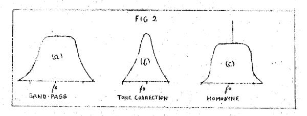
If wanted and unwanted signal reach the detector with equal amplitudes, the result will be a hopeless jem; but if we can add to the desired signal an artificial carrier of just over 30 times the existing carrier strength of either, we immediately obtain a rectifier discrimination of 2 S2/W2 equivalent to 66 db and reception is perfect without any disturbance of the
