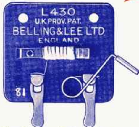
Current in excess of rating—clip jaws open, releasing the trip wire, thus opening the circuit.
