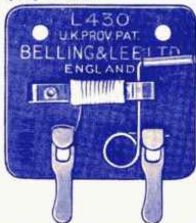
Trip wire reset by springing it back into clip jaws.
