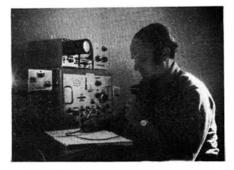
The monitorscope can be seen on top of Cor's allband phasing rig.
