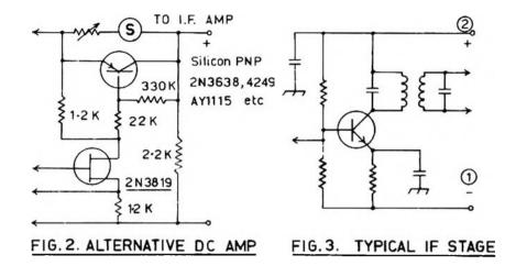
R1, connecting to the SSB detector output. 2. Strong signals do not cause full scale reading. Remedy: adjust resistor in series with the meter.
