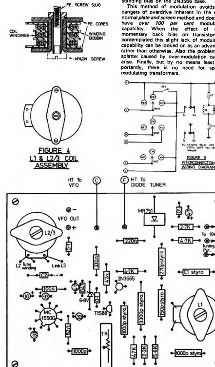
output from the PA in the CW mode is reduced to half before applying modulation. This is achieved by means of the 5K linear pot across the supply rails which sets the standing bias on the 2N3566 base.
