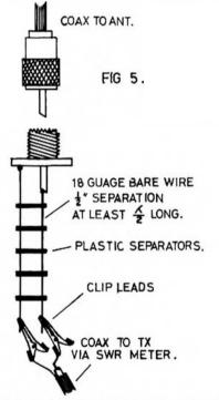
off its ends. The antenna was fed as in Fig 5. Clip leads are slid up and down the parallel wires until a low impedance point is found. This gives a low SWR on the coax line to the transmitter. A tuning unit could of course be used but the method shown is very simple, very cheap, and most important, very effective.
