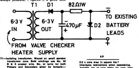
Interleave laminations when assembling. \*middle leg of core taken for core area. D1—Low voltage silicon power diede (25 PIV minimum).
