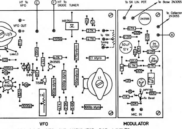
FIGURES 6 & 7 - VFO AND MODULATOR PCB. LAYOUTS
