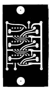
Fig. 3—Copper Copper side of display board (actual size).
