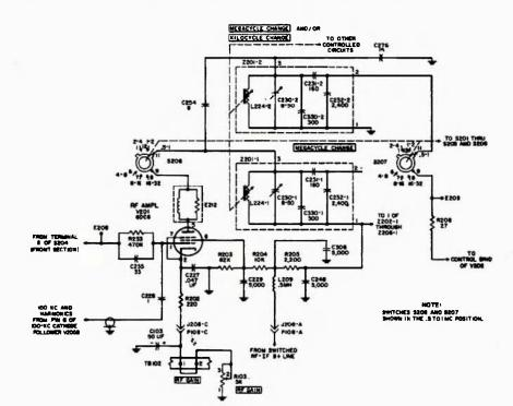
Figure 1. Rf amplifier V201, schematic diagram.
