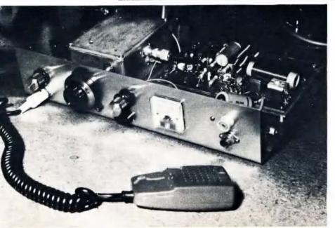
Since silver mica capacitors are no longer stock items in supply houses they were not used in the frequency determining parts of the VFO. Instead, use was made of the freely available *Styroseal* components. They should be used where so indicated in Fig 1. Ceramic disc capacitors should **NOT** be used in place of the styroseals although silver micas could be substituted if on hand.
