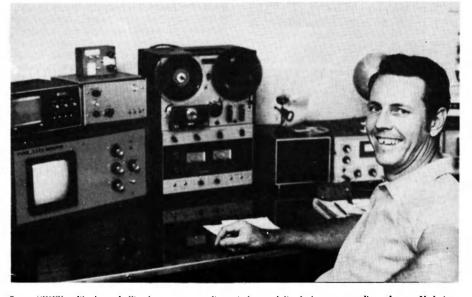
Doug VK8KK with home-built slow ecan monitor at lower lell, faat scan monitor above, Akai tape recorder, and FTDX490 transcelver.
