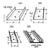
Fig. 3.—Details for forming channel type heat sinks.
