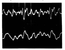
PHOTOGRAPH 2.—OPERATION OF FREQUENCY MALVER Horizontal scale. 1 Division 2ms Upper trace. Typical audio inpul. Lower trace, Hail frequency audio output.
