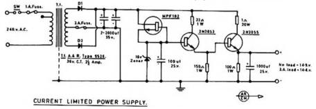
The emitter resistor of the 2N3053 shows 150 ohms. This should be increased to 1000 to 1500 ohms.
