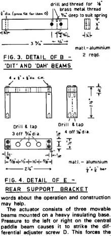
outer "dit" or "dah" beam to move out and close the contacts C. The opposite beam remains stationary as it is held by the spring H against the steel pin K which acts as a
