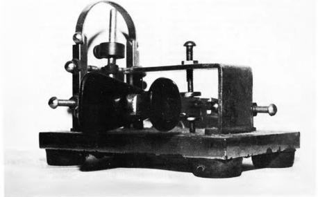
PENDAGRAPH with a difference. Unlike most, the paddles are at right angles to the key — after the design of the SIMPLEX.
