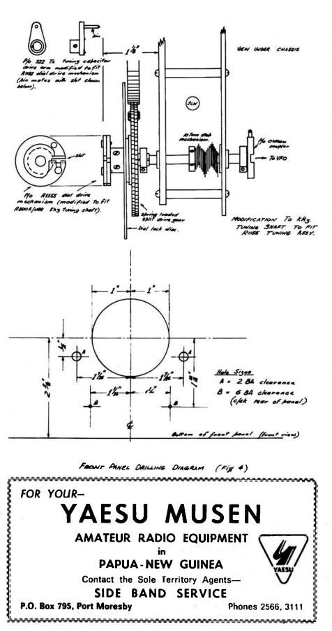
approximately 6.5kHz per revolution. have attempted to show in Figs 3 and 4 as much detail as possible as to how this was done, and the drilling template for the style of knob used. I say this because information recently received leads me to believe that there were a number of different style knobs used on the R1155, and there could be some minor changes in the measurements.
