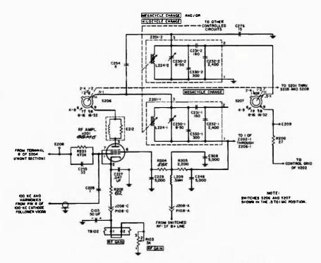
Figure 2. Rf amplifier V201, schematic diagram. (modified)
