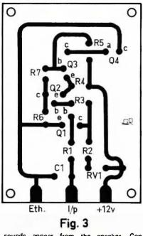
sounds appear from the speaker. Consequently I have made RV1 a trimpot and mounted it on the Vero board with the rest of the circuit.
