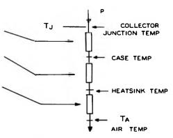
mounted on a 12" piece of 55D heataink. This is cost prohibitive and physically ridiculous. The best compromise is probably 4 transistors each on a 2" piece of 'Miniwatt 55D' heatsink.
