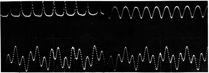
PHOTOGRAPH 3.—ENVELOPE WAVEFORMS Horizontal Scale. 1 division 1 ms. Upper Trace. Two tone audio inpul. Lower Trace. Envelope waveform produced by computer. This waveform corresponds to that defined in equation 4.
