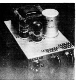
nor even unusual. It uses an orthodox audio amplifier followed by an orthodox twin triode clipper. This stage clips both positive and negative signal peaks. If run below the clipping level it acts as a low gain amplifier with good distortion characteristics. This clipping stage is followed by a single RC filter to remove the harmonics produced by the clipping process. The circuit requires but few comments—
