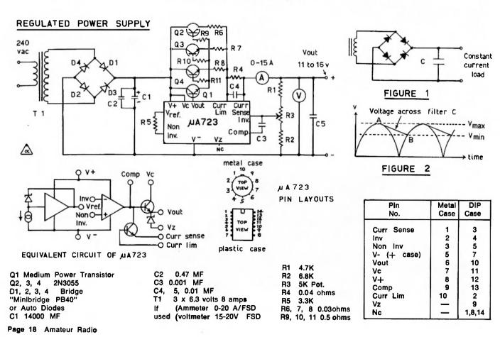
For satisfactory regulation, the input to the regulator must be about +4.4 volts higher than the required output voltage. Therefore assuming +13.9 volts to be the maximum voltage required at the output, the minimum voltage which may appear across the filter capacitor is
