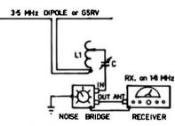
FIG\_1 TO DETERMINE ANTENNA RADIATION RESISTANCE
