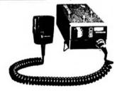
MODEL SR-C430, 10W, 12 channel plus memory channel, Mobile FM 12V DC Transceiver for 420-450 MHz Amateur Band use. A superb compact unit, measures only 84 (w) x 58 (h) x 235 (d) mm, weight .96 kg. PTT microphone has a built-in switch to enable convenient selection of a priority channel (memory channel). Complete with microphone, built-in speaker, snap-clip mobile mount, power cable, DC line filter, stand for base station use, and crystals for 435 MHz. Price \$295
