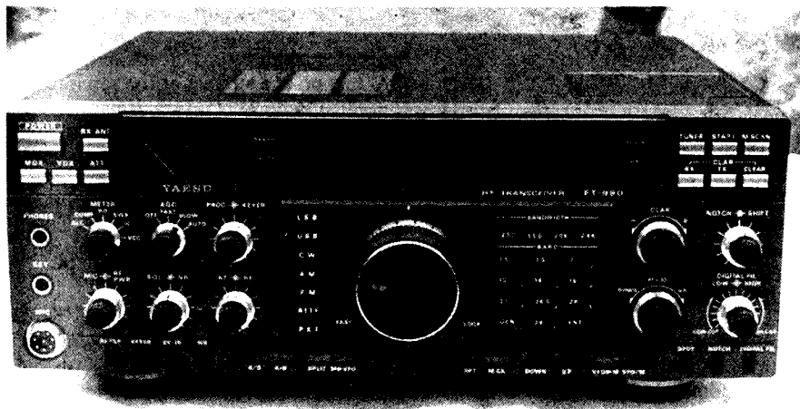
This front panel view of the FT-990 shows up the family resemblance to the FT-1000.
