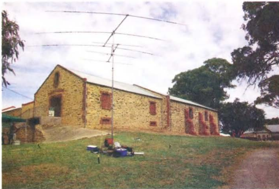
HF triband antenna over a three element Yagi. Portable mast and antennae loaned by Paul, VK5PH.
