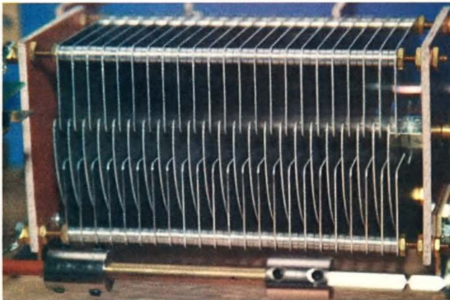
Photo 4: Close up of the differential dual gang capacitor.
