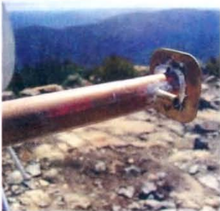
Photo 5: The plate/dipole feed for 3.5 GHz.
