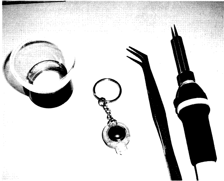
Essential tools: from left, magnifying glass, small spotlight, tweezers, soldering iron.
