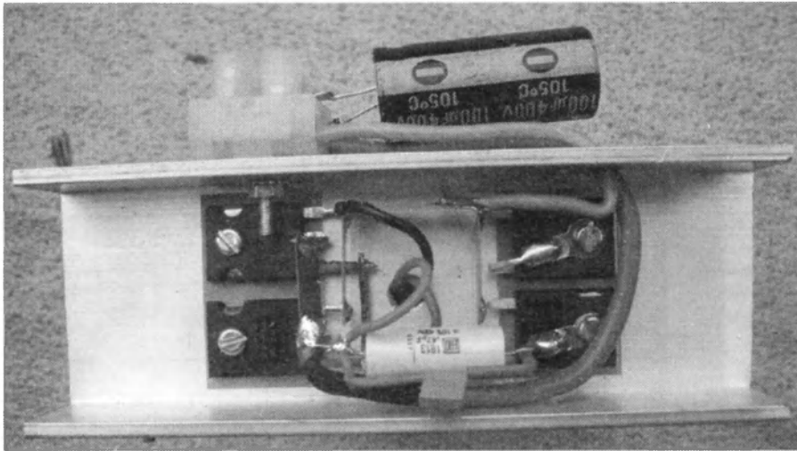
Photo 2: Mounting the MOSFETs and damper diodes. Note the thick short leads used even at audio frequencies to minimise switching times and avoid ringing.
