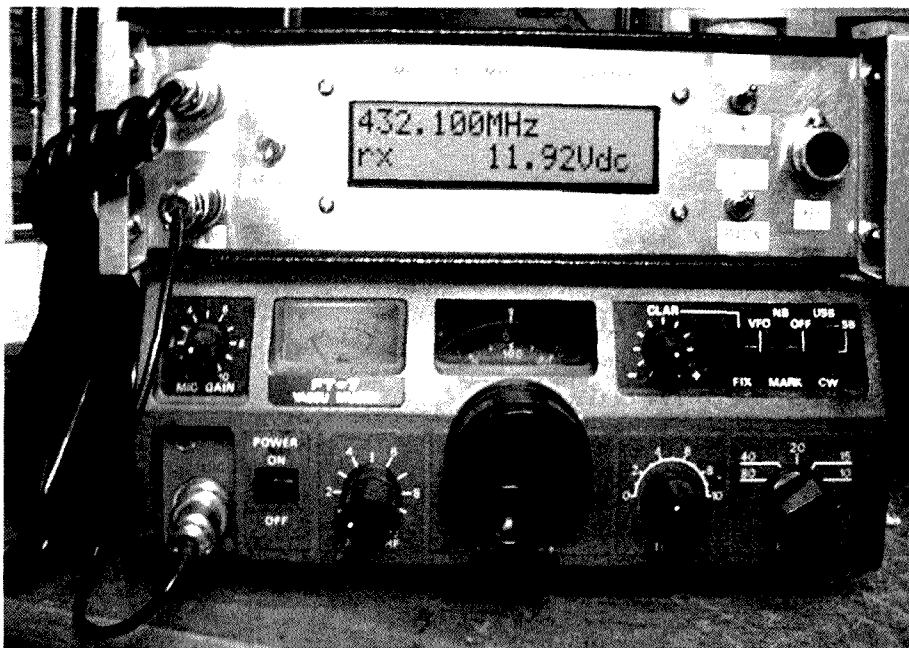
Figure 2: The transverter unit mounted on top of the FT-7 transceiver.
