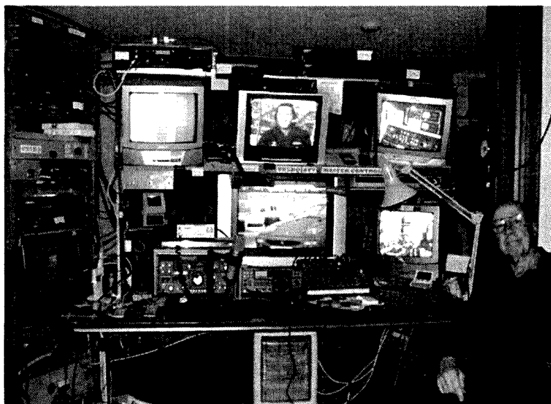
Photo 2: ATV signals being received by Barry VK5BQ – Top L to R, Maitland VK5AO on 2.4 GHz, 86 km; broadcast.TV; Ben VK5RD on 10.35 GHz, 68 km; Bottom L to R, Graham VK5JD on 1250 MHz, 82 km and Maitland VK5AO on 5.76 GHz.
