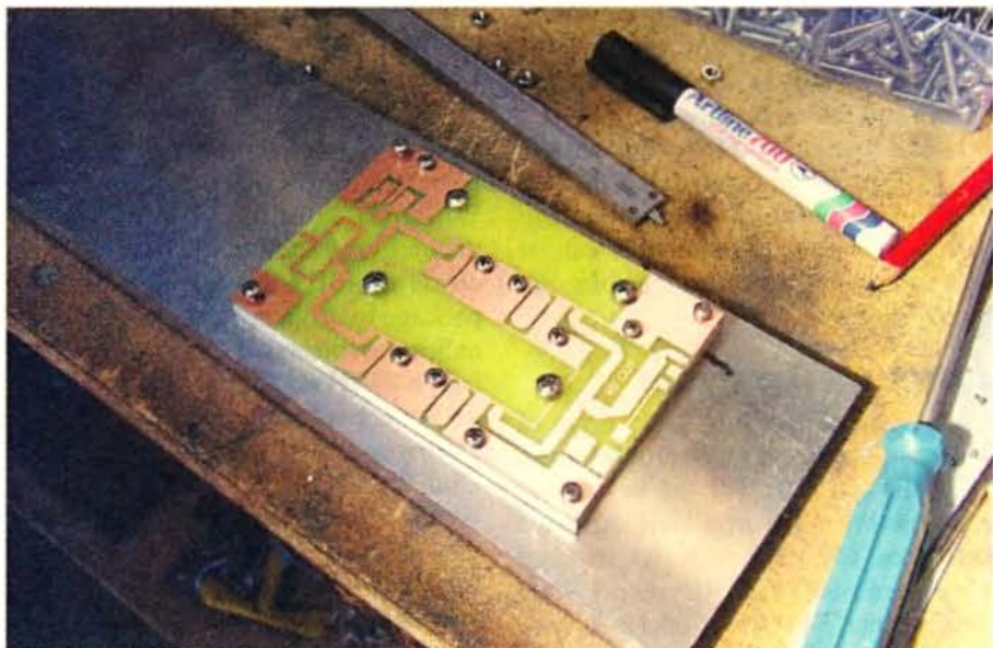
Photo 1: Trial assembly of the circuit board on its mounting base.
