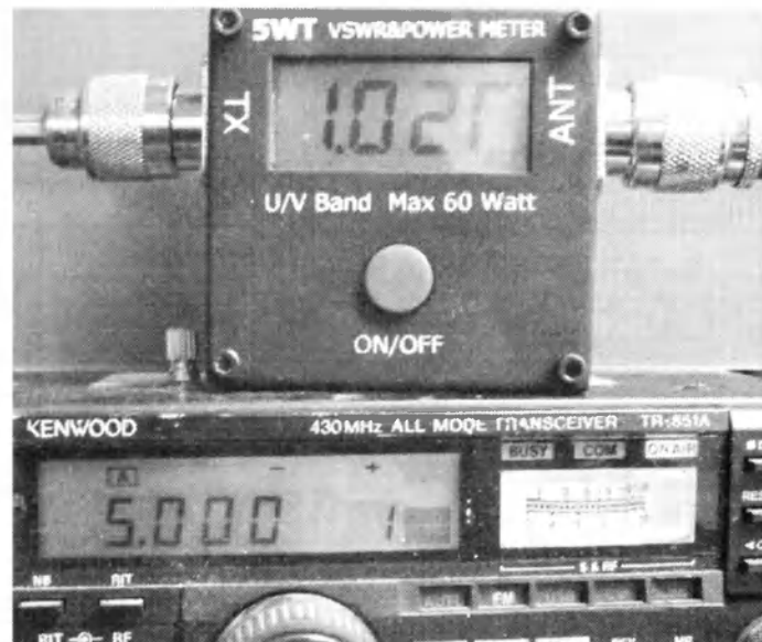
Photo 6: Prototype 70 cm beam driven with 25 Watts at 435 MHz.
