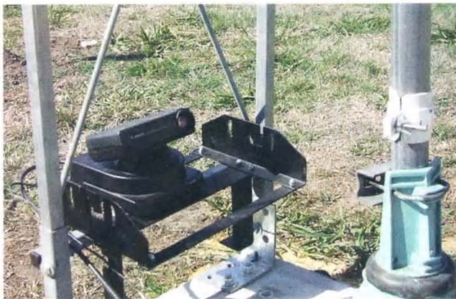
Photo 1: Camera aimed at compass scale on mast.
