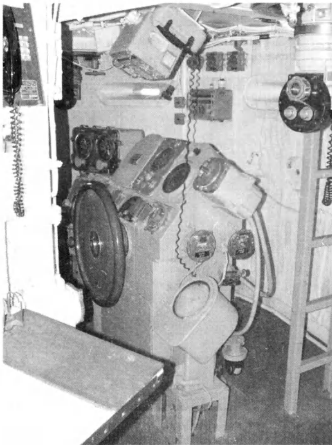
Fortified bridge within the main bridge structure enabling navigation of Missouri whilst under attack. NB: Periscope, wheel, and 'peep' slots in the 300-400 mm steel enclosure.
