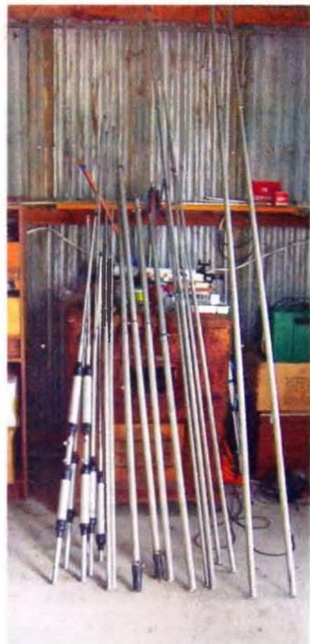
Photo 7: The TH6DXX elements assembled and ready for erection.
