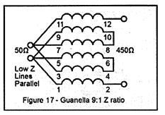
Figure 17: Schematic diagram of a 9:1 Guanella balun.
