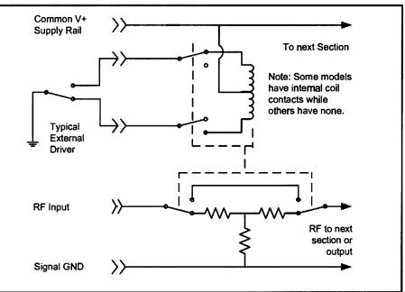
Figure 2: An attenuator section electrical diagram.
