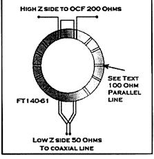
Figure 15: Balun wiring.
