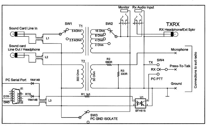
Figure 1: Schematic diagram of interface. Note that the two 1N4148 diodes are mounted in the connector back-shell and that L1, L2 and L3 are common mode chokes made from wrapping the cable through ferrite tubes. The chokes should be as close to the PC as possible.
