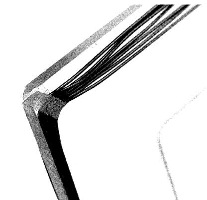
Photo 3: One corner of the loop, showing turns wound side by side in the notch.
