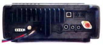
Photo 2: A view of the rear panel of the IC-7200 with the PSU cable plugged in. The connection to the external ATU is to the left of the power plug; the USBB connector is to the left of the Remote and External Speaker jacks.
