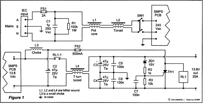
Figure 1: The circuit diagram.
