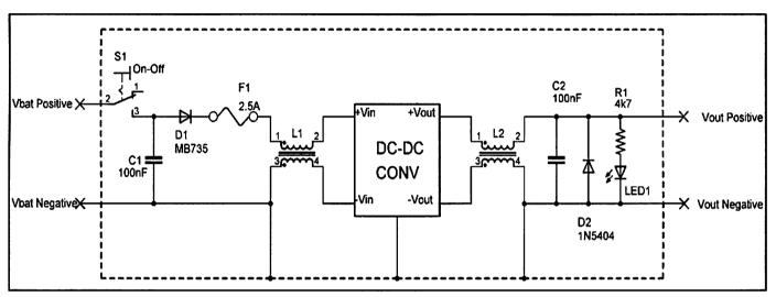
Figure 2: Schematic diagram of power supply.
