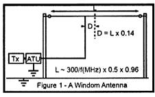
Figure 1: The schematic of a Windom antenna.
