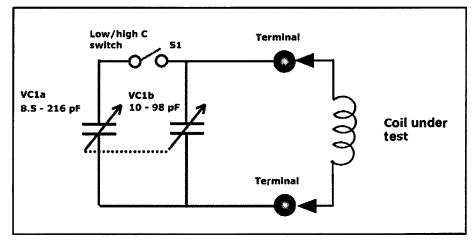
Figure 1: Circuit of the basic dip oscillator helper.
