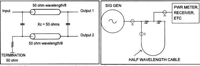
Figure 7: Eighth-wave quadrature network. Taken from Reference 2 which also gives a lumped component version for frequencies where coaxial cable is inconvenient. Reference 1 also has variations on the same theme, with cascaded versions offering guite wide bandwidths. In all cases the feed and
