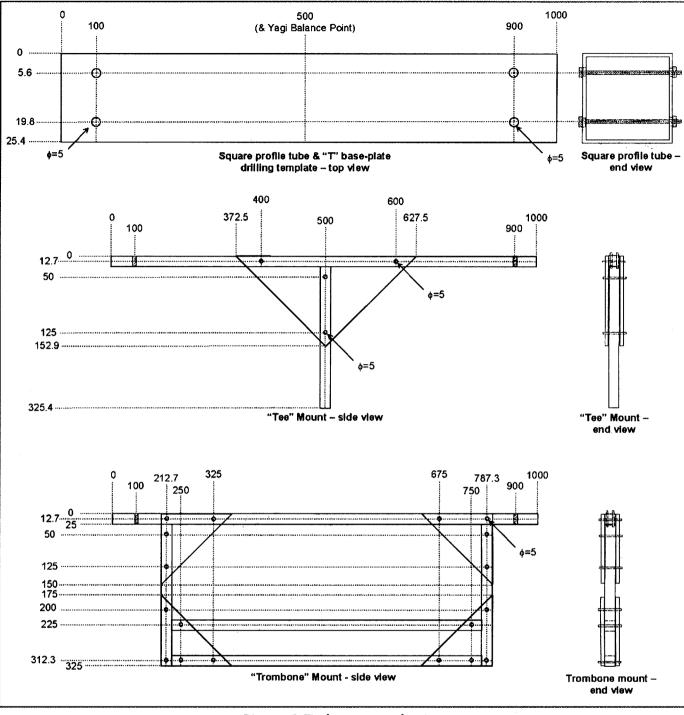
Diagram 5: The boom to mast bracket.
