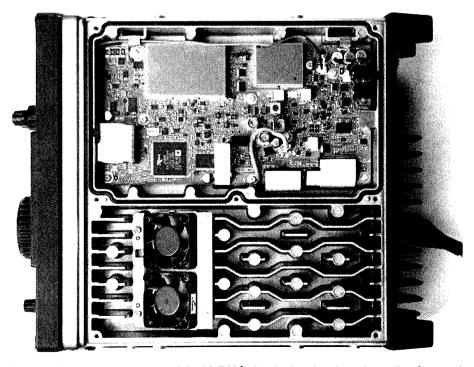
Photo 3: A view inside the top of the IC-7200 clearly showing the twin cooling fans and the extensive cooling fins and ducting.
