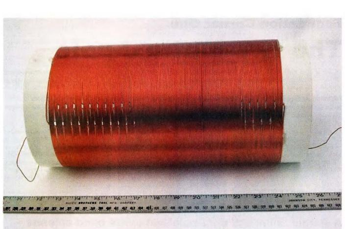
Photo 1: My antenna loading coil, wound with solid enamelled copper wire upon 160 mm diameter UVPC pipe.
