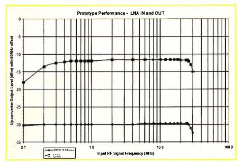
Figure 4: Up-converter frequency response - LNA in and out.
