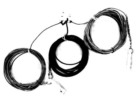
Photo 4: The portable 40 m dipole using homemade PVC insulators.
