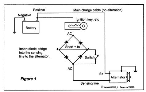
Figure 1: The circuit diagram of the automotive alternator booster.
