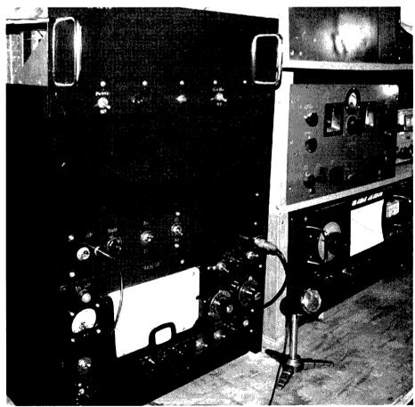
Photo 3: The restored HB10 is on the bottom right. To the left is the restored ex VK3AUL transmitter. The power supply is on the top, the modulator in the middle and the transmitter on the bottom.
