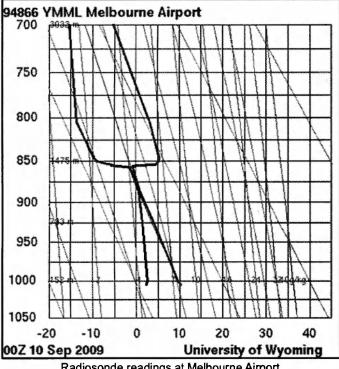
Radiosonde readings at Melbourne Airport
