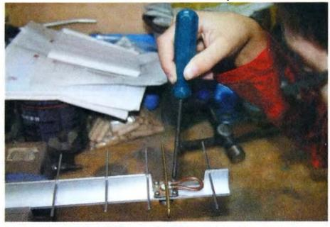
Photo 3: Fitting the Driven Element Assembly
