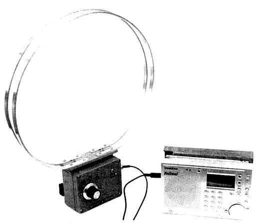
Photo 1: The active loop receiving antenna for 7 - 29 MHz in action.
