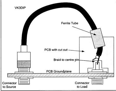
Figure 11: Reversed connections test.
