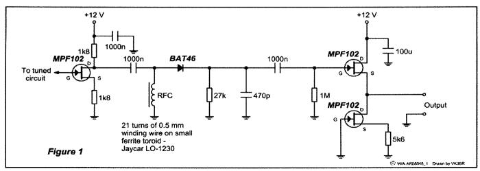
Figure 1: The circuit of the high quality AM detector.
