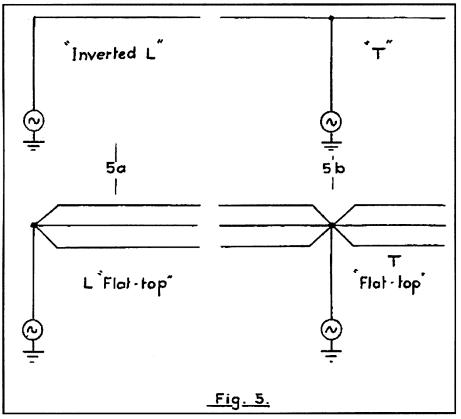
Figure 5: Two popular realistic 136 kHz antenna configurations.
