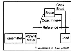
Figure 12: Reversed connections test equipment connections.
