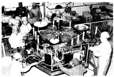
Figure 3: The technological foundations for the Mars mission was created by construction of earth satellite AO-40/P3D, launched n 2000 using an ARIANE 5 rocket.
