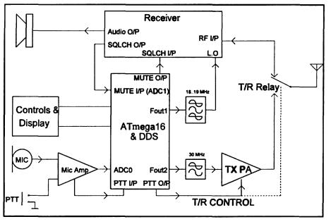
Figure 2: A block diagram of the transceiver.
