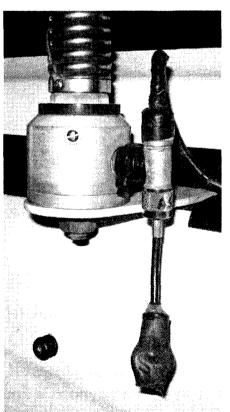
Photo 2: Matching capacitor connected via coax T-piece
