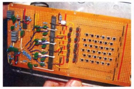
Figure 3: 35 PIN Photo-diode array.
