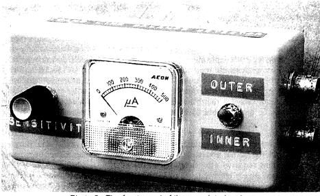
Photo 2: The front panel of the completed meter.
