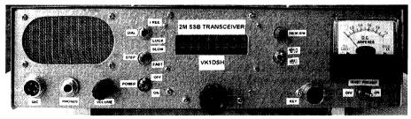
Figure 15: A view of the front panel. The DC ammeter provides useful information on the operation of the transmitter power amplifier; however it is not essential and can be deleted from the design if the constructor wishes.
