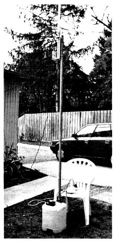
Photo 2: The plastic chair in place, allowing easy antenna tuning adjustments.
