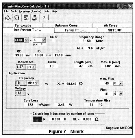
under "max. Flux", as the core could be driven into saturation.
