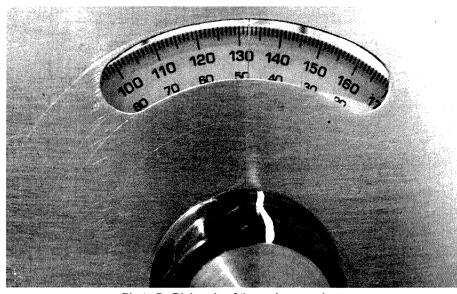
Photo 5: Dial scale of the varicap version.
