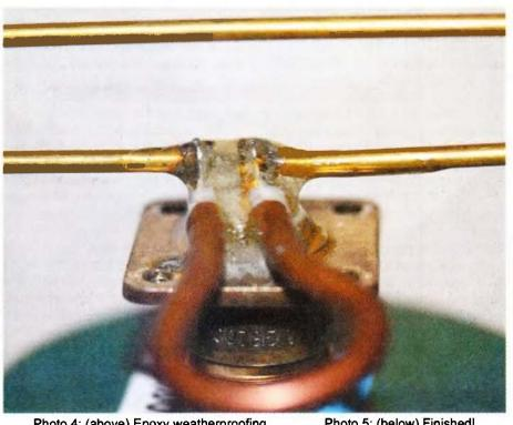
Photo 4: (above) Epoxy weatherproofing
