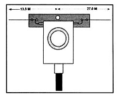
Figure 14: The antenna dimensions.
