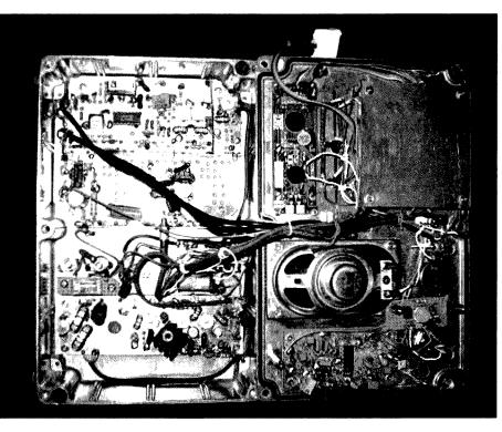
Figure 7: A look inside the 10 metre FM transceiver. The screen that usually covers the circuitry on the right hand side has been removed so that the general construction can be seen. The additional screen on the top right hand side covers the microcontroller and DDS circuitry and is required to reduce RFI from the high-speed digital circuitry. The white connector on the top right hand side is the in-situ programming input for the
