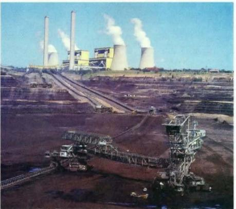
A view of one of the dredgers in the Loy Yang open cut mine, with the station in the background.The vehicles in the forground provide an indication of size. Photo courtesy of PowerWorks and Loy Yang Power.
