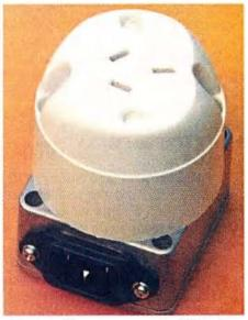
Photo 1: The final assembled IEC filter – mains adapter.
