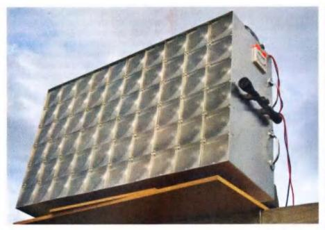
Figure 2: 60 Luxeon LED array with secondary Fresnel Lenses (photo courtesy of A de Quincey VK7NDQ).
