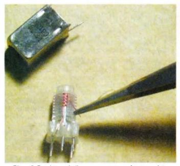
Photo 5: Break top winding to remove turns for new value.
