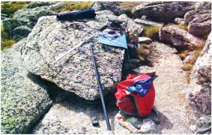
The portable set-up: antennas, radio, tuner, power and pack. Note especially, at about 5 o'clock in the photo, the power pack for the voice activated antenna rotator shown in the front cover picture.
