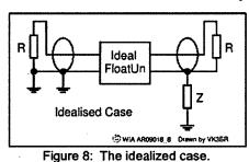
high compared to R so that the unwanted current becomes negligible, then our piece of coax can behave as an ideal float to unbalanced converter. The value of Z without adding anything else to the outer of the coax depends primarily on the length and configuration (that is, if it is coiled or straight) of the coax. Further, as seen above, a float can connect happily to a balanced so in fact a long enough piece of coax, especially if it is coiled, will work perfectly fine as a balun.
