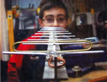
When you are happy with how the assembly looks and the quality of the solder joints, you can place the assembly on the boom, and bolt it down using the M3 bolts. Use either split or star washers, or a thread-lock liquid (such as Loctite®) to ensure the bolts don't work loose (See Photo 3).
