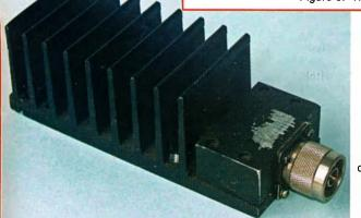
Figure 7: A dummy load, this one rescued from a decommissioned mobile phone base station transmitter. The VK5JST Antenna Analyser is an excellent home brew construction exercise for any club or individual.
