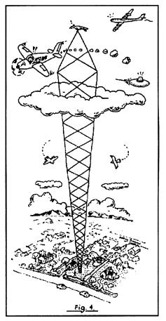
Figure 4: A full quarter wave at 136 kHz would be impractical.
