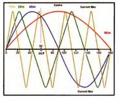
Figure 3: A visualisation of the impedance at different places on any antenna.
