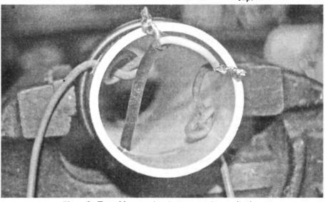
Photo 3: Top of former showing connection to dipoles.
