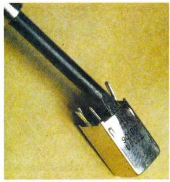
Photo 3: Raising the IF can dimples with a small screwdriver.
