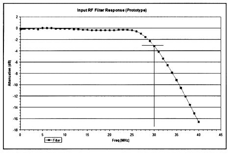
Figure 5: RF input LPF response (prototype).
