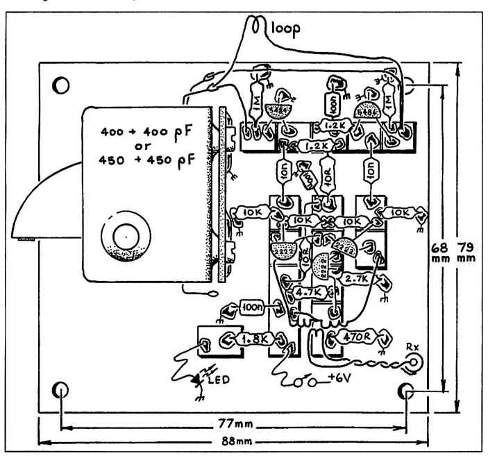
Figure 2: Suggested layout of the components on the 'paddyboard'.
