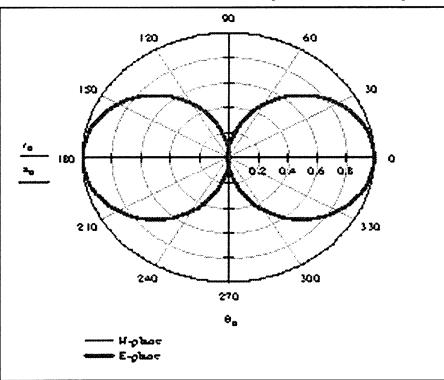
Magnetic loop field amplitude diagram
