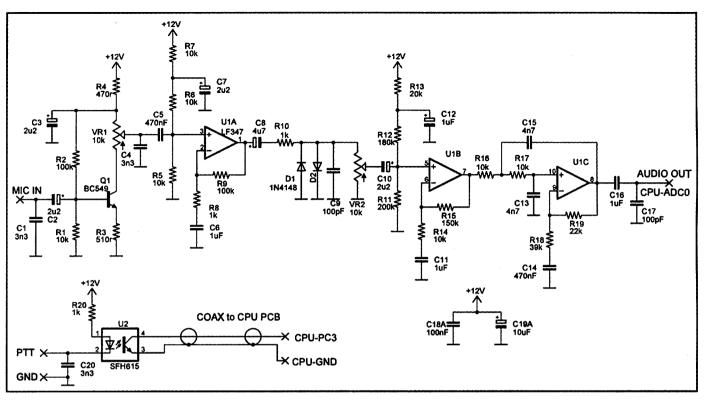
Figure 4: Microphone amplifier, audio processor and PTT circuit.
