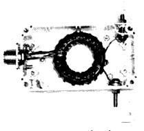
Figure 13: The mounted 4:1 balun – consider using eye bolts instead of the backing board.
