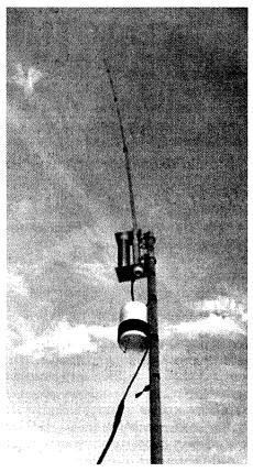
Photo 3: The Stationmaster, converted for 40 metre operation, 'in the air'.
