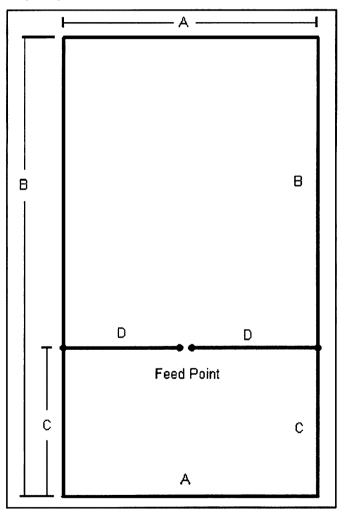
Figure 1: The electrical diagram of the 'Hentenna'.
