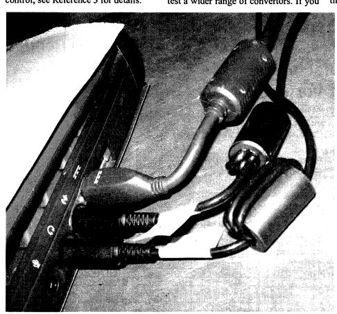
Figure 5: A view of the ferrite chokes and external PC screening.
