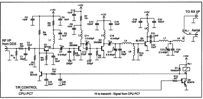
Figure 5: Transmitter power amplifier circuit.
