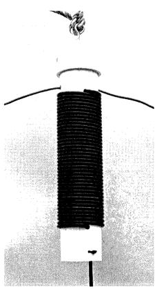
Photo 6: Completed balun up in the air.
