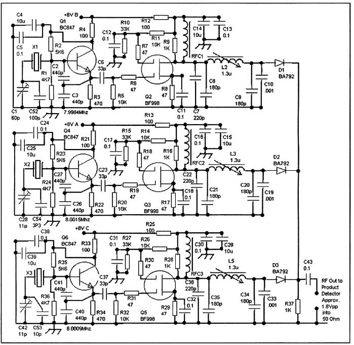
Figure 2: Circuit of the crystal oscillators.
