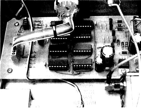
Figure 6: Photo of the assembled attenuator control board.
