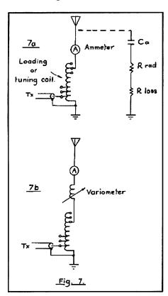
Figure 7: Examples of some typical antenna circuit loading arrangements.
