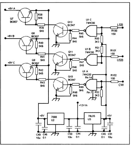
Figure 1: Circuit for BFO module.
