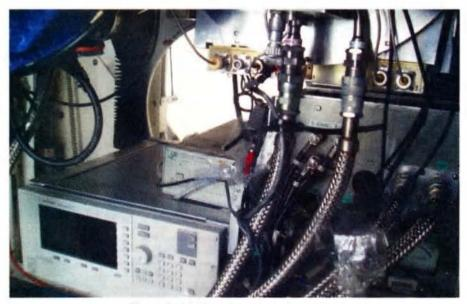
Figure 2: Liquid helium cooled receivers.
