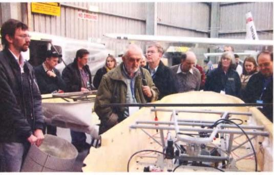
In the development area at Gippsland Aeronautics, Aeronautical Engineer Ed O'Brien explains how the team are developing new applications using a belly pod that fits beneath the GA-8 Airvan.
