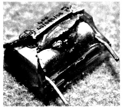
Photo 1 Front view of the faulty cap (you can just make out the brand name (RIFA).
