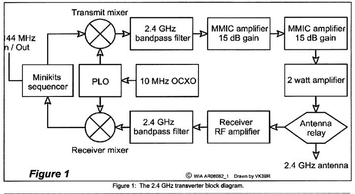
The key to the frequency conversion is the local oscillator signal, provided by a PLO producing a 2256 MHz signal for both mixers. This device is guite small, measuring about 25 mm by 15 mm and produces a signal that is proportionally as stable as the 10 MHz reference signal from the OCXO.
