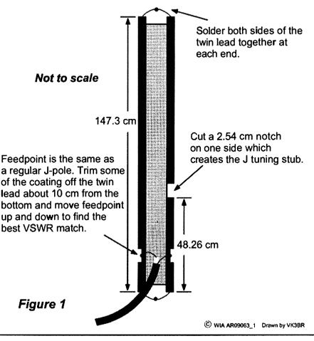
Figure 1: Diagram of the Slim Jim constructed from TV twin lead.
