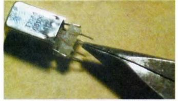
Photo 4: Removing coil former with unused pins.
