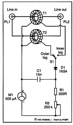
Figure 1: The circuit diagram of the balance meter.
