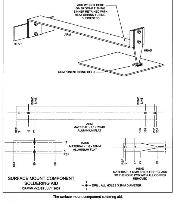
from standard 1.6 x 20 mm aluminium flat section which can be purchased conveniently at your nearest hardware store, and 1.6 mm thick PCB from which all copper has been removed.
