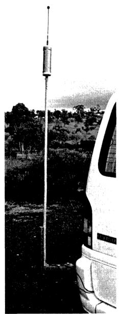
Photo 1: The top loaded antenna deployed
