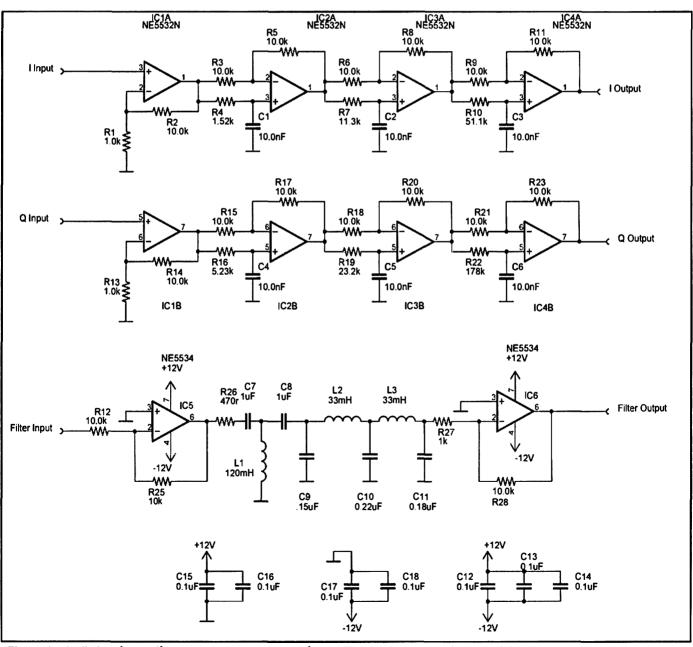
Figure 3: Audio band pass filter and quadrature network board. The connections to the I and Q inputs and outputs depends upon the mode of operation. The inductors are small PCB mounted units, see supplier information.
