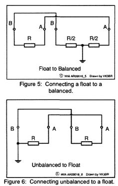
is no longer shorted out so matching is fine and while we are not reinforcing the balance of the load we are also not doing anything to distort it, so our ideal dipole can stay ideal. So connecting a float to a balanced is also OK. Similarly, Figure 6 shows the float to unbalanced case.
