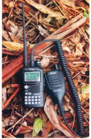
Photo 2: The IC-92AD and optional HM-175GPS displaying the current position using the GPS-A function. No need to worry about dampness or rain drops with this radio, rated waterproof to 1 m depth for up to 30 minutes.
