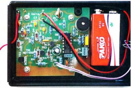
Photo 1: Completed PCB in the case with battery.
