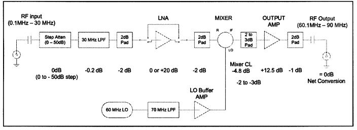
Figure 1: Block diagram of the up-converter.
