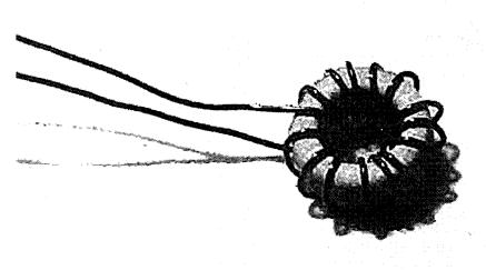
Photo 1: The toroid core used in the circuit.
