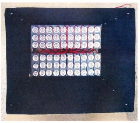
Figure 1: 60 Luxeon LED array with torch lenses.
