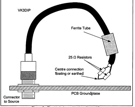
Figure 9: Float to balanced test on the test jig.
