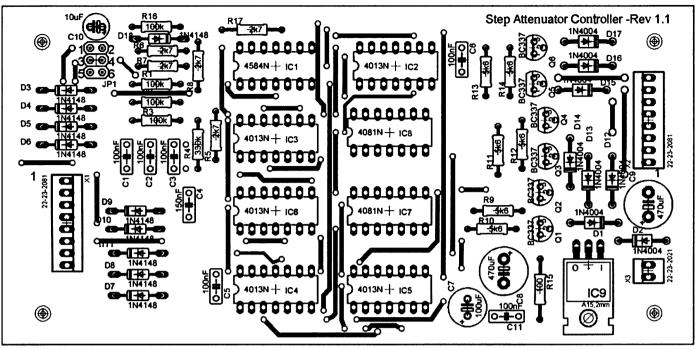
Figure 4: Top overlay showing components and wire jumpers.
