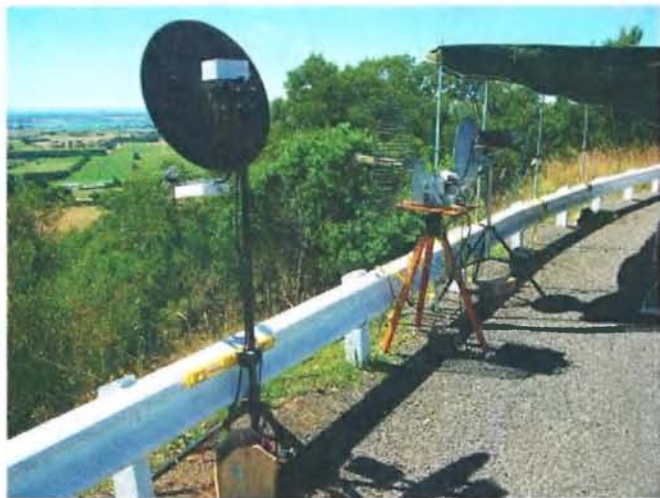
VK3ATL: Microwave dishes (L to R) 10 GHz, 2.4 GHz and 5.7 GHz.
