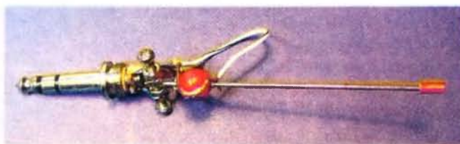
Photo 1: The 6.3 mm stereo plug single paddle lever.
