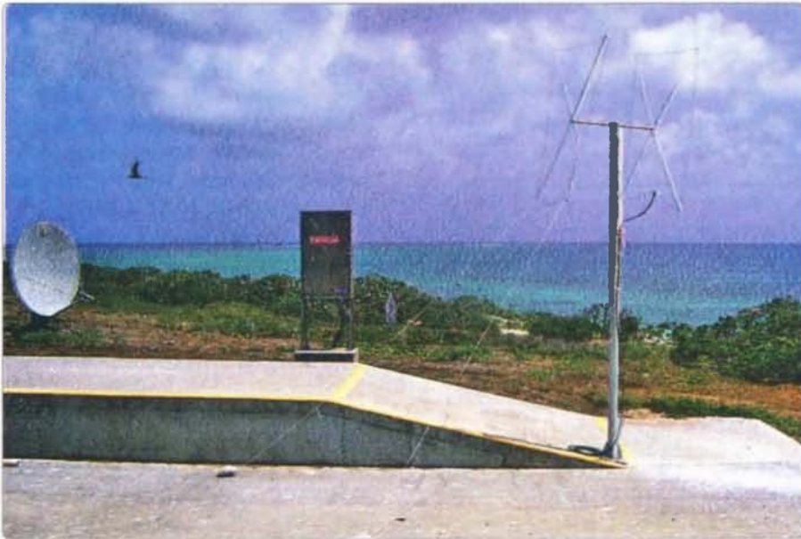
Photo 4: The six metre beam with the unique coral block rotator system. The dish in the background is for digital satcomms.
