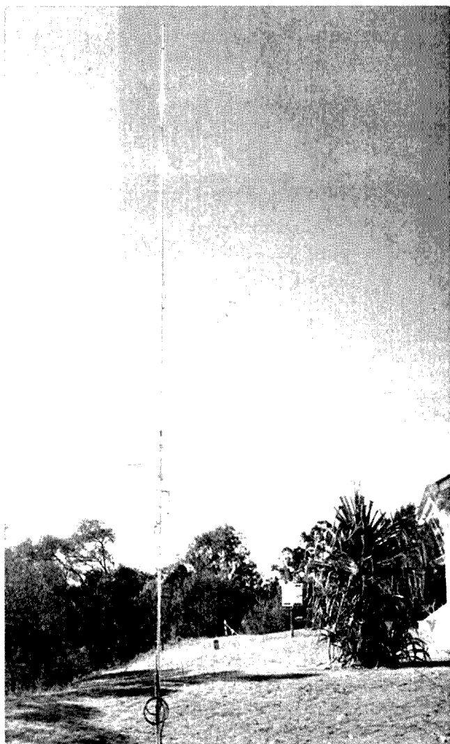
Photo 3: The Butternut HF6V. Our magic antenna for the weekend with ground radials for 10, 15, 20, 40 and 80 m (20 ground radials in total).
