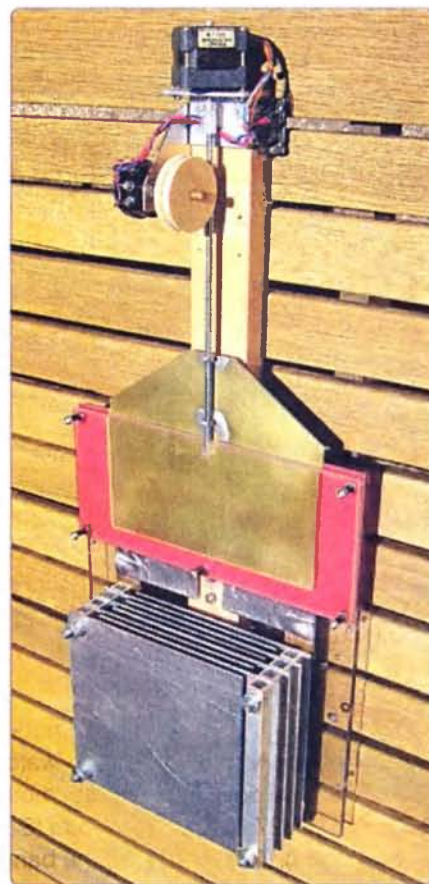
Photo 2: The tuning capacitor and feedback potentiometer assembly.
