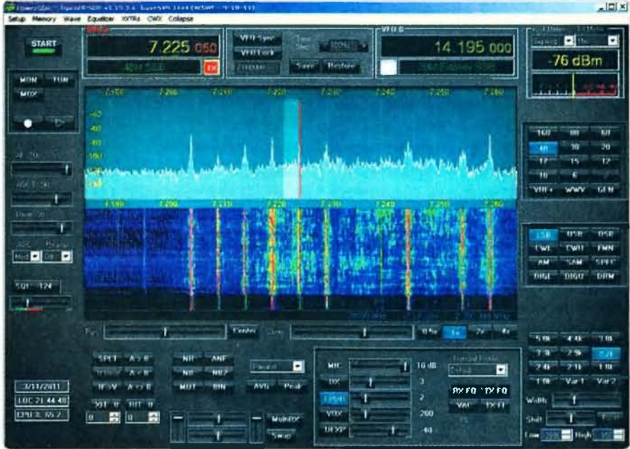
A screen shot of the PowerSDR/OpenHPSDR software in operation. Instead of touch buttons and knobs, controls are mouse click buttons and sliders. You also have panadapter waterfall displays, together with a "S meter" calibrated in dBm, not rubbery "S" units.
