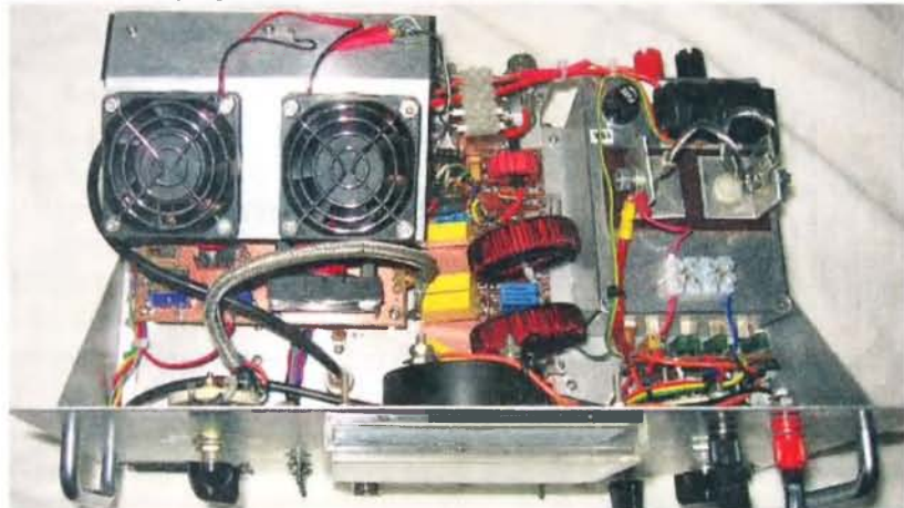
Figure 11: Top view showing (from left to right): the power amplifier module (beneath the fans), low-pass filter and meter circuit and power supply box. The fans are only necessary if running at full power for an extended period of time. Otherwise they are optional. The home-made current shunt can be seen on the top right-hand side of the picture.
