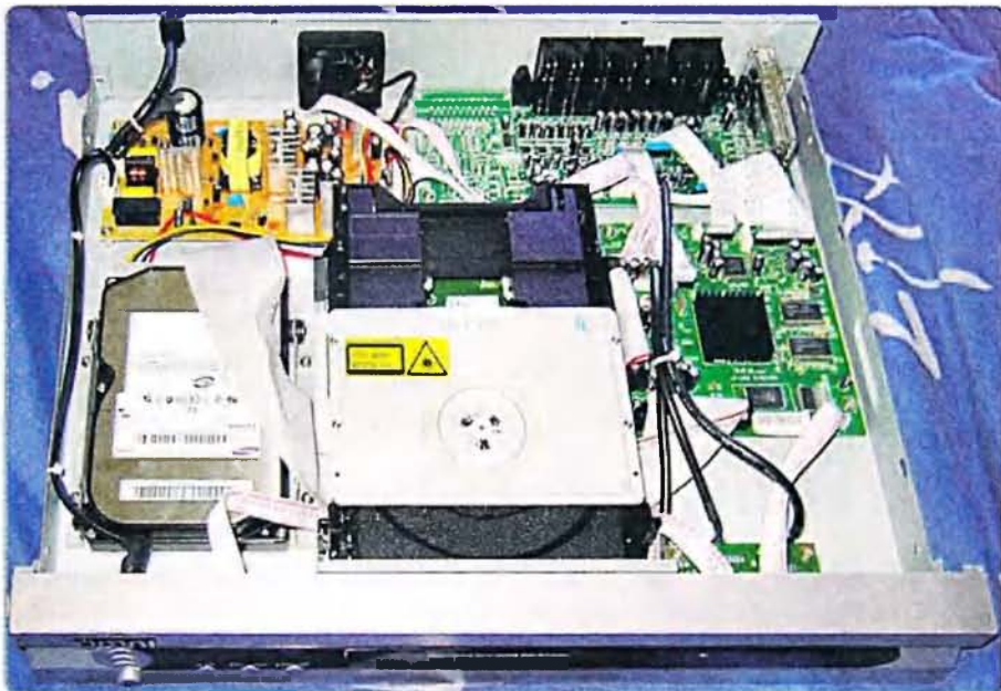
Photo 2: The power supply is clearly visible once the lid is removed.
