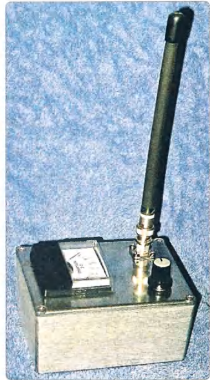
Photo 3: The completed field strength meter, antenna attached, ready for use.
