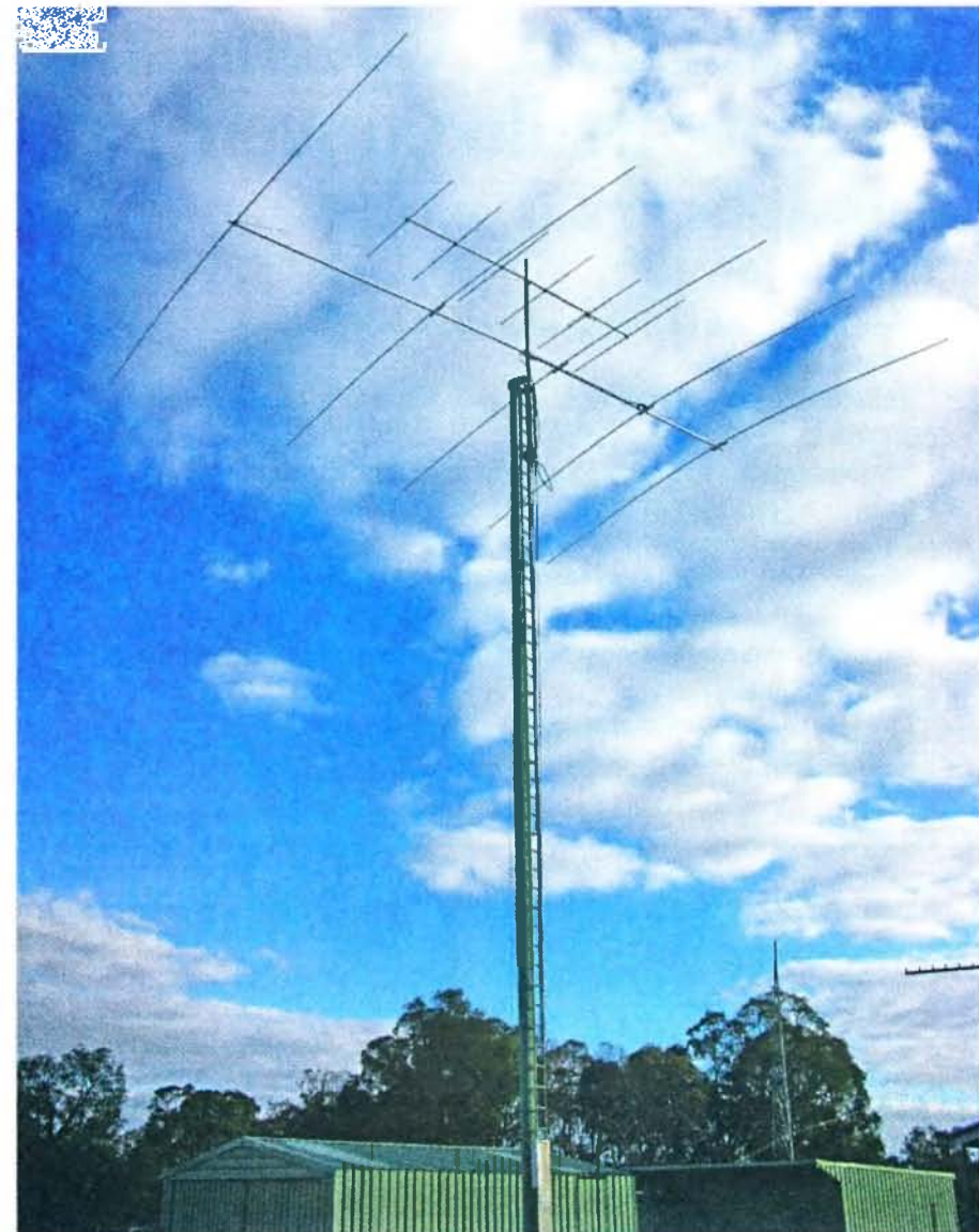
Photo 1: The new 20 metre beam.
