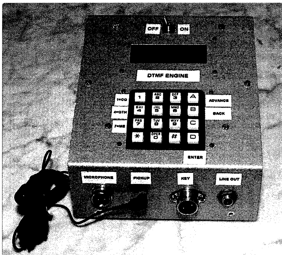
Figure 1: The DTMF engine with optional pick-up microphone. Connections to the radio and 12 VDC are on the back of the unit and operator connections (microphone and key) are on the front. The prototype unit was built into a small home-made enclosure that could sit adjacent to the transceiver.
