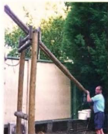
Photo 4: A view of the counterbalance, actually two buckets of sand.
