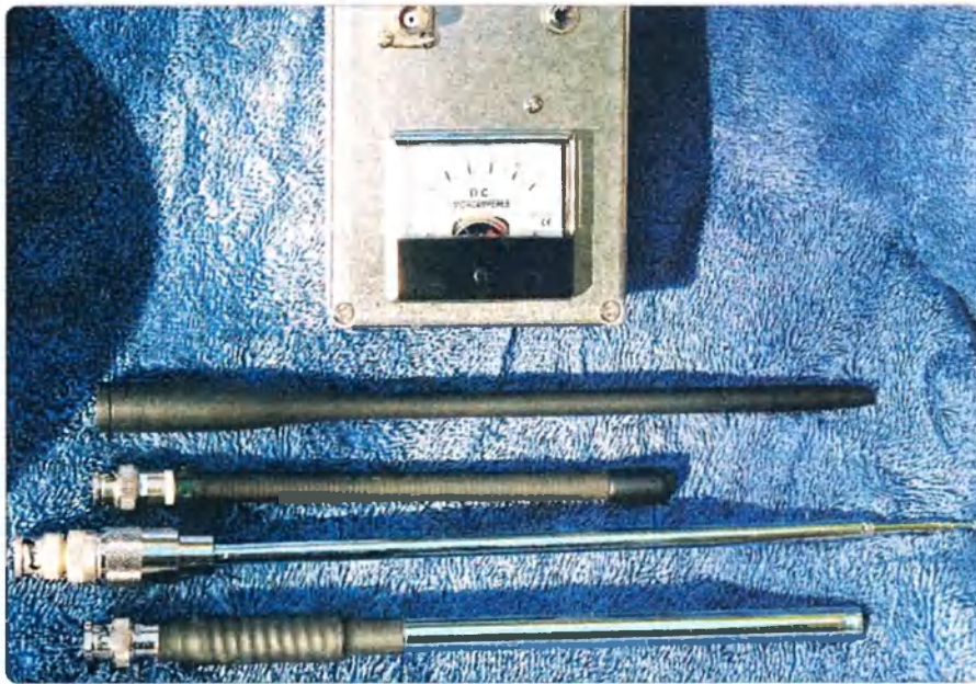
Photo 2: A selection of potential antennas for use with the field strength meter.
