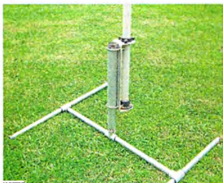
Photo 3: The antenna base with the Hidaka vertical fitted to the base using a slightly larger piece of pipe.
