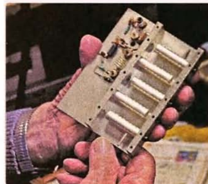
A 23 cm receive converter, entirely built and silver plated by Wally VK6WG.
