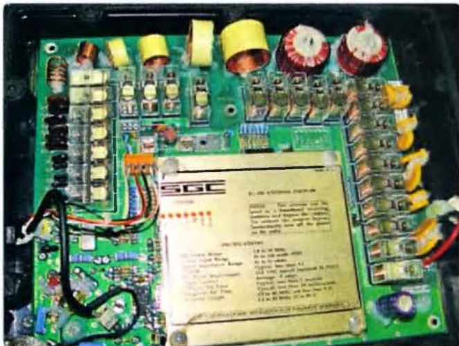
Photo 2: The board of the auto tuner, detailing specifications.
