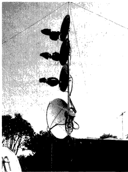
Photo 2: The VK3ER/p array of offset dishes for microwave operation.
