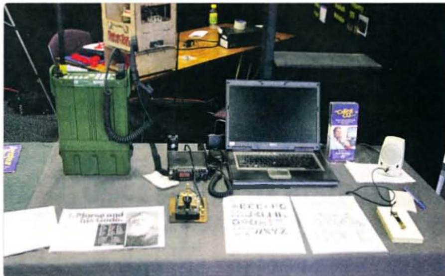
Photo 1: Booth display – Codan HF manpack, Yaesu FT-817, Morse keys, documentation and laptop for decoding the Morse transmissions.
