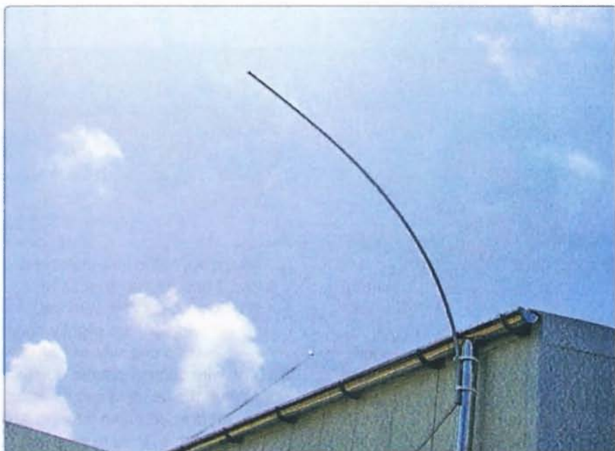
Photo 3: The six metre Slim Jim and part of the HF longwire in the background.
