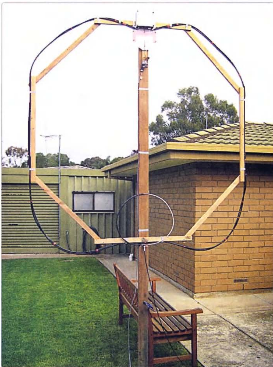
Photo 1: Testing the loop on a temporary frame.
