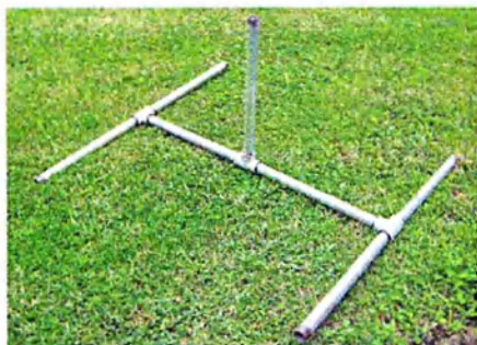
Photo 2: The antenna base assembled with all legs screwed in place.
