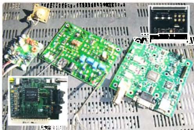
Photo 1: Some of what is available on the SDR market today. L to R: SoftRock, Mercury (bottom left), SDRZero, RFSPACE SDR-IQ and Flex 5K (top right). The photo was sourced from the Internet and enhanced.
