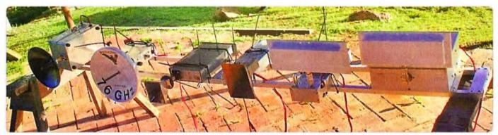
Photo 1: Six transverters on a mounting frame with 2.4 GHz on the left, through to 47 GHz.
