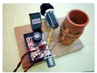
Photo 6: The completed 'Blob Board 500 mW CW transmitter'.
