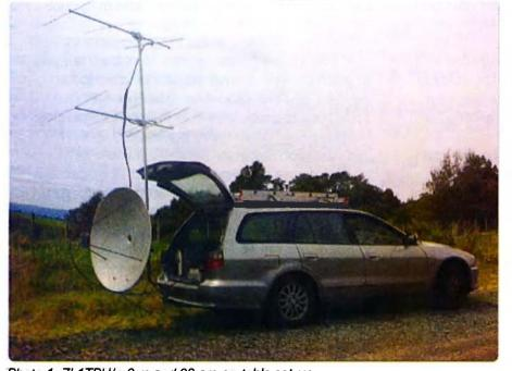
Photo 1: ZL1TPH/p 2 m and 23 cm portable set-up.
