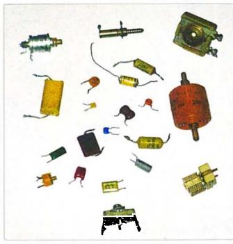
Photo 3: Various fixed and trimmer capacitors.
