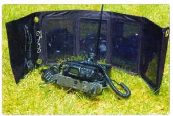
The Goal0 Sherpa Adventure Kit (50 Watt-Hours lithium ion battery with 13.5 watt mono-crystalline folding solar panel)) powering an FT-817 in the field. The antenna attached to the rear is a Miracle Whip by Miracle Antenna, tuned for two metre operation. The battery and radio are strapped together making for a sturdy and highly compact ultra-light QRP station that can literally travel anywhere.
