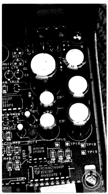
Photo 2: Sequencer power supply capacitor filters.
