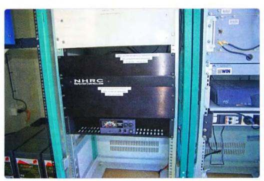
Photo 3: The two metre repeater, controller, APRS digipeater and power supply.
