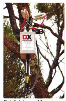
Photo 2: A close up of the vee beam feedpoint.
