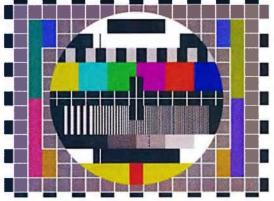
Photo 4: Philips PM5544 electronic test card.
