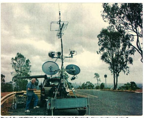
Photo 5: Roy VK4ZQ/4's 'loaded' mast partly elevated. Electrically-driven elevation and azimuth.
