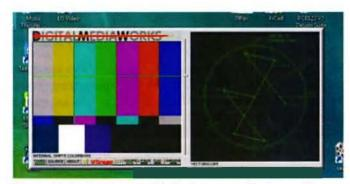
Photo 12: Colour bars in the Vectorscope display mode.
