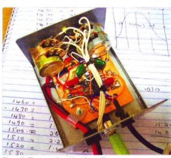
Photo 1: The completed bandpass filter.
