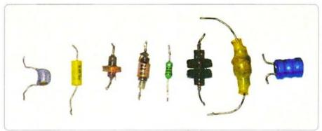
Photo 4: Various inductors and RF chokes.
