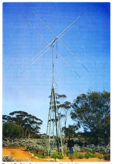
Photo 1: The Cubex Quad antenna on top of the windmill tower.
