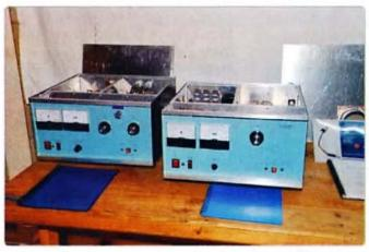
Photo 1: Two high power amplifiers from Bob VK3ZL. On the left is a full power water cooled amplifier for 20, 15 and 10 while on the right a legal limit amplifier for two metres.
