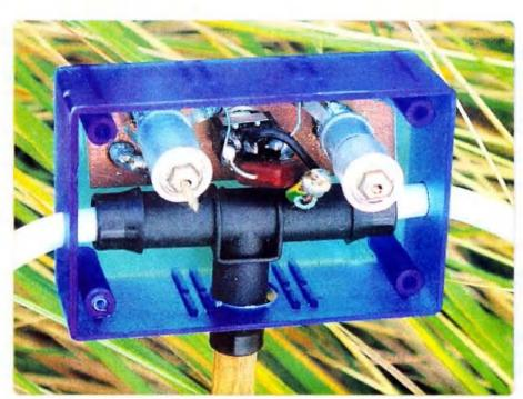
Photo 3: A close up of the capacitor box.
