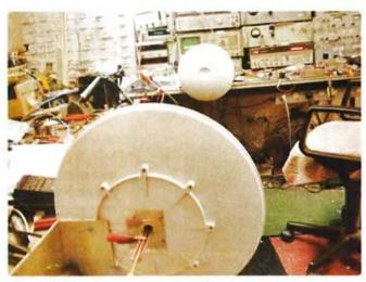
Figure 2: The Cassegrain dishes during early testing.
