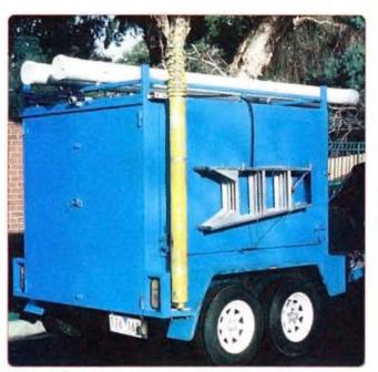
Photo 2: Rear view showing the Clark pneumatic mast.
