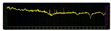
Figure 3: 20 m ground plane with L-Match tuned to 12 m band.
