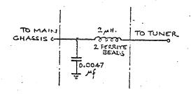
Filtering the leads in this way produced a marked reduction in L.O.R., by about 15dB.
