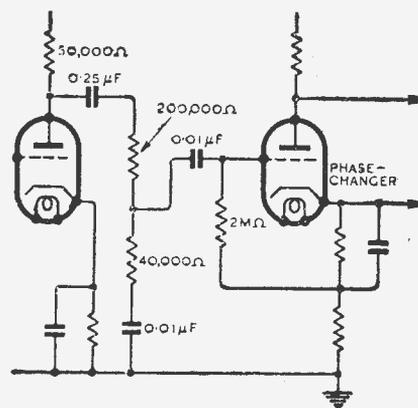
Figure 2.: The suggested correction circuit, designed for English valves, but readily adaptable for our types.
