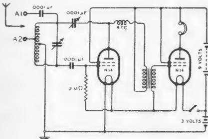
Suggested circuit diagram for two-valve headphone set to use a very low high-tension voltage. The valves are both of the "beam power" output type.
