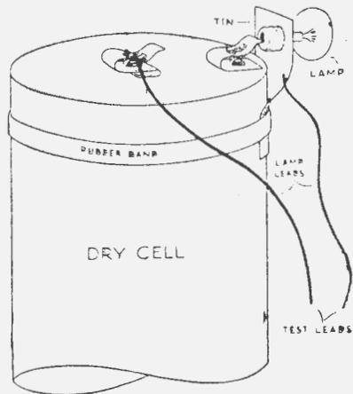
A drawing of the simple test equipment.
