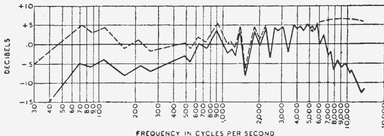
Figure 1.: The heavy line shows the response of the author's loud-speaker before correction, and the dotted line the approximate curve after correction.
