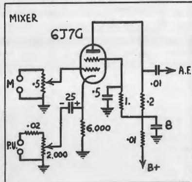
In any amplifier a mixing circuit can be obtained by feeding the pick-up into the cathode circuit.
