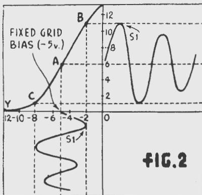
applied to the control grid, which has been given a bias of -5 volts (see fig. 2.). The first peak of the curve ("S1") has a peak value of 3 volts, and so reduces the bias to -2 volts, taking the operating point of the valve from "A" to "B". The succeeding half-cycle swings the operating point in the opposite direction, to "C." In other words, the application of the signal has caused the bias to vary from its normal figure of -5 volts to first -2 volts and then -8 volts.
