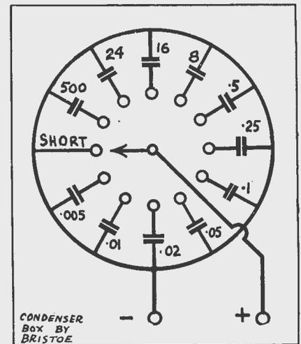
switch is the master switch, which is used to connect whichever one of these switch deck is required to the terminals.
