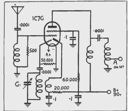
Circuit of the short-wave converter suitable for fitting to any battery set.
