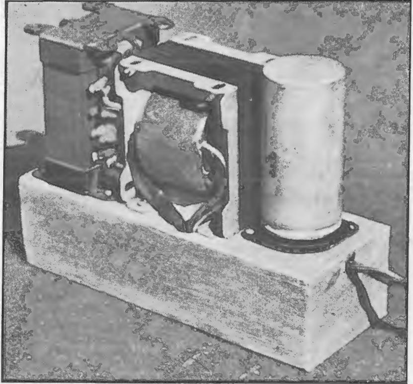
Photograph of the vibrator power unit, made up from parts still readily available.
