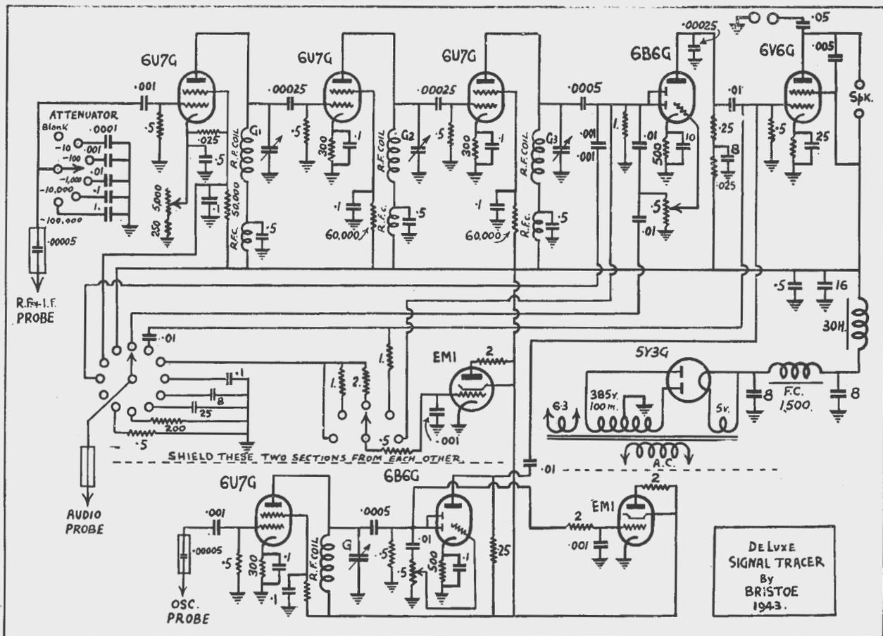
Circuit schematic of the latest version of the Signal Tracer.
