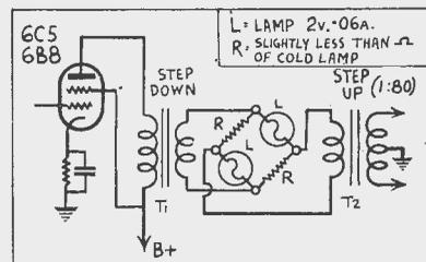
A pilot light bridge arrangement for automatic volume expansion.
