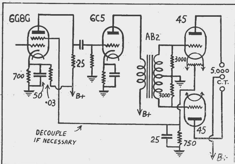
Circuit for automatic volume expansion, taking the screen voltage from the bias resistor of the output valves.
