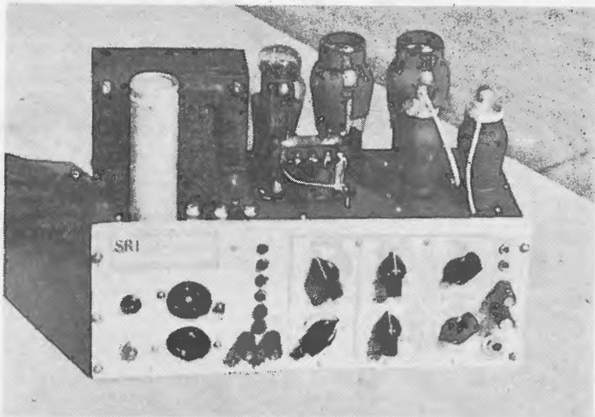
The finished amplifier, built on to a deep base with control panel in front
