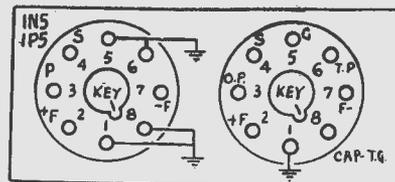
Diagram of the socket connections; left, the 1N5 and 1P5; and, right, for the 1D8GT.
