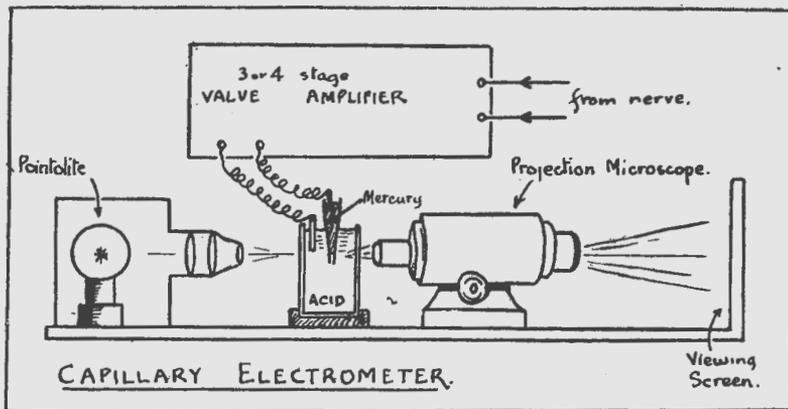
Figure 4. The capillary electrometer for recording minute electrical impulses.
