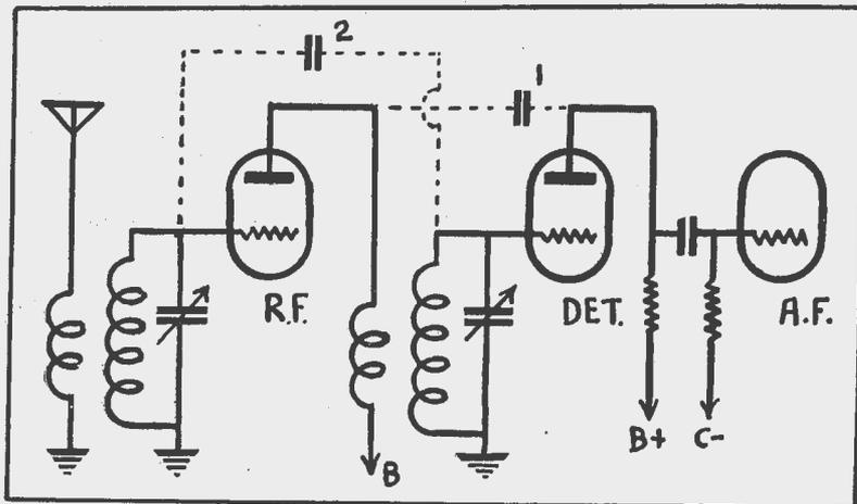
Diagram to indicate where capacity can introduce regeneration.
