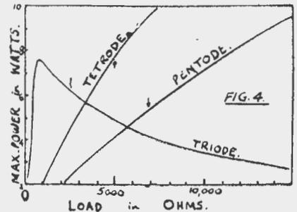
Fig. 4, showing effect of load on output.
