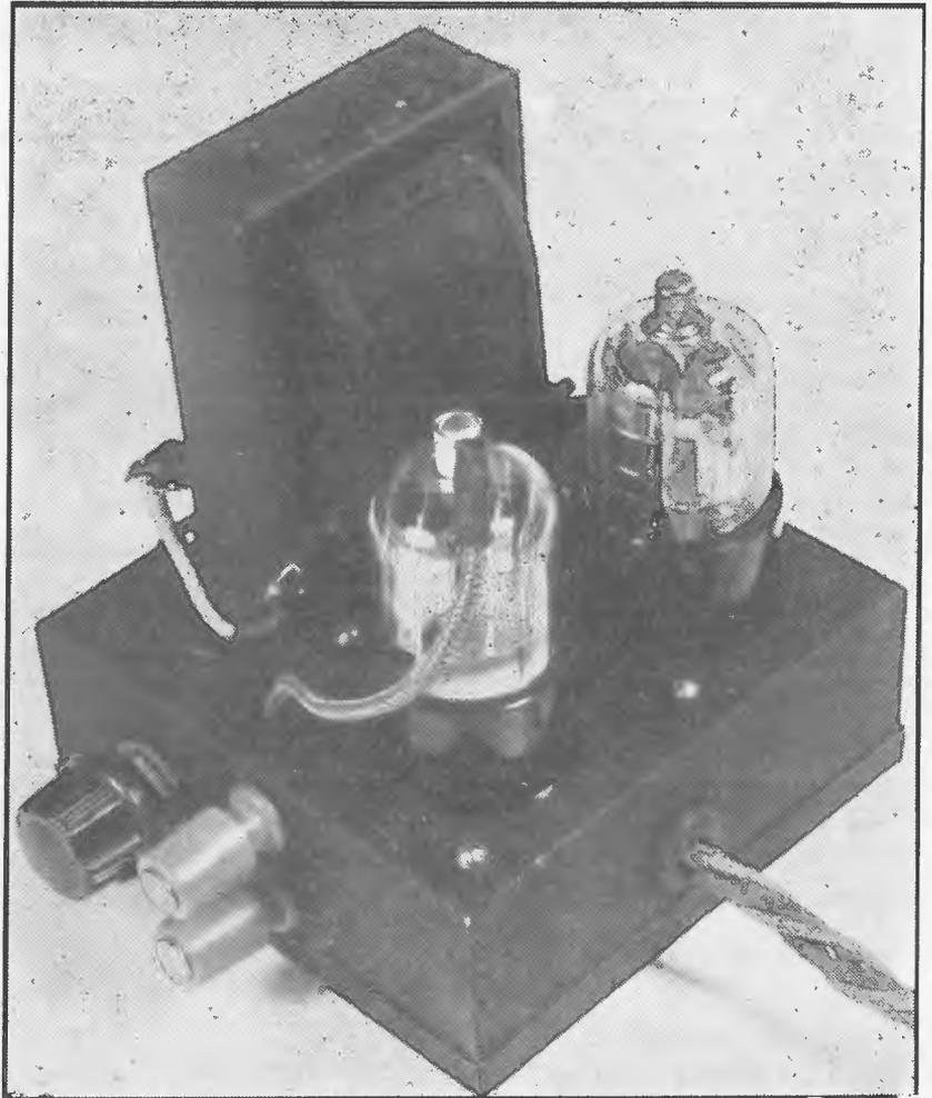
A photograph of the unique little battery-operated amplifier, which uses only two output pentodes.
