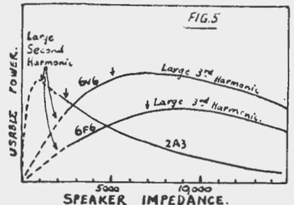
Fig. 5, showing effect of load on usable power.
