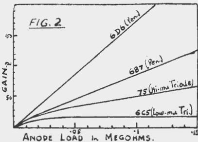
Fig. 2, showing effect of load on gain.
