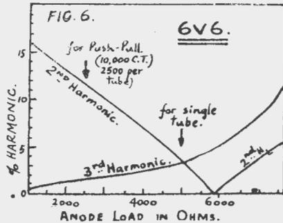
Fig. 6, showing effect of load on harmonic distortion.
