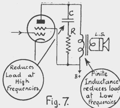
Fig. 7. Output Circuit to prevent rise of Load at Low and High Frequencies.
