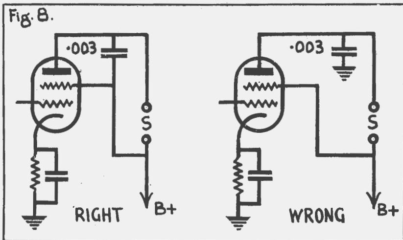
In order to avoid possibility of breakdowns, condensers should be fitted across lowest permissible potential.
