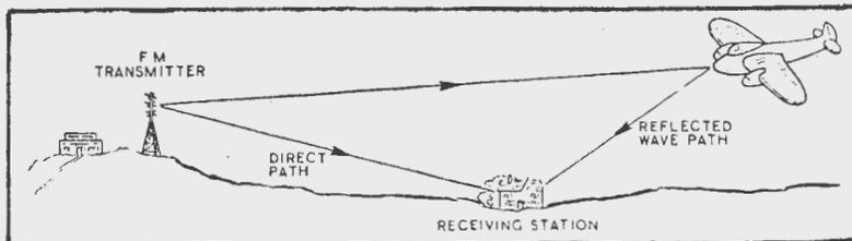
Frequency modulation can be affected by reflections, as from a moving aircraft overhead.
