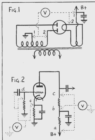
plied anode voltage is, peculiarly enough, by measuring the anode current by means of a milliammeter. If this were inserted at the point marked c, the current consumed by the valve could easily be found (provided that the resistance of the meter were not high by comparison with that of the anode-circuit load). By comparing the current with that shown on the curves for the particular valve in use it would be possible to obtain a fairly accurate indication of the actual plate voltage.
