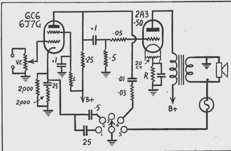
Circuit for use when a pentode valve is used in the first stage.
