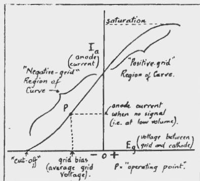
positive. If the signal voltage exceeds the grid bias voltage, then the grid will become positive at one end of the swing and because a positive body attracts electrons, grid current will flow at these times. To indicate that grid current flows, the figure 2 is used. Note:—In the case of class AB operation, the valves may be class AB1 for medium-sized signals, and
