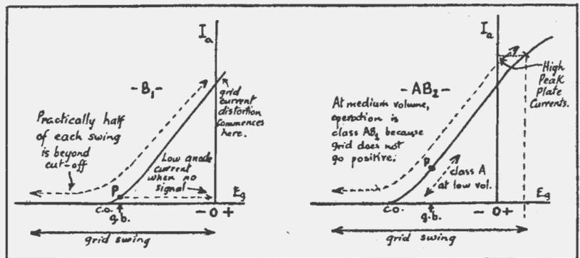
Typical grid-plate curves of output valves to illustrate the different classes of operation.
