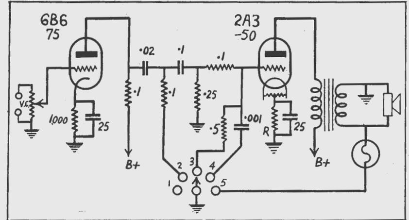
Circuit for use with a triode valve in first stage.
