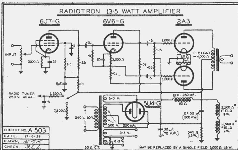
Circuit of the Radiotron circuit A503, which was originally released in 1939. Since that time it has proved itself to be a particularly effective and handy circuit.
