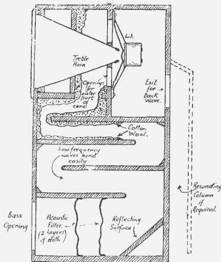
FOLDED HORN WITH TWO ACOUSTIC CHANNELS.
