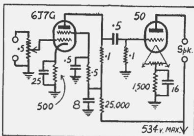
A suggested circuit, with a large power triode driven by a pentode first-audio valve.
