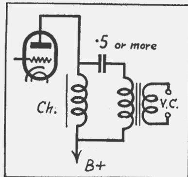
Schematic to show shunt-feed arrangement to improve efficiency of the output transformer.
