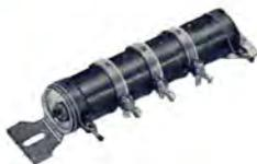
Voltage dividers are available in two sizes—15,000 ohms and 25,000 ohms. They are fitted with 2 fixed clips, 3 adjustable clips, and 2 strong mounting brackets. Like the resistors, all dividers are finished with green insulating lacquer. Careful selection of metal and a patent clip makes adjustment and soldering a quick and simple matter.
