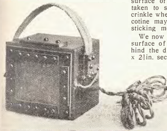
Finished view of the original microphone. The job is built for portability and will stand rough handling. A protective mesh is used to prevent damage to the mica diaphragm.
