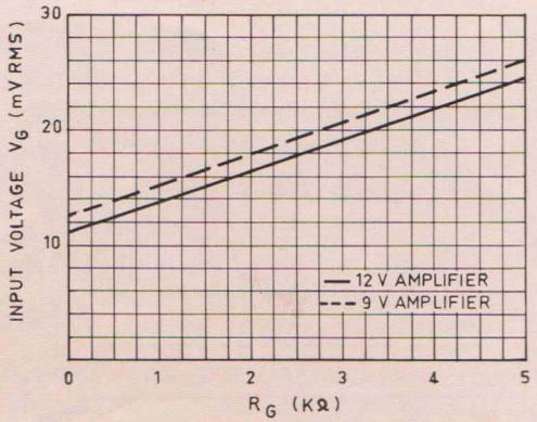
Fig. 4. Sensitivity for maximum power output.
