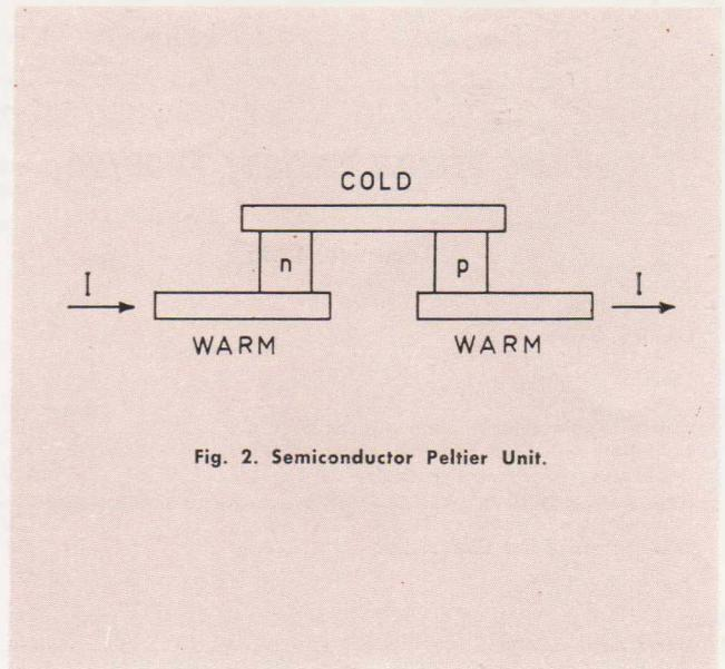
Fig. 2. Semiconductor Peltier Unit.
