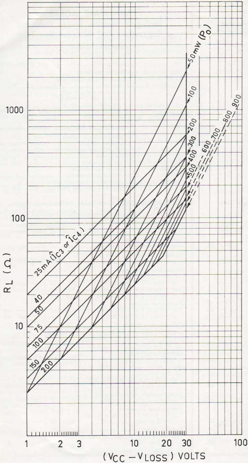
Fig. 6. Initial Design Nomograph.
