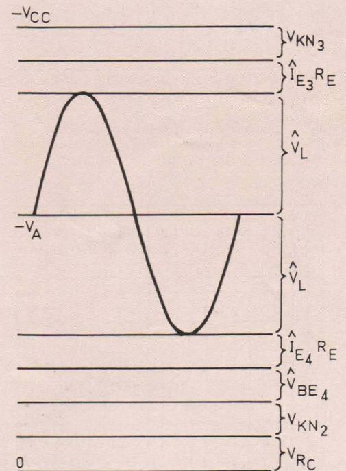
Fig. 2 (b). Dynamic operation about operating point A.
