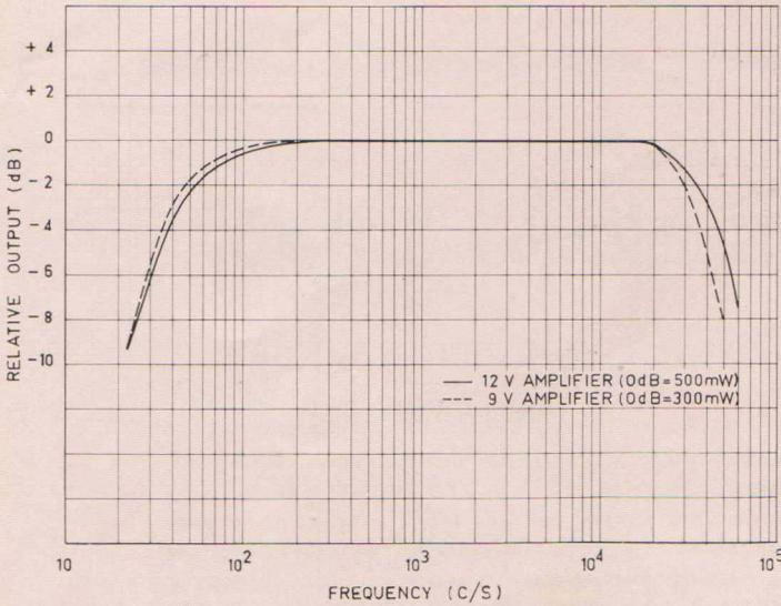
Fig. 3. Frequency response at maximum power output.
