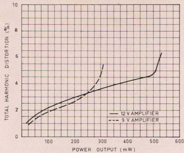
Fig. 5. Distortion characteristics at 1 Kc/s.
