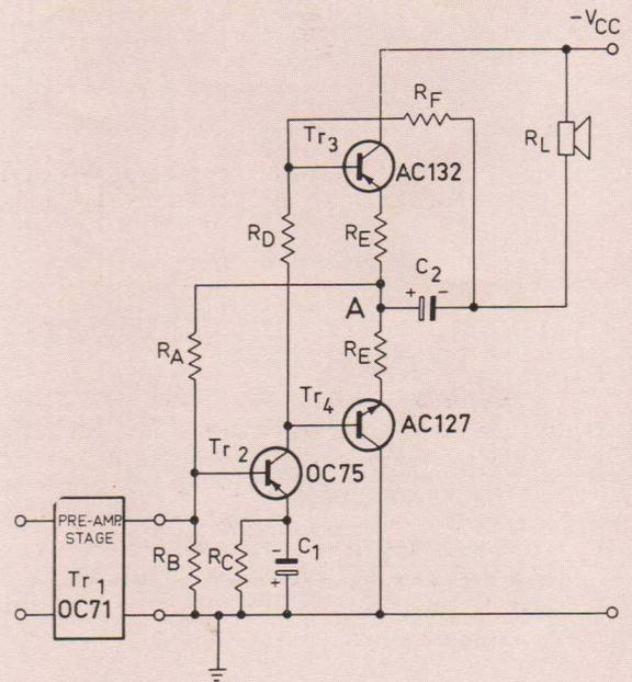
Fig. 2 (a). Basic complementary-symmetry amplifier.
