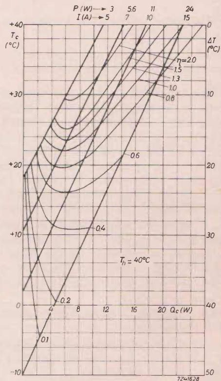
Fig. 4. Cooling capacity and current versus temperature, measured for hot-side temperatures ( $T_h$ ) as indicated.
