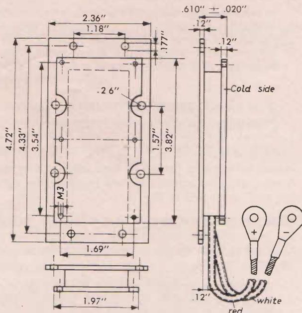
Fig. 3. Dimensional drawing of Peltier battery PT 20/20. (The length of the terminals, including mounting tags, is 9½ ins.).
