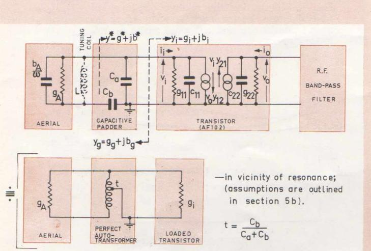
Fig. 5.—Derivation of simplified equivalent circuit, useful for estimating VSWR and source conductance, for mast-head units described.
