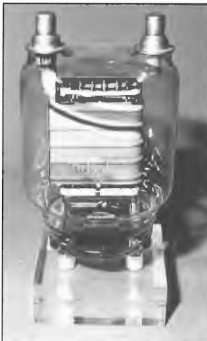
The Radiotron 833/833A valve was one of the most widely employed valves in AWA transmitters for many years going back to the late 1930s. The valve was a power triode with all four terminals protruding out of a specially designed envelope. For Class C telephony it provided a power output up to 630 watts. This valve was used in the 3CS transmitter installed in 1952 by Chief Engineer, Roy Streeter.
