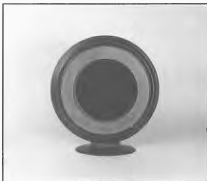
13. Rola Cone Recreator, 1926. Made by Rola Co., USA. Magnetic cone type and supplied with matching transformer. Hardwood baffle disc and cast base.
