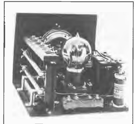
working into a 200 ohm load. Power for the valve was provided by batteries. At some studios this comprised 6 volt accumulators for filament and 130 volt battery system for anode and the microphone polarising voltage.
