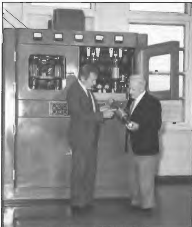
Bob Barrett (left) Broadcasting Operations Manager and Wally Clair examining 4279Z valve of the STC 2 kW HF transmitter VLI at Liverpool. The service was commissioned in December 1948 and transmitted ABC programs to outback New South Wales until it was closed down in October 1983. The centre also housed the 2FC and 2BL transmitters. Wally worked at the centre during the period 1938-71.
