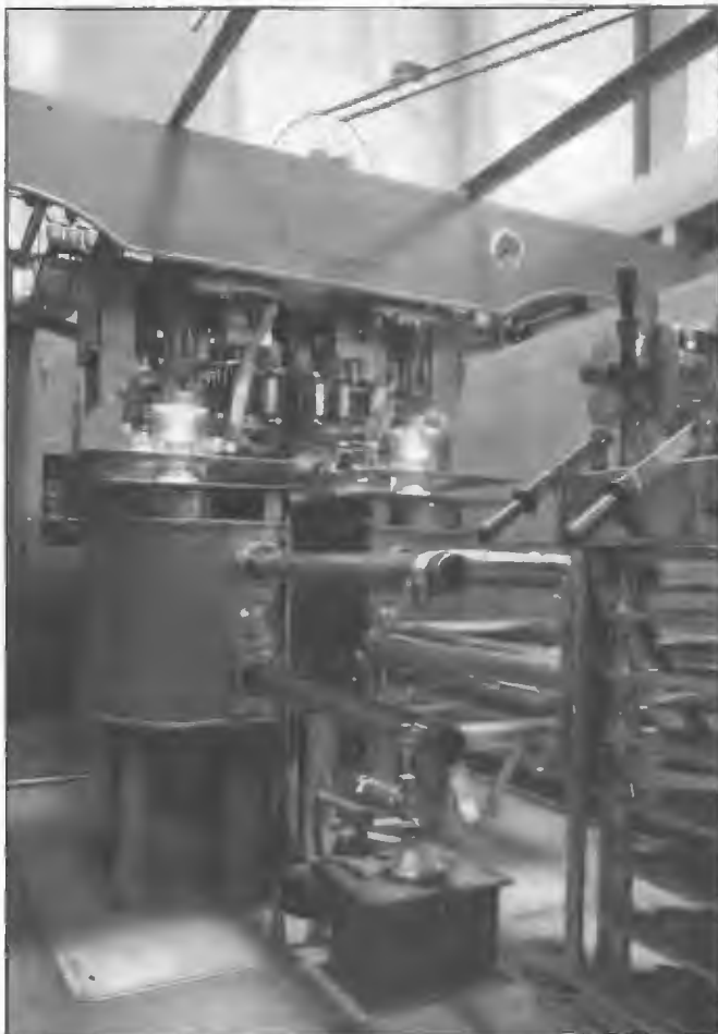
Federal/ITT power triode transmitting valve type F124A used in the power amplifier stage of the two original 100 kW transmitters at Radio Australia, Shepparton in 1945. Each transmitter used four F124A valves in push-pull parallel configuration. The filament of these water cooled valves was pure tungsten and valves had an average life of 6500 hours of operation. Commissioning Engineer, Tony Brettingham-Moore.
