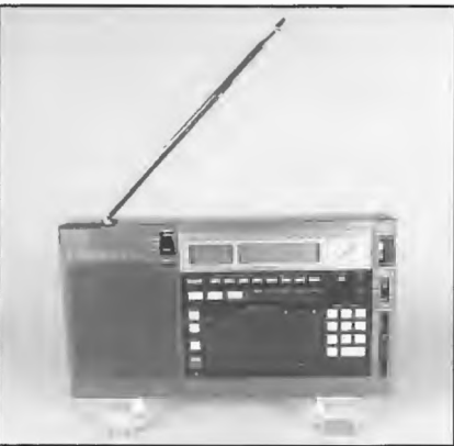
Typical high performance modern receiver. This Sony ICF2000D receiver purchased in 1985, employed a quartz controlled phase locked loop (PLL) synthesiser system with a microcomputer for pin-point tuning. It gave a choice of direct, manual, scan, memory or memory scan tuning. Up to 32 stations could be memorised for instant tuning at the press of a button. It operated from three dry cell batteries.
