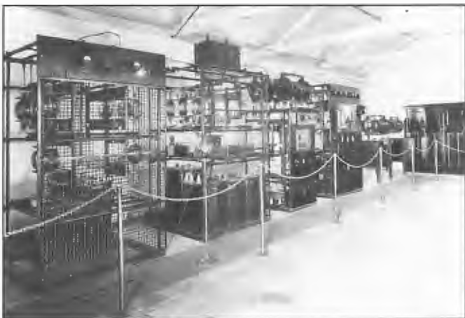
One of the 5000 watt transmitters designed and manufactured by AWA for A Class stations 2FC, 3LO, 5CL and 6WF commissioned during the period 1923 to 1925. Stations 2FC, 3LO and 6WF operated on long wavelengths while the others operated on medium wavelengths. The installation comprised six main units and the transmitter required a power supply of 15 kW. Senior AWA Engineers associated with design and manufacture included Joe Reed and Chief Engineer Arthur McDonald.
