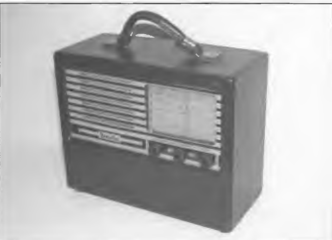
Five valve battery-powered portable receiver manufactured by Breville Radio Pty Ltd, 1946. It featured 5 inch permag loudspeaker, inbuilt loop aerial and facility for external aerial with on-off switch having a position for either aerial system. Case was covered with leatherette fabric.
