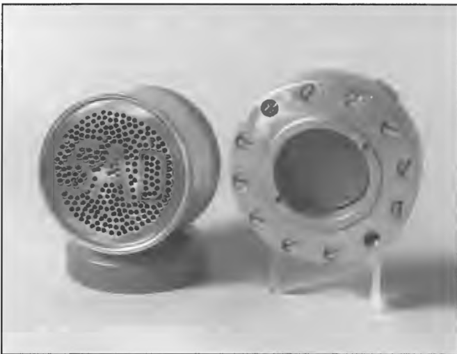
Many stations with good workshop facilities manufactured their own microphones in the 1930s. This condenser type was manufactured by staff at 5AD Adelaide. The station began operation in August 1930.
