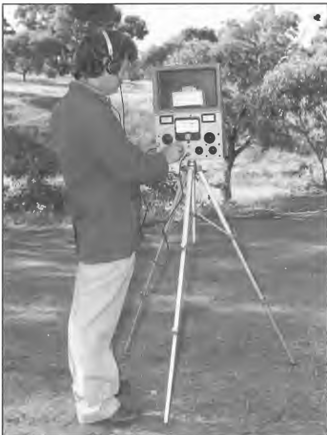
RCA type WX2E field intensity meter used for many years in the measurement of the field intensity produced by an MF radiator for a number of purposes including determination of figure of merit of the radiator, a field strength survey of the service area of the station and determination of the extent of night-time fading. The meter covered the range 540 kHz to 1600 kHz. An earlier RCA model employed in the late 1930s, the type TMV75B covered the range 515 kHz to 20 MHz. Operator, Brian Kennedy.
