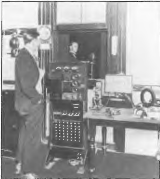
Program amplifier, control panel and wavemeter, 6WF Perth 1924. The panel, equipment and microphone were manufactured by Western Electric Co., USA who also provided broadcasting station equipment for stations in England and USA. George Sutherland Chief Operator near control panel and Walter Coxon, Chief Engineer and Manager, near microphone behind observation window.
