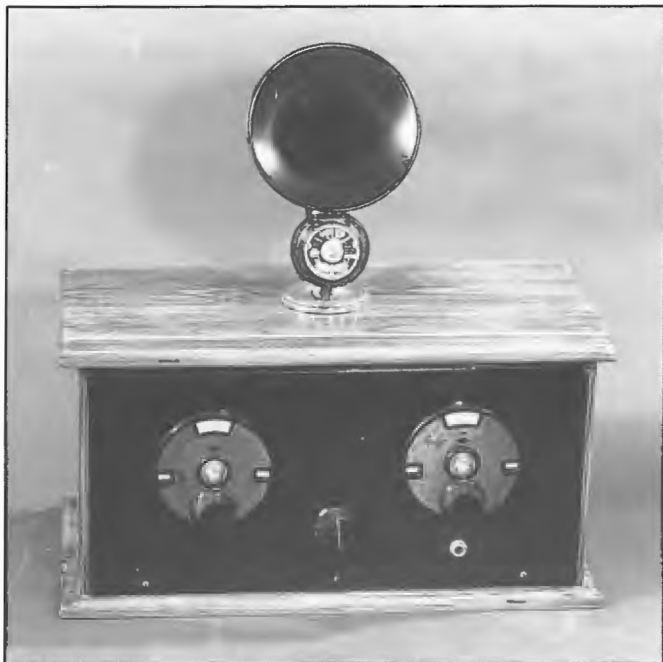
Two valve battery receiver made in 1927. It employed a regenerative circuit with reaction being achieved by variable capacitance feedback. Dials controlled tuning and the reaction capacitor. The third control was a rheostat for filament voltage control. The owner, a Mechanic in the Post Office built the set while living in Perth but brought it to Adelaide in 1929 when transferred to that city.
