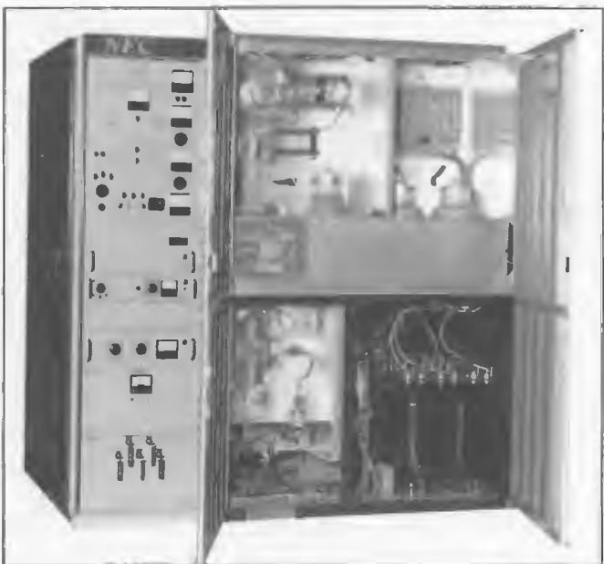
NEC type MBN-7237B 5 kW medium frequency broadcast transmitter installed at Commercial stations late 1970s. It employed four high gain tetrode valves, one in exciter stage, two in modulator and one in PA. Other stages employed solid state circuits.
