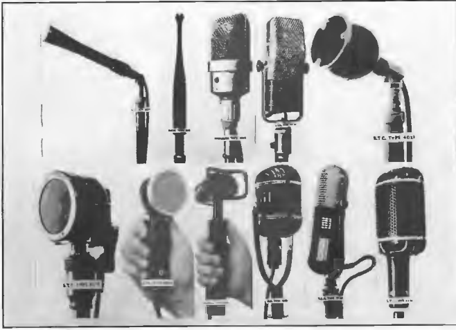
Typical microphones used in studios and for outside broadcast work by the ABC in the 1930-1950 period. Many were also used by Commercial stations. They included condenser, ribbon and moving coil types.
