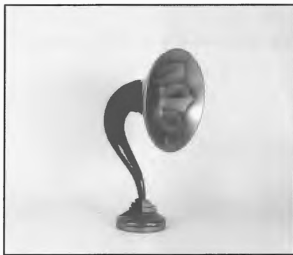
5. Sterling Baby, 1923. Made by Sterling Telephone and Electric Co., UK. Metal horn with sprayed leaf decoration in antique gold in the flare. Sensitivity control lever in base unit.
