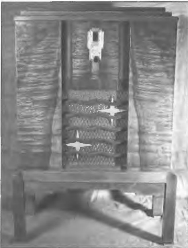
Philips luxurious Radioplayer five valve Model 1404M AC powered receiver, 1931 featuring the Philips 'stars and waves' motif on the loudspeaker grille. This was the second design produced by Philips when they began manufacture of broadcast receivers in Australia in 1931. The model featured a TRF circuit, cast aluminium chassis, recessed tuning and volume controls on the sides of the cabinet, a pressed metal hood covering the tuning capacitor and Philips type 2118 loudspeaker. Receiver production ceased shortly afterwards and did not resume until 1934.
