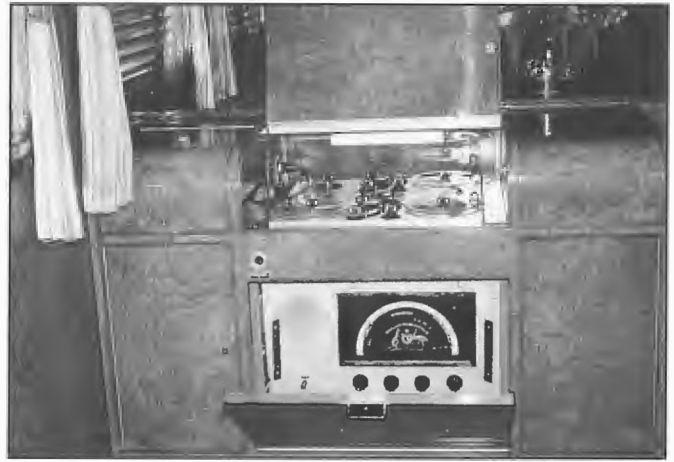
Broadcast receiver and tape deck installed in Lounge Car of Commonwealth Railways train travelling between South Australia and Western Australia for entertainment of passengers.
