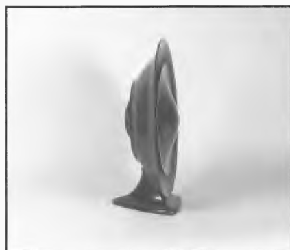
21. Mullard Pure Music Model E, 1927. Made by Mullard Wireless Service Co., UK. Paper cone driven by moving iron mechanism. Mottled brown bakelite body with cast metal base. Similar model by Philips.
