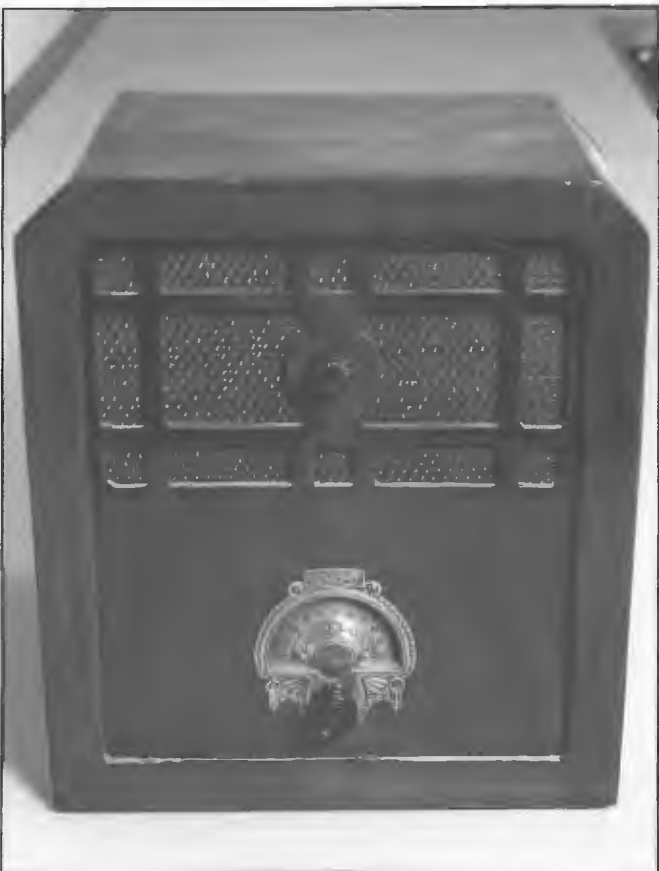
Baby Astor lacquered metal cabinet three valve battery-powered regenerative receiver with screen grid RF amplifier manufactured in 1931 by Radio Corporation Pty Ltd, South Melbourne. Valves comprised Philips A442 screen grid, Philips A415 detector and B409 power amplifier. It had long range reception capability and was popular with country listeners. This receiver purchased by Postmaster Goulburn, a few weeks after 2GN began transmission on 17 December 1931.
