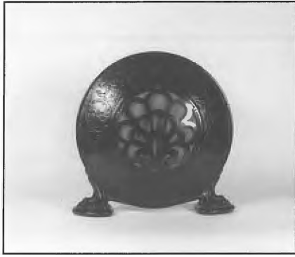
22. Utah Cone, circa 1926. Made by Utah Radio products Co., USA. All wooden enclosure with elaborate embossing. Utah were the largest manufacturers of loudspeakers in USA at the time.
