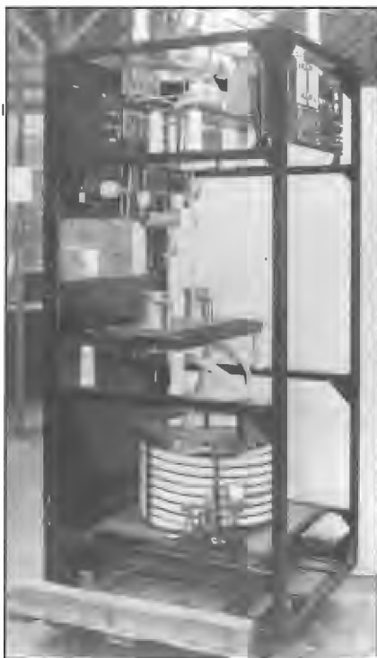
Power amplifier unit 2CO Corowa and 5CK Crystal Brook at the installation stage 1931/32. The unit contained two WE4220B water cooled valves, hose coils, water flow and water temperature alarms plus anode and grid meters on the front panel.
