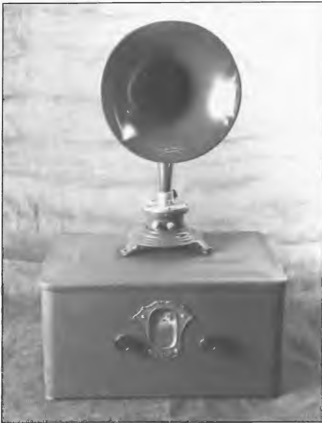
Baby Astor lacquered metal cabinet three valve battery-powered regenerative receiver with screen grid RF amplifier manufactured in 1931 by Radio Corporation Pty Ltd, South Melbourne. Valves comprised Philips A442 screen grid, Philips A415 detector and B409 power amplifier. It had long range reception capability and was popular with country listeners. This receiver purchased by Postmaster Goulburn, a few weeks after 2GN began transmission on 17 December 1931.
