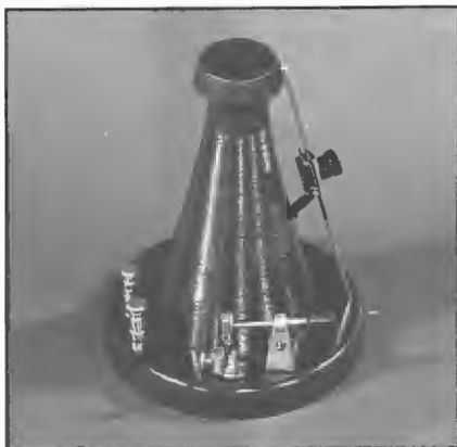
Crystal set using a tapered coil and single slider available in 1925. Distributed capacitance of the winding provided resonance conditions. The tapered coil enabled a more even spread of station positions along the slider. The crystal was gripped by a screw mechanism with a moveable serrated jaw. Radio Shops which sold this model included John Lunn, a Chemist and Licensed Radio Dealer of Sandgate near Brisbane, and Varcoe and Co., Adelaide.
