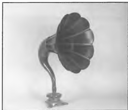
4. Burndept Ethovox Type 750, 1923. Made by Burndept Ltd, UK. Sectioned mahogany petal design flare held together with metal ribs. Painted metal swan neck and cast metal base.
