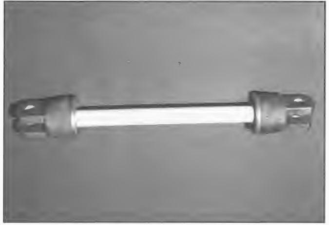
Strain type low loss ceramic insulator provided with aluminium alloy end caps to minimise corrosion problems with aluminium or aluminium covered steel conductors (alumoweld) employed with transmission lines and aerial systems at high frequency broadcasting stations including Radio Australia and NBS HF Inland Service in Northern Territory.
