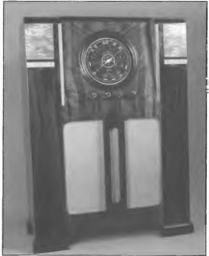
Five valve AC powered Gladiola Radio receiver manufactured by Gladiola Co., Adelaide, 1939, with SA stations being highlighted on the dial. The company made some parts and produced a range of mantle and console models including a radiogram. Cabinets made by the company, a former cabinet maker, were noted for their high quality veneer designs. First receivers using chassis brought in from outside, were released in the late 1920s. Proprietor, William Black. Son, William was responsible for radio aspects of the business.
