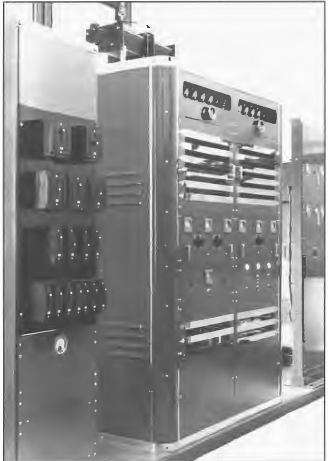
Station 5KA Adelaide 500 watt transmitter made by station staff 1938. Most of the major components including transformers, chokes fixed capacitors and rheostats were manufactured in the workshop. The final amplifier used four 805 type valves in parallel push-pull configuration. The unit was originally installed at Currie Street but in 1943 was transferred to a building in Franklin Street. Chief Engineer during construction of the transmitter was Charlie Tareha.
