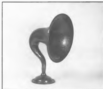
18. Kellogg Symphony Reproducer, 1925. Made by Kellogg Switchboard and Supply Col., USA. Magnetic diaphragm. Moulded non metallic composition body and flare with black and gold crocodile pattern finish.
