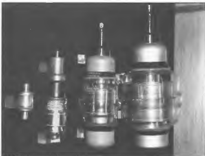
Typical vacuum capacitors used in modern transmitters and aerial coupling units. Fixed capacitors using vacuum as a dielectric were first manufactured in 1937 but did not find acceptance with Broadcast Engineers until about 1950 when concentric re-entrant flange construction technology was employed. The introduction of high power transmitters resulted in widespread use of this type of capacitor in high voltage circuits.
