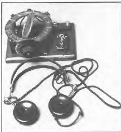
Crystal sets employing basket weave coils had a strong following in the 1920s. Although more difficult to wind than a standard cylindrical type, they could be easily made up as a fixed/variable combination. The method of winding was to turn the wire in and out between spokes on a special former, or slots in a cardboard former. A kit set for the crystal set shown was available from Bullocks Cycle and Radio Stores, Adelaide in 1927.
