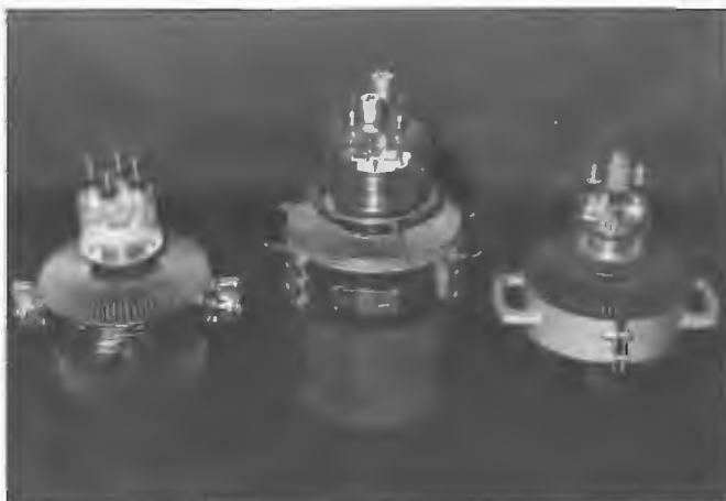
Typical large forced air cooled transmitting valves. (L to R): Ediswan ESA5000, 3J/261E and ML899RA. The Ediswan ESA5000 was a direct replacement for the American ML899RA and both were used with 10 kW transmitters installed at Radio Australia in 1945. The 3J/261E was used in the modulator and power amplifier stages of STC 55 kW MF transmitters installed at many National stations.
