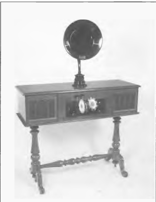
Two approaches to battery receiver cabinet designs of the early 1920s. In one model, the A and B batteries were housed in wing compartments while in the other they were mounted in a cabinet below the receiver. The Browning-Drake
