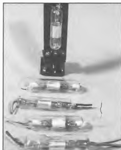
A collection of double ended receiving type valves used in Adelaide by Bill Bland circa 1923 with his experimental station 5AG. Notes found with his papers indicated he had at various times acquired valves manufactured by Lee de Forest, Elmer Cunningham, Harry Roome and Otis Moorhead in USA; Expanse from AWA and an Annaka brand valve from a Japanese ship's wireless operator during a visit to Adelaide. Bill Bland was involved in experiments with broadcasting technology from about 1920 and in 1927 established Bland Radio, a major receiver manufacturing company in Adelaide.
