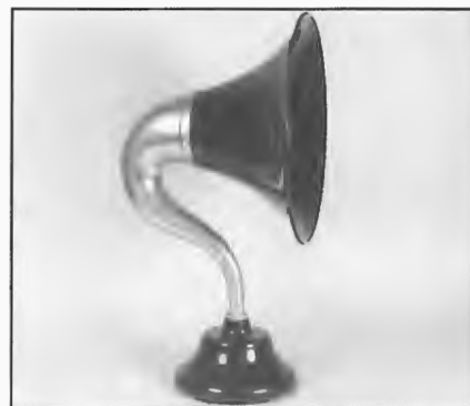
3. BTH Type C2, 1923. Made by British Thomson-Houston Co., Ltd, UK. Aluminium swan neck, painted aluminium flare, brown bakelite base and air gap screw for adjustment of sensitivity.
