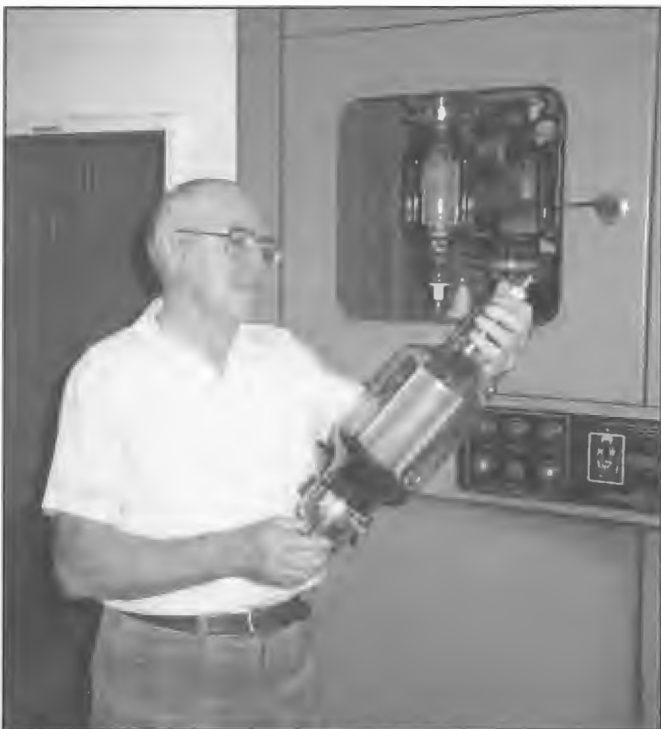
A 4279Z valve being examined by Ray King alongside one of two STC 2 kW type 4-SU-14 transmitters installed at NBS station 4QY Cairns. When commissioned on 20 January 1950 the power amplifier and modulator stages were each equipped with a pair of 4279A type valves. The valves were subsequently replaced by 4279Z types manufactured by STC in their Sydney valve factory. The station was closed down during April 1997. First Officer-in-Charge, Eric Gough.
