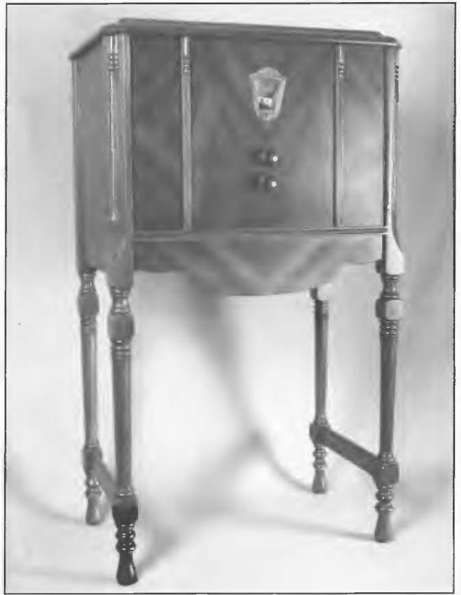
Stromberg-Carlson three valve TRF receiver, 1931. Valve types employed were E415 detector and audio; B442 output penthode and 1560 full wave rectifier. Built-in magnetic loudspeaker was mounted on a baffle underneath the cabinet shelf. The Lucan Console cabinet was finished in Queensland walnut and was used to house three and four valve receiver models. It was distributed by Mick Simmons Ltd, Sydney.
