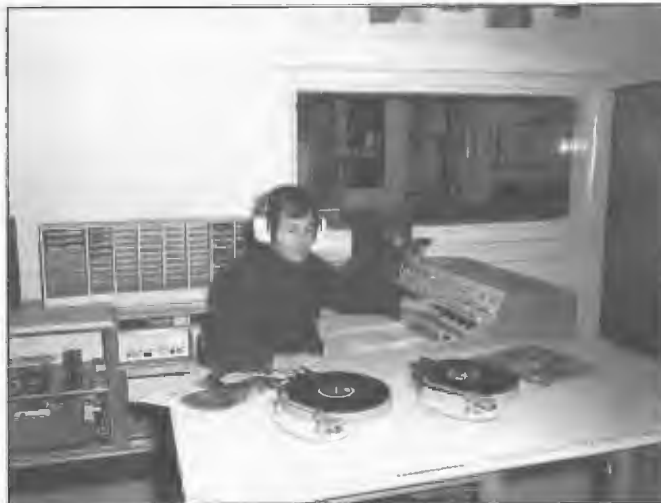
Enclosed type high quality headphones used by Commercial station announcer in 1960s. Some announcers preferred a single headphone unit as it allowed them to cue up the next record item while still keeping an ear on the program already being broadcast.
