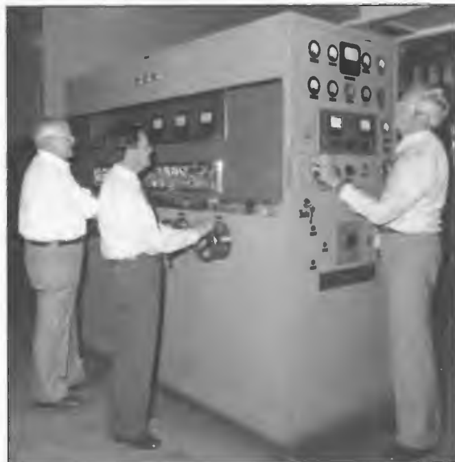
Last day of operation of STC/AWA 100 kW HF transmitters Radio Australia, Shepparton 1983. The transmitters were originally installed during 1946 and upgraded during the 1960s. Retired staff were invited to perform tuning operations of the old transmitters. (Left to right) Jack Nicholas adjusting PA tuning, Bill Davidson adjusting output tuning and Fred Barker adjusting input tuning.
