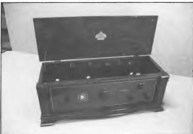
(A) Six valve King-Hinners Neutrodyne battery operated receiver manufactured by King Manufacturing Corp., USA and factory tested, according to label, on 15 July 1927. It was imported by Adelaide radio Dealer, Len Harper. The circuit comprised three RF stages, detector and two AF stages. Features included single
