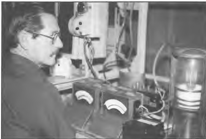
Carburising the filament during rebuilding of a transmitting valve at AWA works, Sydney 1987. The filament was flashed in a hydrocarbon vapour bell. The process ensured correct hot filament resistance and electron emission level and stability during service life. The company operated a rebuild service for some types of transmitting valves.
