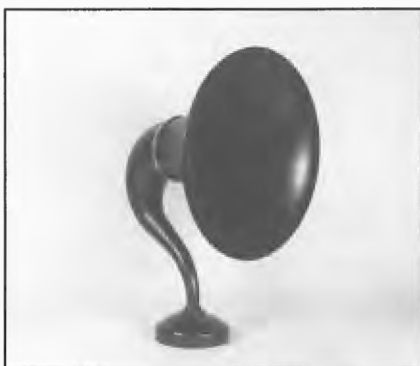
16. Reichman-Thorola, 1925. Made by Reichman Co., USA. Burnished bakelite horn with gold coloured throat band. Mica diaphragm with powerful magnet and driving rod.
