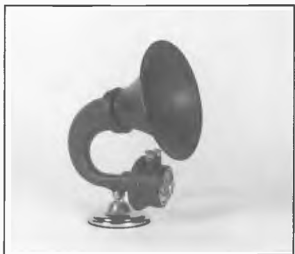
7. Amplion Dragonfly Type AR102, 1924. Made by Alfred Graham and Co., UK. Spun aluminium flare and cast metal horn. Black crystalline enamel finish.
