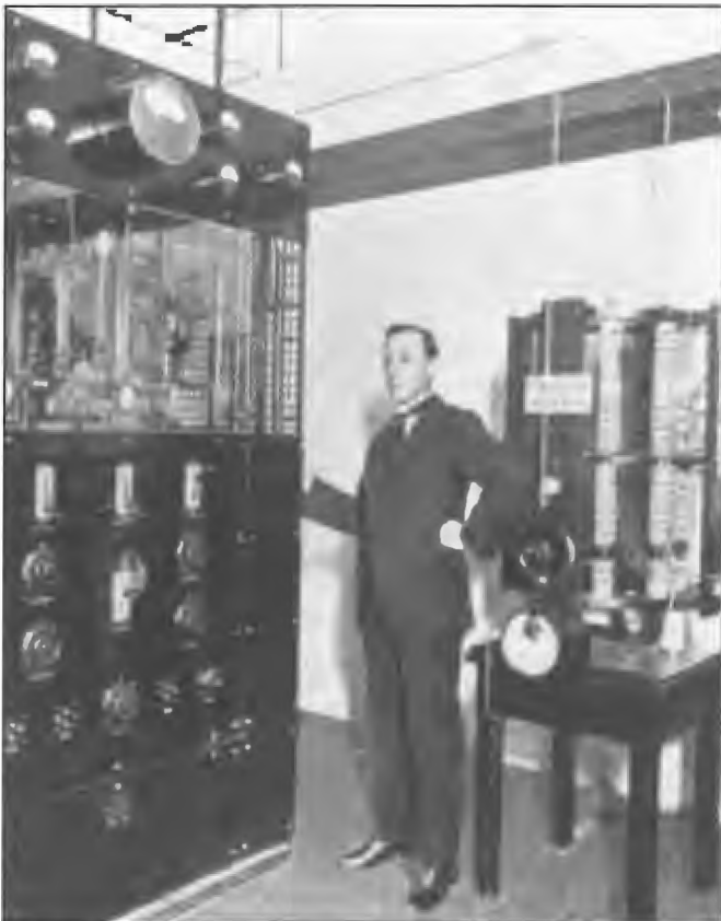
Walter (Walley) Coxon, Chief Engineer and Manager, Westralian Farmers Ltd beside the Magnifier unit of the 6WF 5000 watt AWA transmitter. It operated on 1250 metres (240 kHz). Service began on reduced power on 4 June 1924. Studios, transmitter and aerial were all located on the roof of the company building.
