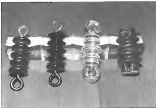
Typical insulators of the corrugated surface type used for home aerial installations. Materials commonly employed included porcelain, pyrex, ebonite, fibre and electrose. Outside aerials were rarely used after about 1946.
