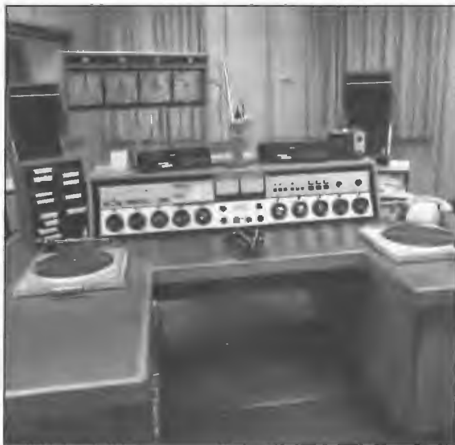
ABC FM studio 508 Adelaide. The ABC FM Stereo network commenced in January 1976 with the commissioning of transmitters at Canberra, Sydney, Melbourne and Adelaide with programs originating in the ABC studios in Adelaide where two studios were provided.
