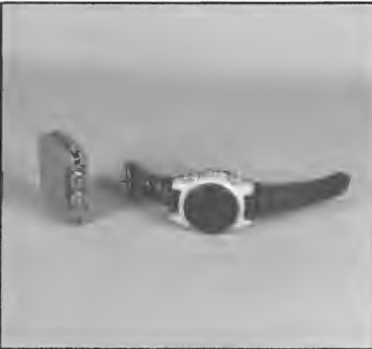
Imported miniature solid state receivers marketed as Purse Set (left) and Wrist Set in 1970s. Following the introduction of the first commercially produced all-transistor radio in 1955 under the Sony label, a pocket size version was released the following year.
