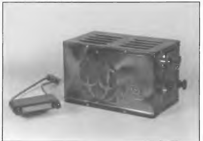
Model 510 Endeavour car radio manufactured in 1934 by Eclipse Radio Pty Ltd. It was a six valve superheterodyne type enclosed in a metal case. AVC was applied to the RF amplifier, IF amplifier and pentagrid converter. Controller attached to the steering wheel column and linked to the receiver with flexible Bowden cables. A selection of remote control units was available. Works Manager, Bill Kerr and Chief Laboratory Engineer, George Williams.
