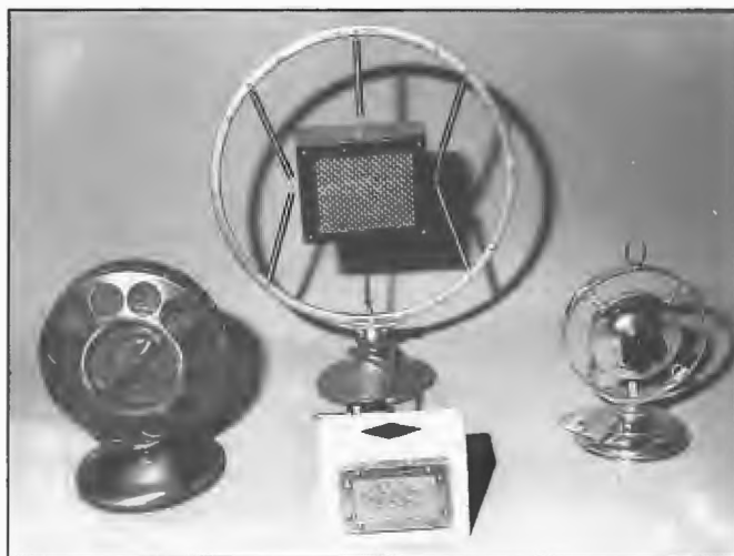
Typical carbon granule type microphones used during the 1920s. They included the Western Electric double button type, a suspended French made model, a marble cased transverse current type and a solid back type. The transverse current type was also referred to as a Reisz type and many were manufactured by station staff.
