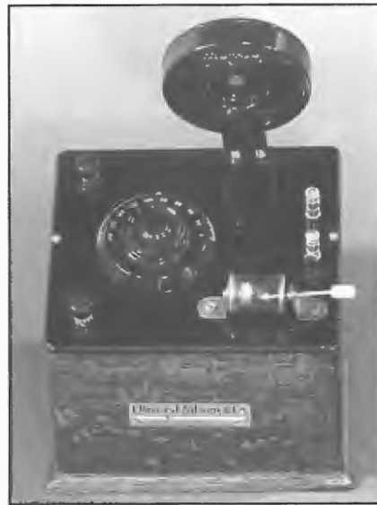
The Super crystal set manufactured by Oliver J Nilsen and Co., Melbourne, 1926. It employed an enclosed crystal and cat's whisker and plug-in coil. The model was popular even in the early 1930s.
