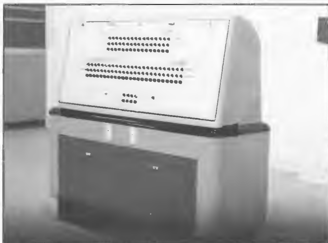
Aerial Switching Control Desk Radio Australia, Shepparton 1945. The desk controlled external line switches by means of push buttons. There was a push button for each aerial and aerial direction available to its associated transmitter. Once the transmitter was powered, the DC supply to the desk was removed so preventing shifting of power carrying switches. Officer-in-Charge, Jack Hargreaves.
