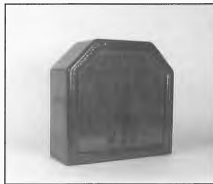
15. Celestion Cone C12, 1927. Made by Celestion Radio Co., Ltd UK. Piston diaphragm. Both sides of paper cone reinforced with copper wire. Mahogany cabinet.
