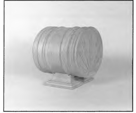
24. Operadio Senior, 1928. Made by Operadio Manufacturing Co., USA. Featured a horn moulded in the shape of a human ear. Drive system acted on an aluminium diaphragm. Patented 1927.
