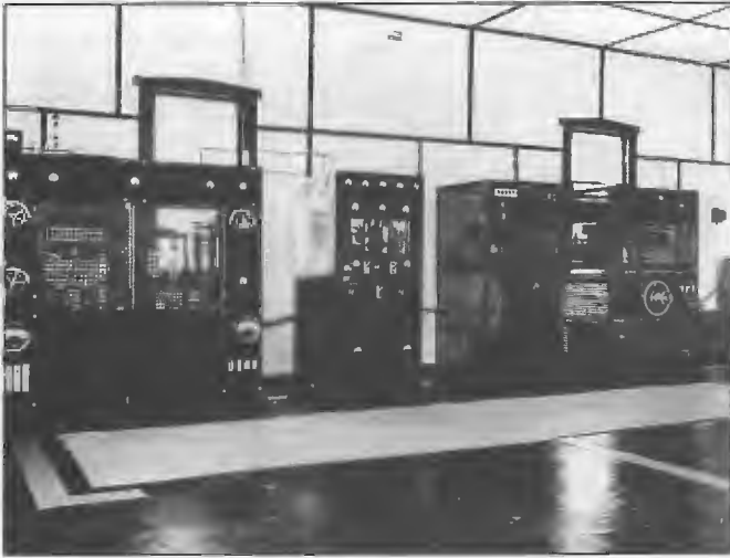
Station 5PI Port Pirie 2000 watt transmitter 1934. Designed and constructed by 5AD Adelaide staff under Chief Engineer Don Gooding. Final stage employed STC 4228A water cooled valves with filament power being supplied by two DC generators 24 volts at 100 amperes.
