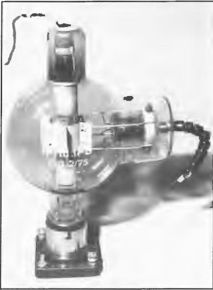
Philips QB2/75 screen grid transmitting valve with oxide coated filament and maximum anode voltage of 2000 volts. Anode dissipation was 75 watts. Commercial station 3BA employed one of these in the final stage of the transmitter when it was commissioned on 31 July 1930. The transmitter produced 50 watts into the aerial. Manager and Station Engineer Warne Wilson, Operating Engineer, Alf Kerr.
