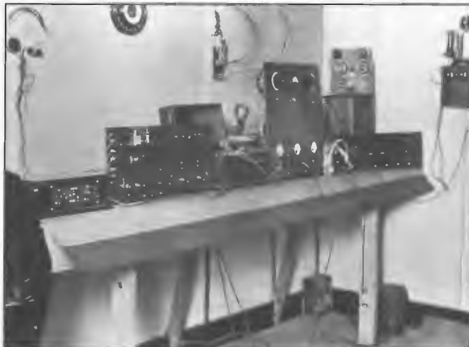
Original 5DN Adelaide transmitter 1924. The transmitter was previously used with an experimental station operated by Lance Jones. The speech input equipment included microphones purchased direct from Western Electric Co. in USA by the station owner Mr E J Hume. Initially, input to the final stage was 35 watts.
