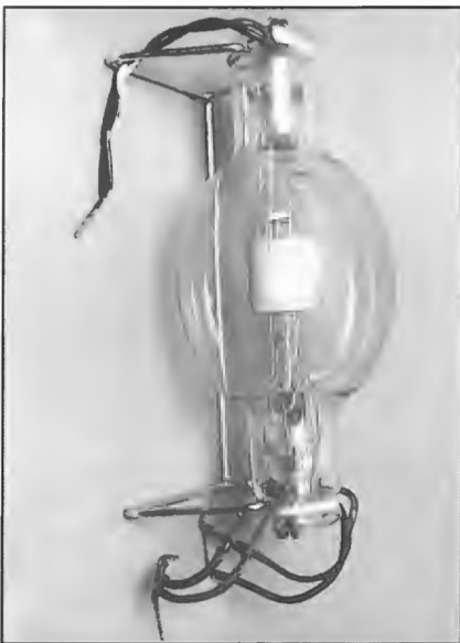
Typical radiation cooled transmitting valve used in the early 1920-30's known as 'football' valves. The valve was mounted vertically in a cushioned bracket keeper and the flexible leads were inserted in standard brass clamping terminals.
