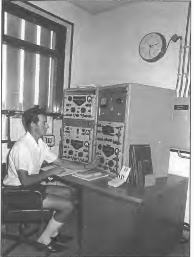
Reconnaissance position with three Racal HF receivers type RA117-C2 and panoramic adaptor at Receiving Station, Cox Peninsula, 1969. The equipment was used for collection of occupancy data as part of work in preparing Radio Australia transmission frequency schedules. The panoramic adaptor provided a visual representation of transmissions in a band at a particular time. Operator, Mal Stewart.
