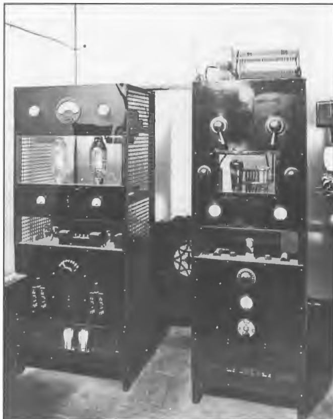
Original 50 watt 3BA Ballarat transmitter commissioned 31 July 1930. The station was established by two local radio experimenters Warne Wilson and Alfred Kerr. The locally constructed transmitter was contained in two cubicles and produced 50 watts of carrier power. The power amplifier valve was a Philips QB2/75 type.
