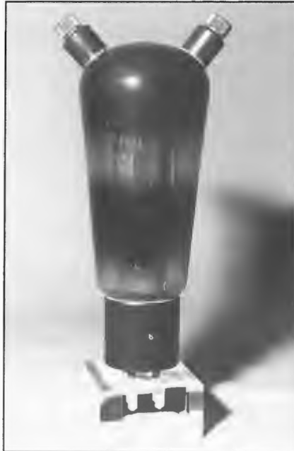
Philips TC04/10 valve widely employed in low power Commercial transmitters in the early 1930s, and known as a 'horn' valve due to its appearance. This valve was used in the crystal oscillator buffer stage at 3WR when the station went on air in January 1931, producing 50 watts into the aerial. Station 3WR originally went on air on 25 February 1925 but closed down on 22 December of the same year as a public broadcasting station. It began again on 5 January 1931 with new studio and transmitting facilities designed by Les Glew and manufactured in the Melbourne workshops of Oliver J Nilsen.
