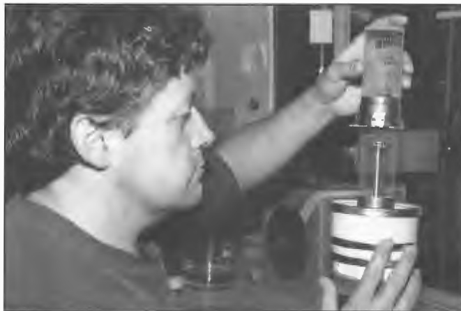
As part of a valve rebuild operation, grids were concentrically lined up with respect to the filament strands to ensure correct electrical characteristics. Rebuilt valves gave comparable operating life at less than half the cost of a new valve.
