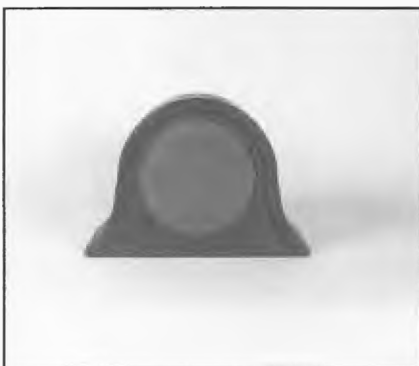
17. Steward-Warner Magnetic Cone Reproducer, 1927. Made by Stewart Warner Corpn, USA. Bidirectional in cast metal case. Four pole balanced armature system.
