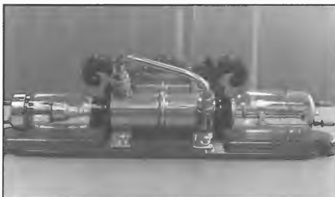
A mounted double ended water cooled valve 3Q213E as employed with early STC 10 kW 4QR/VLQ Brisbane transmitters as replacement for original SS1971 type valves and presented to Doug Sanderson on the occasion of his retirement in 1989. Doug was an Engineer with Postmaster General's Department/Telecom and spent most of his career extending over 48 years with the National Broadcasting Service.
