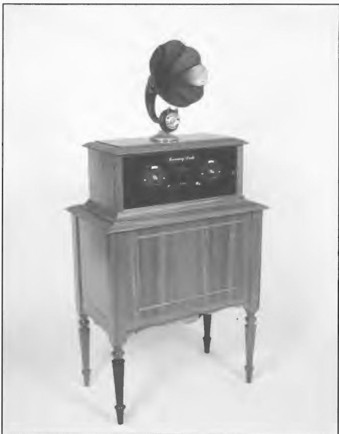
receiver (right) used a circuit developed by Glenn Browning and Fred Drake in USA. The key to the receiver's high performance was a new type of RF transformer known as the National Regenaformer.
