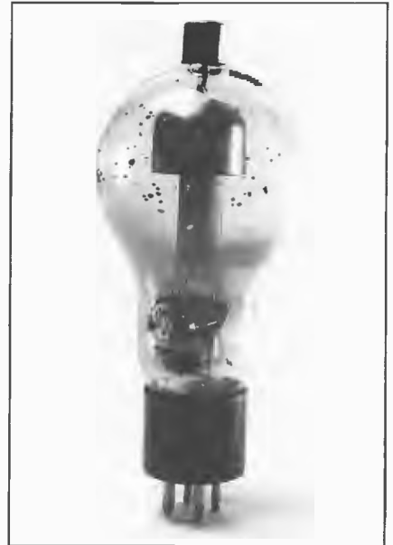
The 866/866A hot cathode mercury vapour rectifier was one of the most widely used rectifier type valves in Commercial and National transmitters from the early 1930s. It was rated at 1 ampere peak anode current and 10000 volt inverse peak. This valve was employed in the medium voltage rectifier circuit of VLQ short wave transmitter STC type A880A commissioned at Bald Hills on 17 February 1943. Officer-in-Charge of installation, Arthur Clark.
