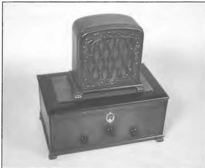
Kolster Model 20 manufactured for Kolster Radio Corporation, USA, in 1928. This receiver was purchased from Homecrafts, Melbourne, about 1930. The receiver cabinet and a matching loudspeaker were patterned using wood under high pressure in a steel mould. The patent for the process was held by Brandes Laboratories. The set was AC powered and employed 7 valves including rectifier, three RF, one detector and two AF stages.
