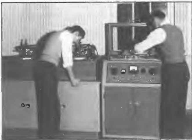
Technical staff dubbing from console tape recorder machine to disc recording unit at 4BC Brisbane studios circa 1955. Console tape recorders were widely employed at Commercial and National studios from about the mid 1950s. They were frequently installed in pairs with a matching control console between the recorders.
