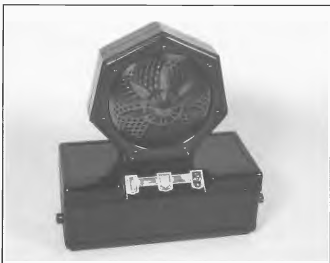
Philips All Electric Model 2510 Radioplayer with Sevenette loudspeaker. Produced in Holland, 1930, it was housed in metal casing with five Arbolite panels of thin plastic laminated board. The receiver employed two stages of screen grid amplification. The lid was hinged and could be locked. Purchased by a publican in Broken Hill from Philips, Sydney, in mid 1932, shortly after broadcasting stations 5CK and 5PI began operation in Crystal Brook.
