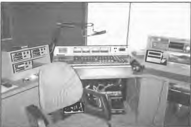
Ward Beck console, Sonifex cartridge machines and other facilities at 2NEW FM Newcastle operated by Newcastle FM Pty Ltd. The console was originally installed at studios in Darby Street, Newcastle and transferred to studios in Sandgate with operations at the new site beginning on 5 November 1995. Chief Engineer is Ian Porteous.
