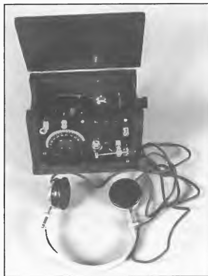
Homemade receiver using open crystal detector and single valve audio amplifier. Tuning by capacitor, and rheostat provided for valve filament voltage adjustment. Constructed 1926 by member of Glenelg Radio Club, Adelaide.
