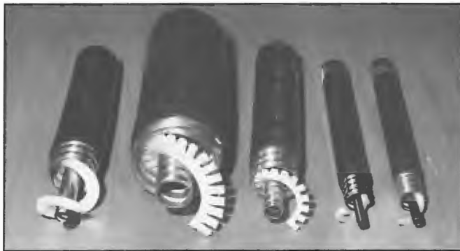
wide range of power levels and construction including outer conductors of braided, smooth tubular or corrugated materials; stranded, solid or tubular inner conductors; and solid, air or foam dielectrics.
