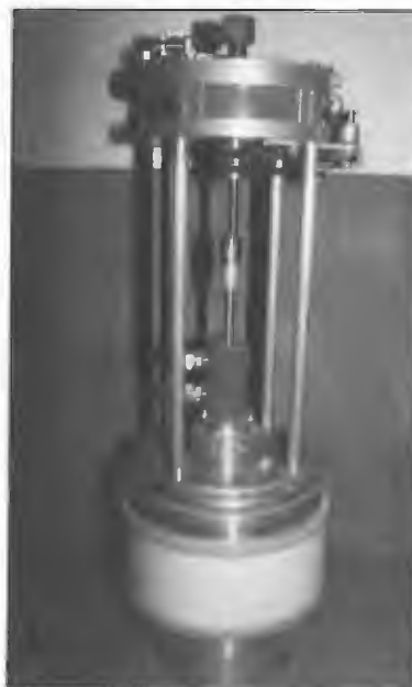
The Comet capacitor modified to fit into the Collins transmitter. It enabled tuning of the transmitter over the designed range 6-26 MHz without any component change.
