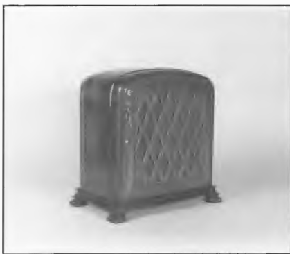
14. Kolster Cone Reproducer Model K6, 1928, Made by Kolster Radio Corpn, USA. Wooden cabinet embossed by a steam heated mould during manufacture.
