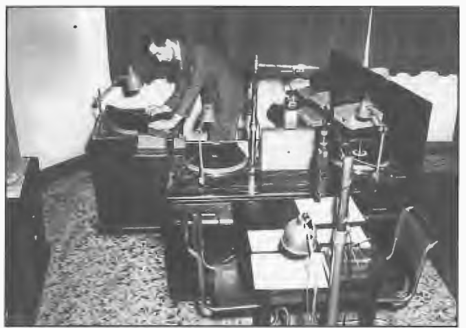
3UZ studio 1947, operated by Nilsen's Broadcasting Service Pty Ltd. Facilities included a replay unit to allow Announcer to check a record without using control desk, a standard announcing desk and control panel and an interview desk with time gong.
