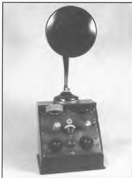
Fellophone Super Two, a two valve receiver manufactured by Fellows Magneto Co., Ltd, England, 1923 and purchased by a listener at Murray Bridge in mid 1925 from Varcoe and Co., 57 Gawler Place, Adelaide. The receiver had a sloping fronted cabinet with an ebonite panel on which was mounted controls, valves and plug-in coil. One high frequency valve and one detector were used with reaction. Selectivity was obtained by coupling the tuned anode coil.
