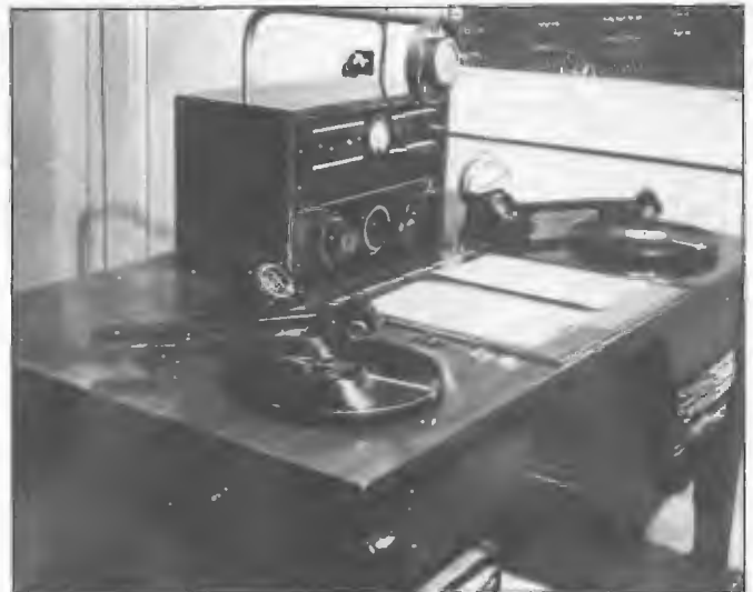
Emergency studio at transmitting station 3GI Sale, the first Victorian Regional station of the NBS to begin service when it was commissioned on 30 October 1935. Facilities included STC 4017 microphone, two WE4A gramophone reproducers, STC mic/gramophone amplifiers and two receivers. Divisional Engineer Harold Robertson.
