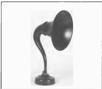
8. Siemens, 1924. Made by Siemens Bros., UK. Cast metal base, spun aluminium flare and aluminium swan neck. Black enamel finish.
