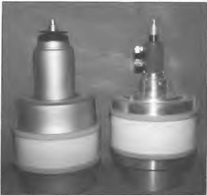
Main water cooled tuning capacitors used with Collins 250 kW transmitters Radio Australia, Cox Peninsula. Jennings CVT 1600-70X types (left) were employed in the transmitters from 1969 but in 1992, Comet CV4W 1000E types were fitted. Both types had similar electrical characteristics. Capacity range was 100-1600 pF, peak working voltage 36 kV and maximum RMS current 1000 A.
