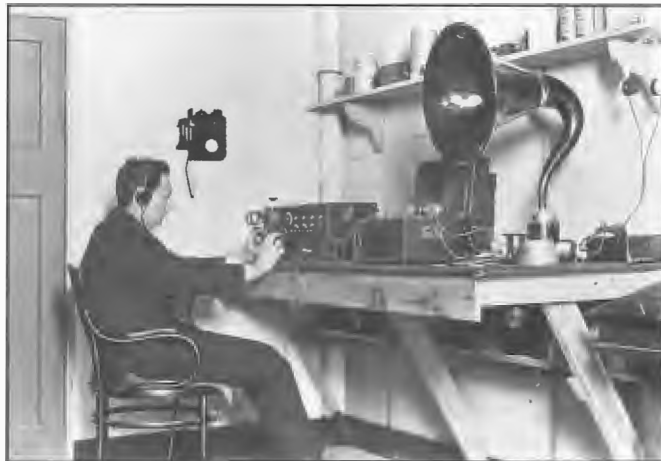
Receiving equipment installed at B Class station 5DN Adelaide 1924. Ern Hume in charge of technical facilities at the controls. Although the transmitter and aerial were located near the studio, program monitoring was carried out off-air. There was no pick-up monitoring point provided on the transmitter.
