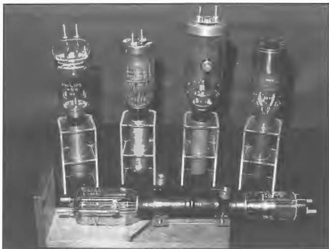
Water cooled transmitting amplifier and rectifier valves used with National transmitters. (L to R): Philips DA12/15, STC 4220C, Federal/ITT 124A, STC 4222A and (front) STC 3Q213E. The double ended valve 3Q213E replaced SS1971 types in 4QR and VLQ transmitters when SS1971 types were no longer manufactured. The first National transmitter provided with water cooled valves was 2NC Newcastle commissioned on 19 December 1930 by Engineer Harry Weir.
