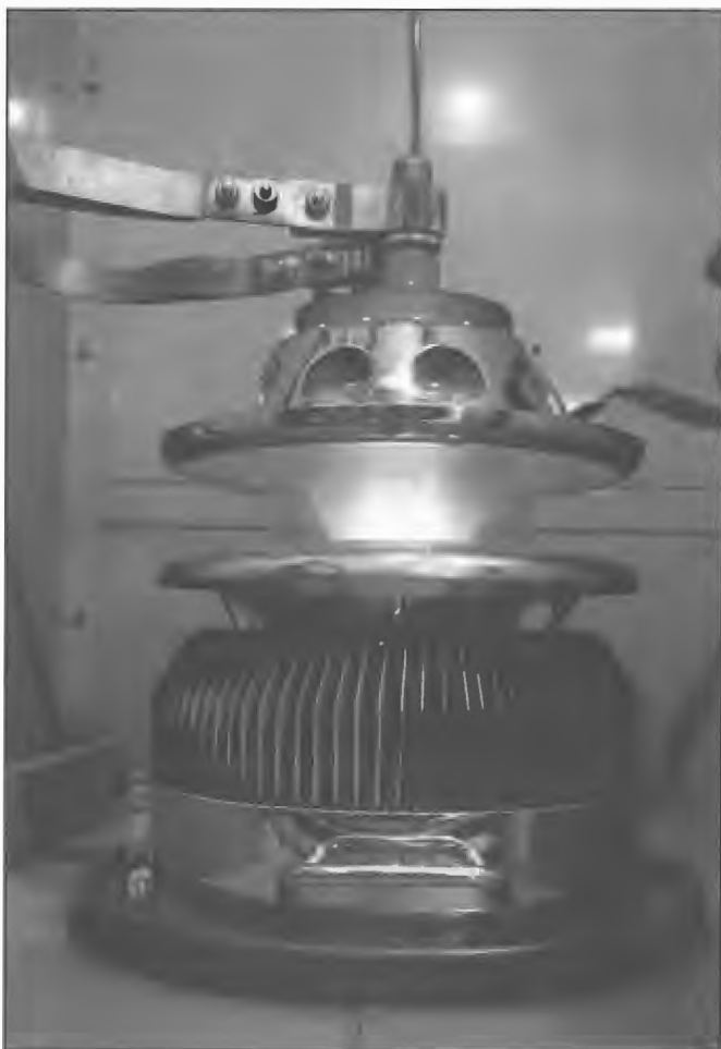
The GEC BR189 air blast triode which replaced the water cooled 4030C modulator valves in the Radio Australia, Shepparton 100 kW transmitters. The original transmitters were taken out of operational service in 1984 when Bruce Wilson was Officer-in-Charge.
