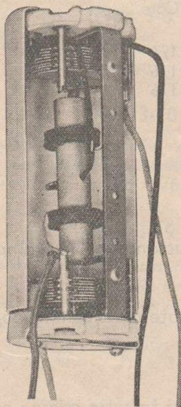
To increase selectivity and sensitivity and where 100% efficiency and absolute stability are essential requirements, these special type air tuned units are an absolute necessity.
