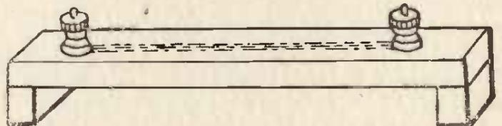
FIG. 2.—A home-made grid leak for use with a detecting (or rectifying) valve.
