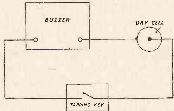
FIG. 1.—Showing connections of buzzer circuit.
