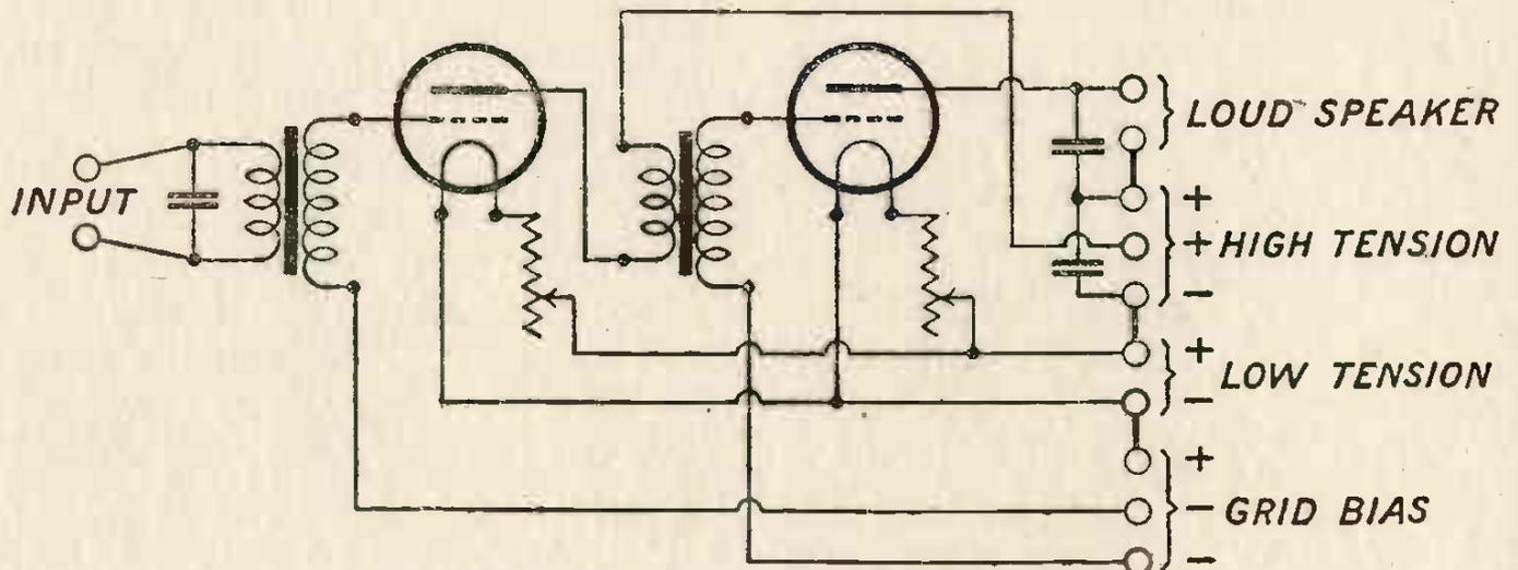
FIG. 2.—Showing the positions of the twelve terminals.
