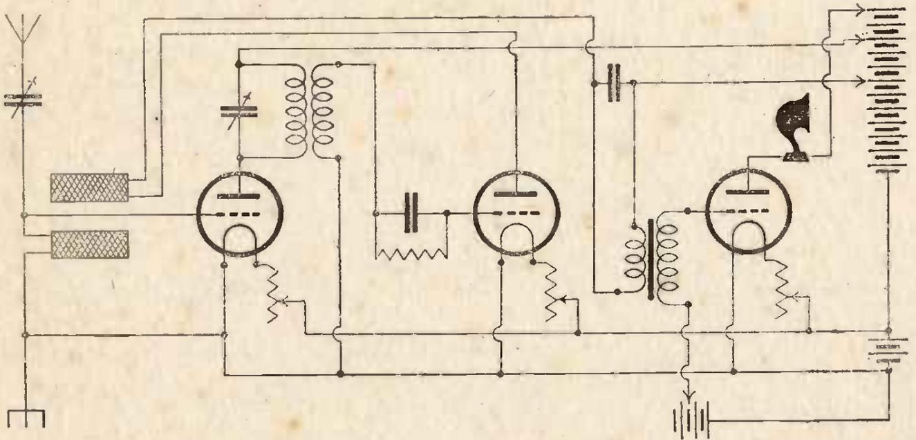
16. This circuit is similar to the previous one, except that the first and second valves are here coupled on the "tuned-transformer" principle. By using high-frequency transformers of the plug-in type, with a variable condenser across the primary, a very wide range of wavelengths can be received.
