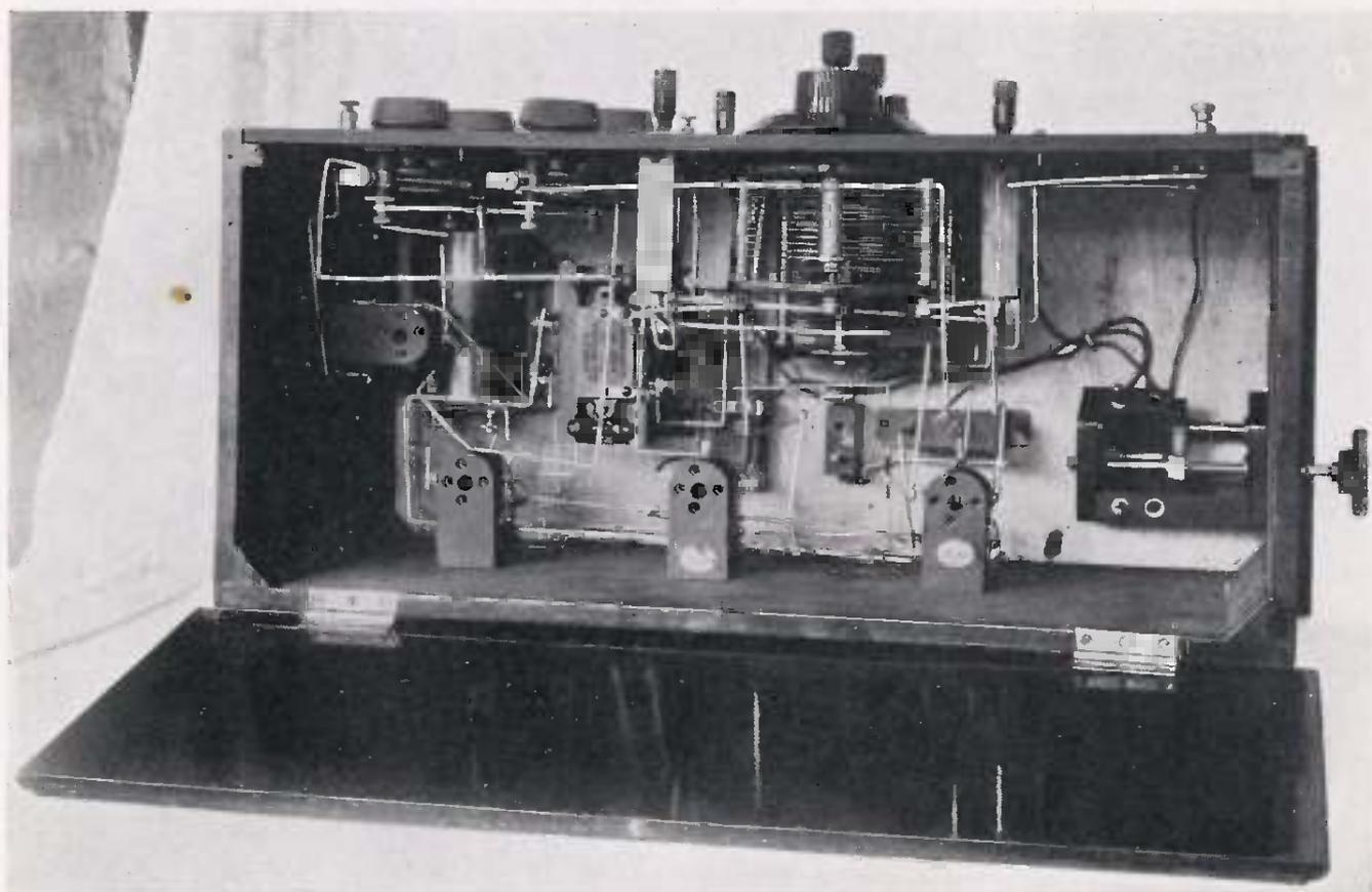
Interior view of Four-Valve All-station Receiver.
