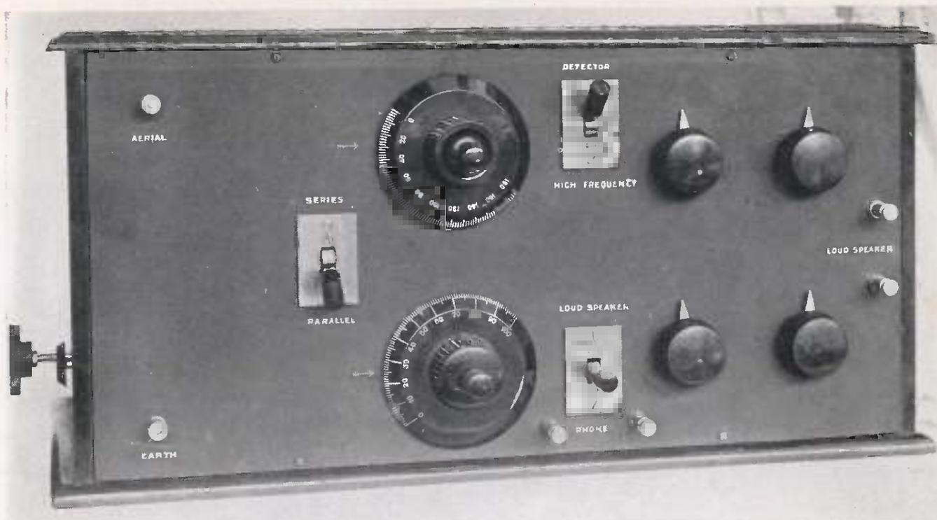
Front view of the Four-Valve All-station Receiver.
