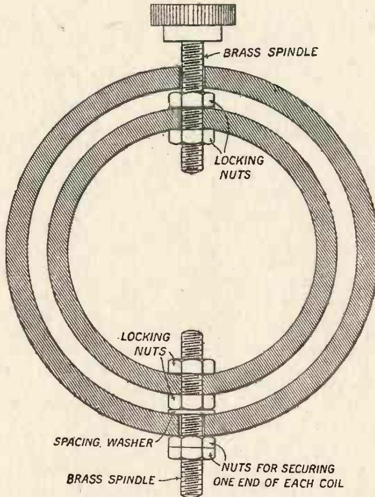
FIG. 11.—Arrangement of tubes for rotary variometer.
