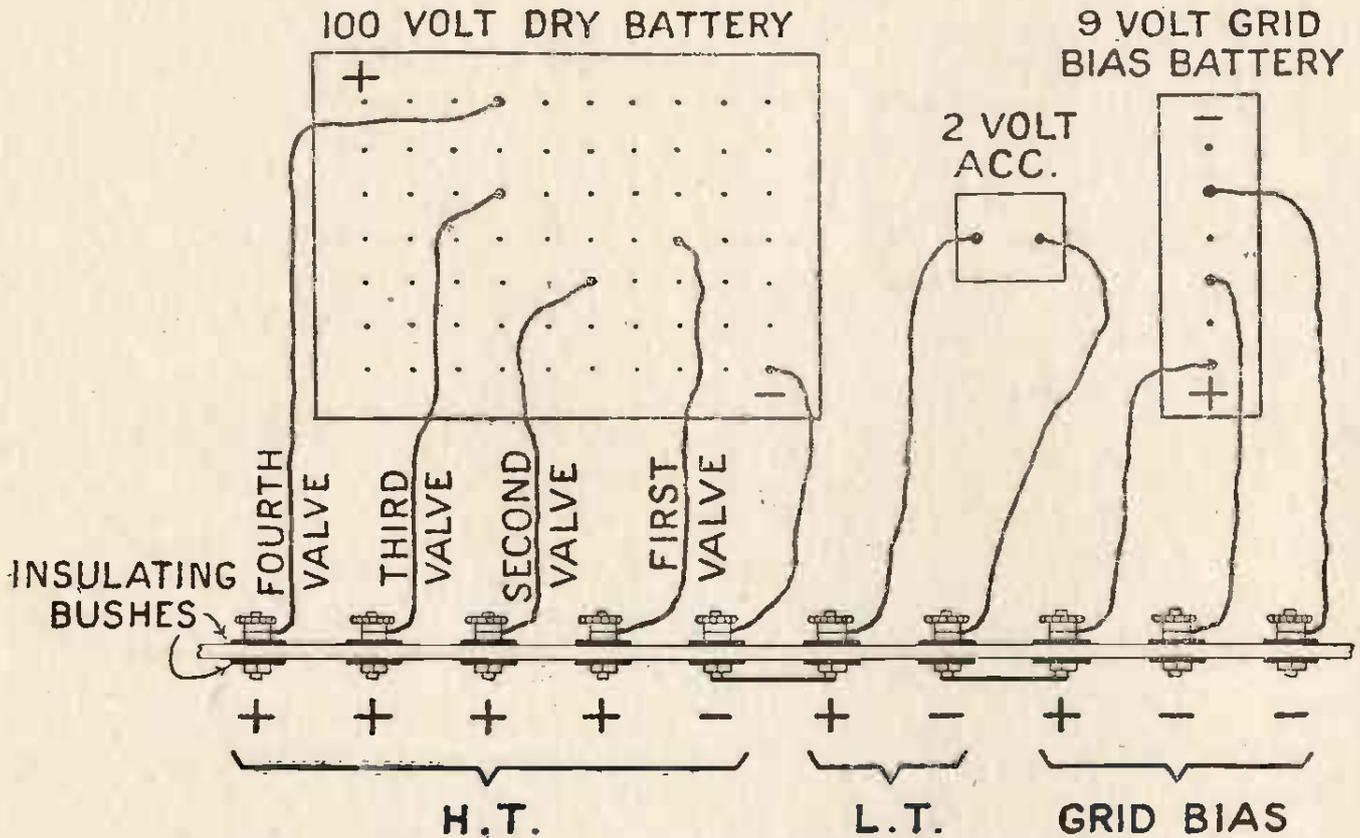
FIG. 2.—Showing connections from the three batteries to the terminals in back wall of cabinet.
