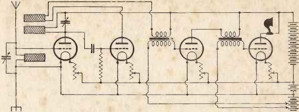
18. A four-valve, all-station receiver, in which the first valve is a high-frequency amplifier, the second a detector, and the third and fourth low-frequency amplifiers. Each low-frequency valve is provided with a separate grid bias.
