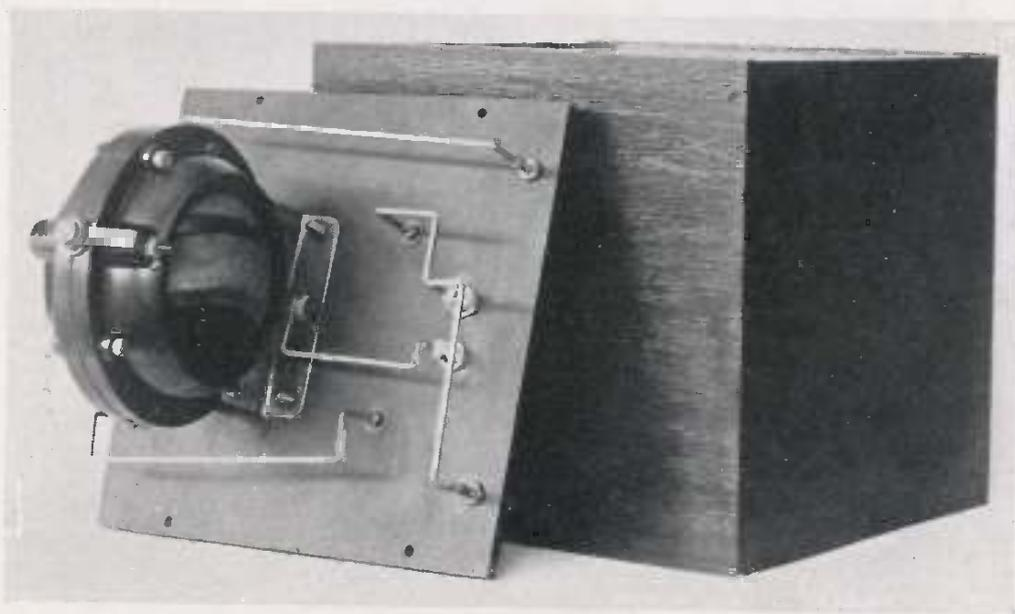
Showing internal wiring of Variometer Crystal Set.
