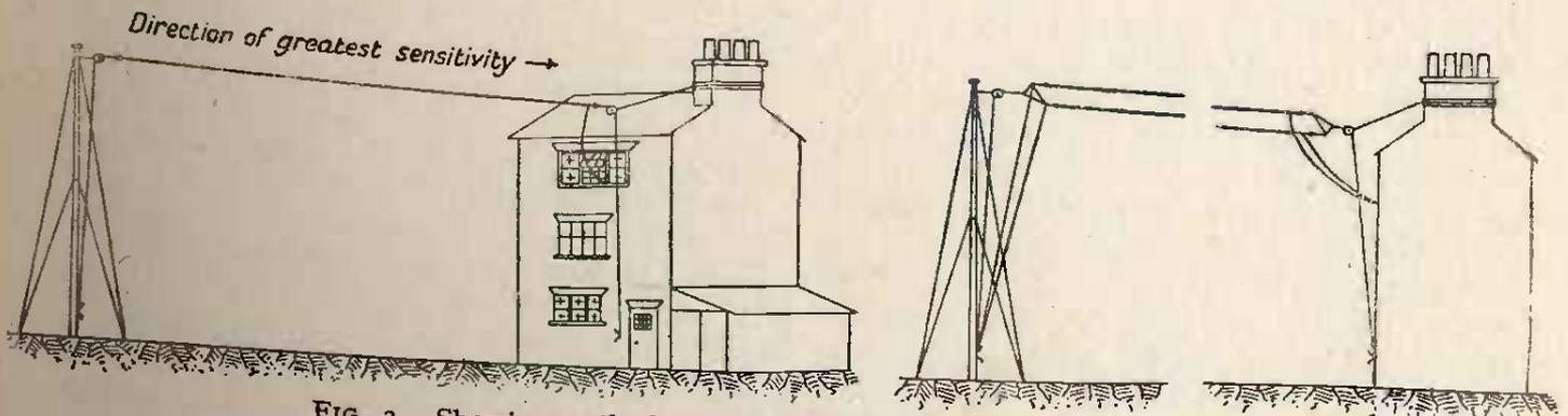
FIG. 3.—Showing methods of erecting single- and double-wire aerials.
