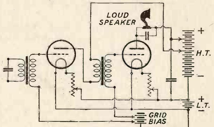
FIG. 1.—Diagram of connections of the amplifier.
