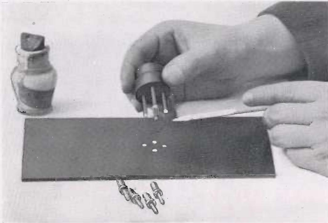
In order to ensure that the holes in the ebonite are drilled at the correct distances apart, the prongs of the holder, or of the valve itself, may be marked with white paint or chalk, and an impression of the latter reproduced on the ebonite, by contact. All traces of paint or chalk should afterwards be removed.
