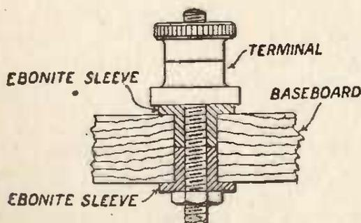
FIG. 6.—Showing how a terminal may be insulated from the base board by an ebonite sleeve.
