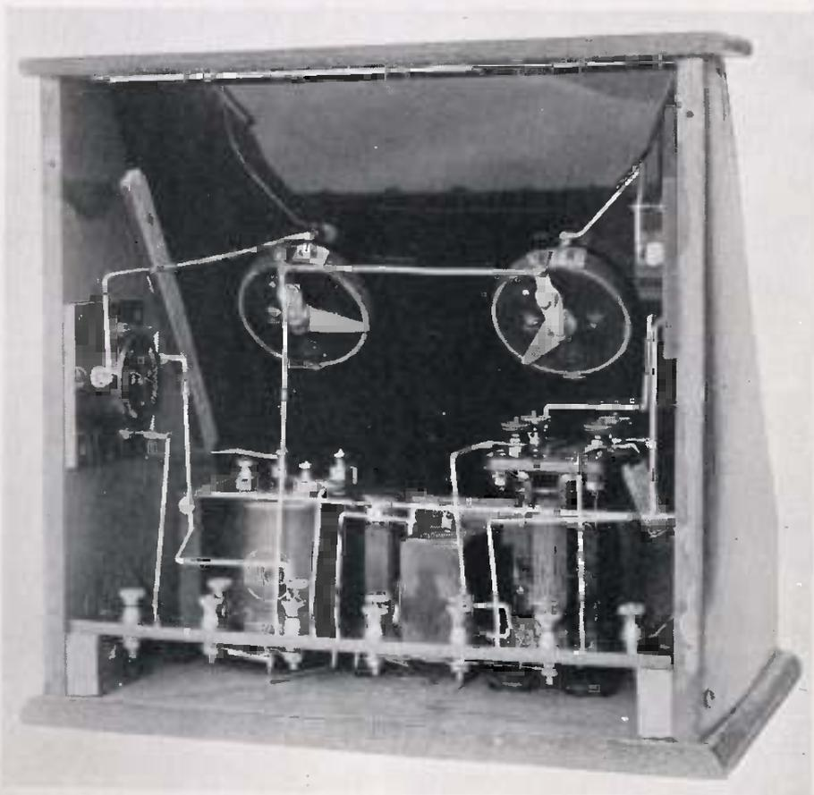
Rear view of the Two-Valve Amplifier.
