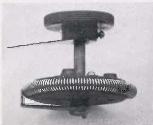
A manufactured rheostat, or variable resistance, for regulating the flow of current through the filament of the valve.
