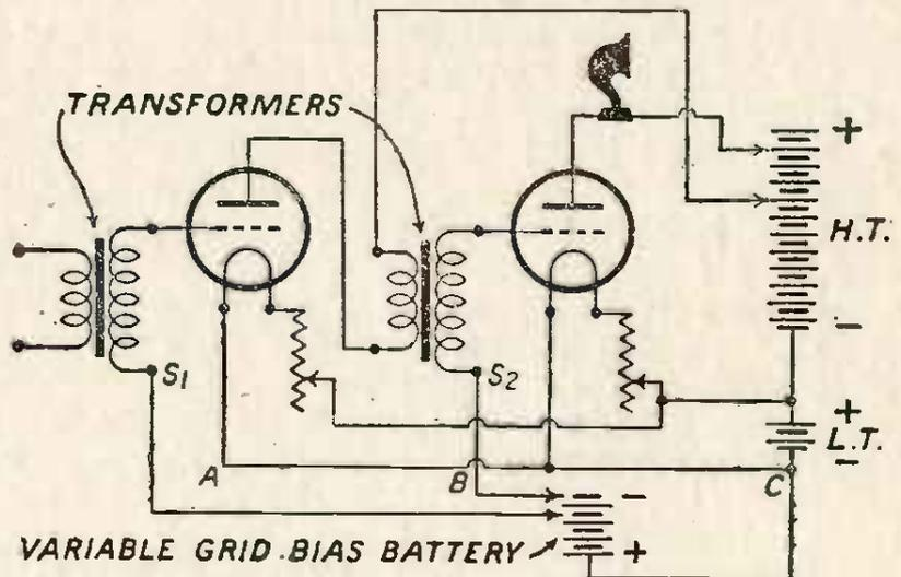
The correct way to apply “negative grid bias” to low frequency valves.
