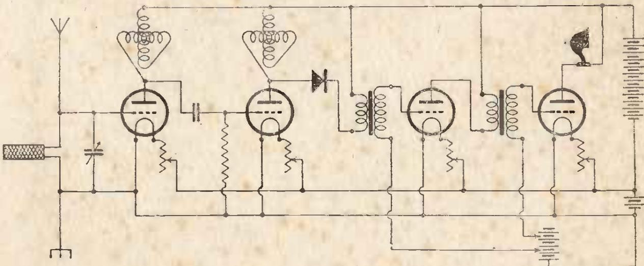
20. This combined crystal and four-valve receiver is capable of operating a loud speaker at a distance of a couple of hundred miles or more from a broadcast station. It is comparatively simple to operate, the two high-frequency valves being tuned by variometers.
