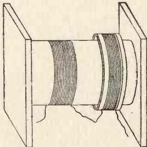
FIG. 9.—Illustrating the principle of the sliding variometer.
