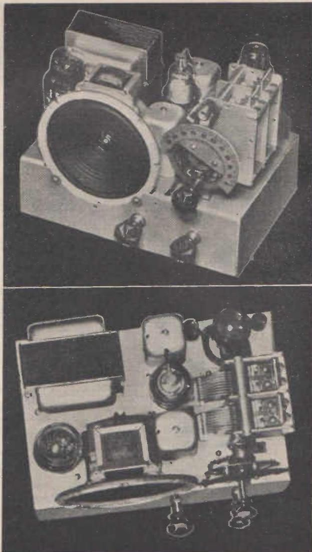
To align the receiver, set the trimmers on top of the gang about halfway out, and tune in a station near the middle of the band—one that requires a fair amount of reaction to bring it up to quiet room strength is best. The trimmer on the first section of the gang can then be adjusted for best results.
