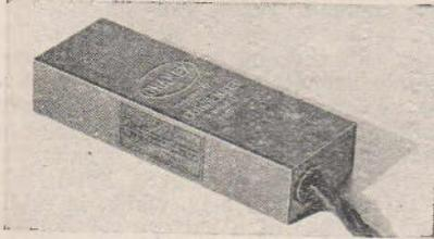
Chanex type H 11 metal-cased condenser suppressor unit, capacity .5 mfd. + .5 mfd., designed for connection to large D.C. motors, generators, and at power points, etc. Fuses are incorporated.
