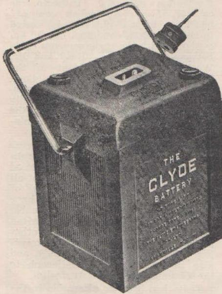
two-pin, non-reversible socket. Connection to the positive and negative terminals is made by means of lead-coated brass straps, moulded into the cover, with lugs at each end to fit over the battery terminals.
