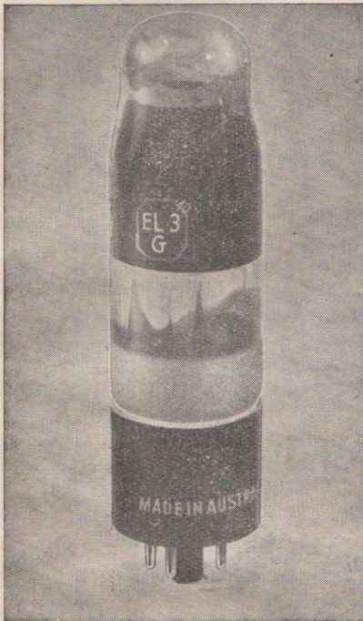
The new Philips EL3G high slope pentode, reviewed on this page.
