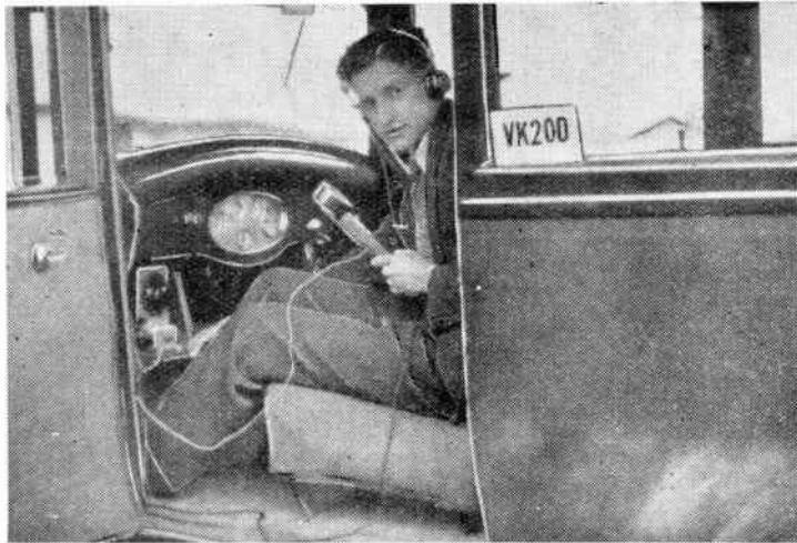
Equipment used by VK2OD during mobile tests on five metres in 1934-5. The transceiver is mounted under the dash-board at the left. This photo was taken at Bathurst during tests with VK2NS over the 1935 Easter holidays.
